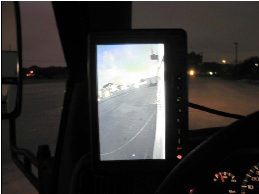
Figure 5-27. Image from camera-based system during nighttime
