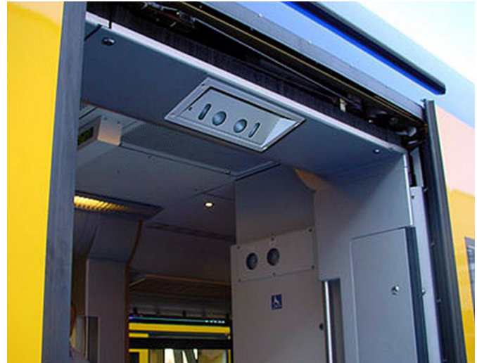
This image shows one type of Automated Passenger Counter integrated unobtrusively into the top of a bus doorway.
