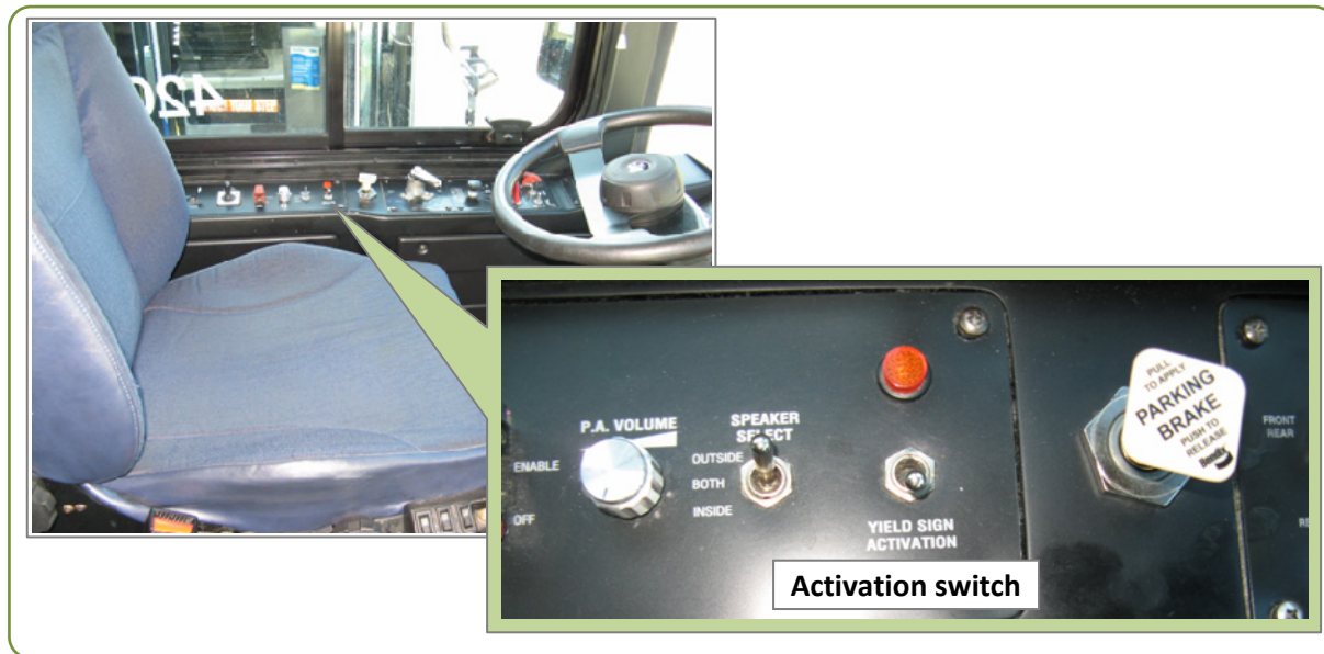
Figure 7: YTB-LED sign activation switch.
