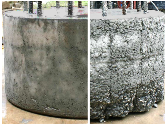
Effect of slurry viscosity on concrete flow: left – 60 sec/qt; right – 90 sec/qt.
