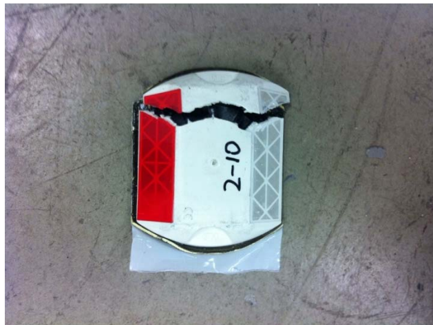
Figure 9-17 Typical 3M 290 Failure in the RRLFT
