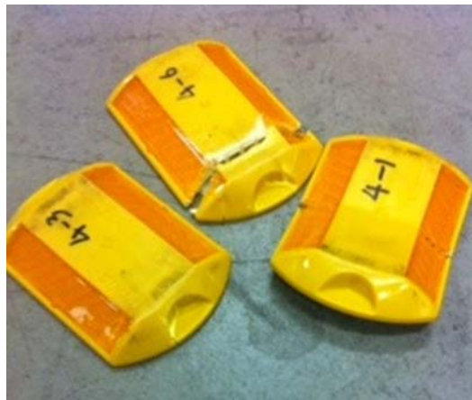
Figure 9-19 Typical Ennis C80 Failure in the RRLFT
