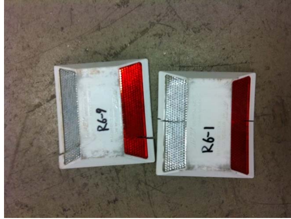
Figure 9-21 Typical Apex 921AR Failure in the RRLFT
