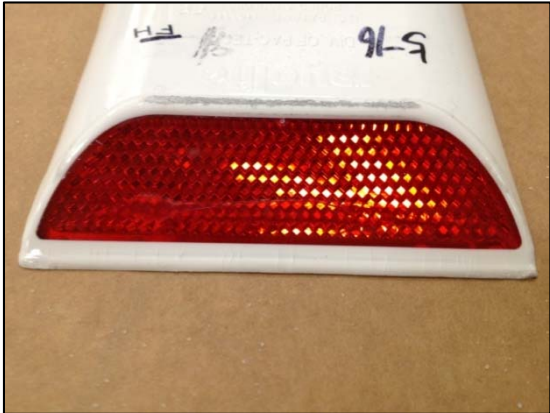
Figure 9-2 Edge Breakage of Marker 5-16 in Compressive Test
