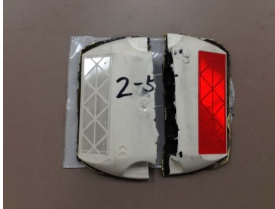
Figure 9-10 Center Breakage of Marker 2-5 in 1/3 Flexural Test
