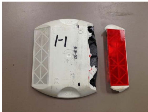
Figure 9-9 Edge Breakage of Marker 1-1 in 1/3 Flexural Test
