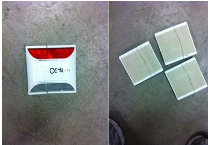
Figure 9-25 Typical Rayolite RS Failure in the OLFT
