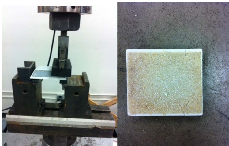
Figure 9-26 Typical Apex 921AR Failure in the OLFT
