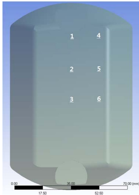
Figure 8-19 RRPM Impact Location ID for Pendulum Test
