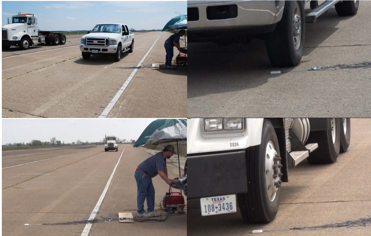
Figure 7-4 Testing Scenes of Pickup and Tractor Running Over Marker Specimens
