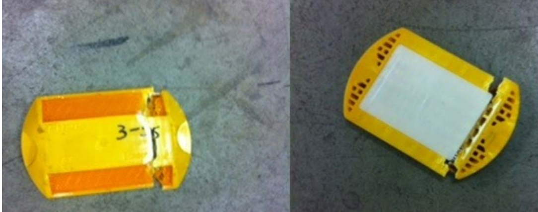
Figure 9-18 Typical Ennis 980 Failure in the RRLFT
