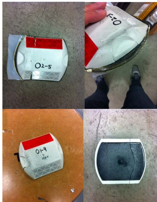
Figure 9-23 Two Types of 3M 290 Failure in the OLFT
