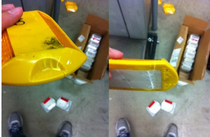
Figure 9-24 Typical Ennis 980 and Ennis C80 Failure in the OLFT
