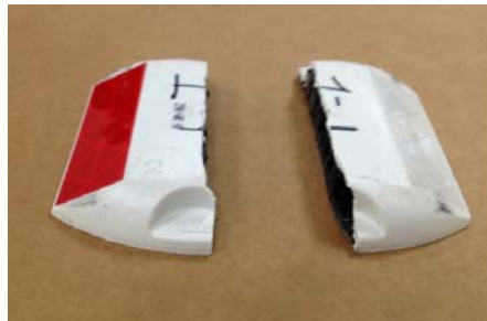
Figure 9-5 Typical Center Breakage in Flexural Test
