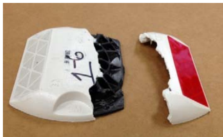
Figure 9-6 Typical Edge Breakage in Flexural Test
