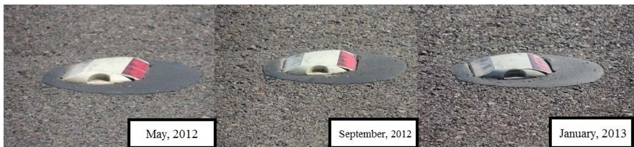
Figure 4-11 One 3M 290 Marker at Site 15 (on Causeway Blvd & S 50 th St.)
