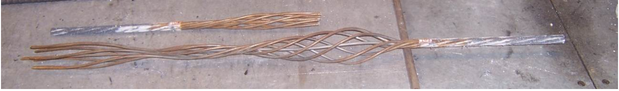
Figure 36 Typical Strand after Tensile Testing
