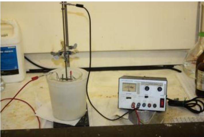
Figure 39b Hydrogen Charging Setup with Variable Power Source
