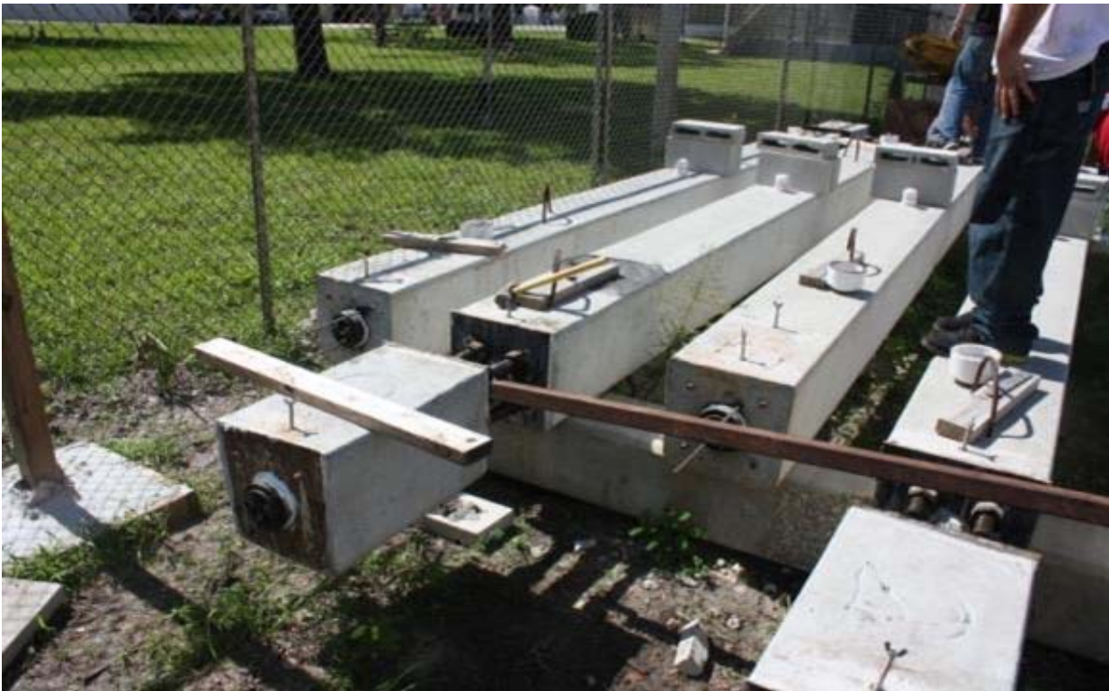
Figure 32 Stressing Strand at USF
