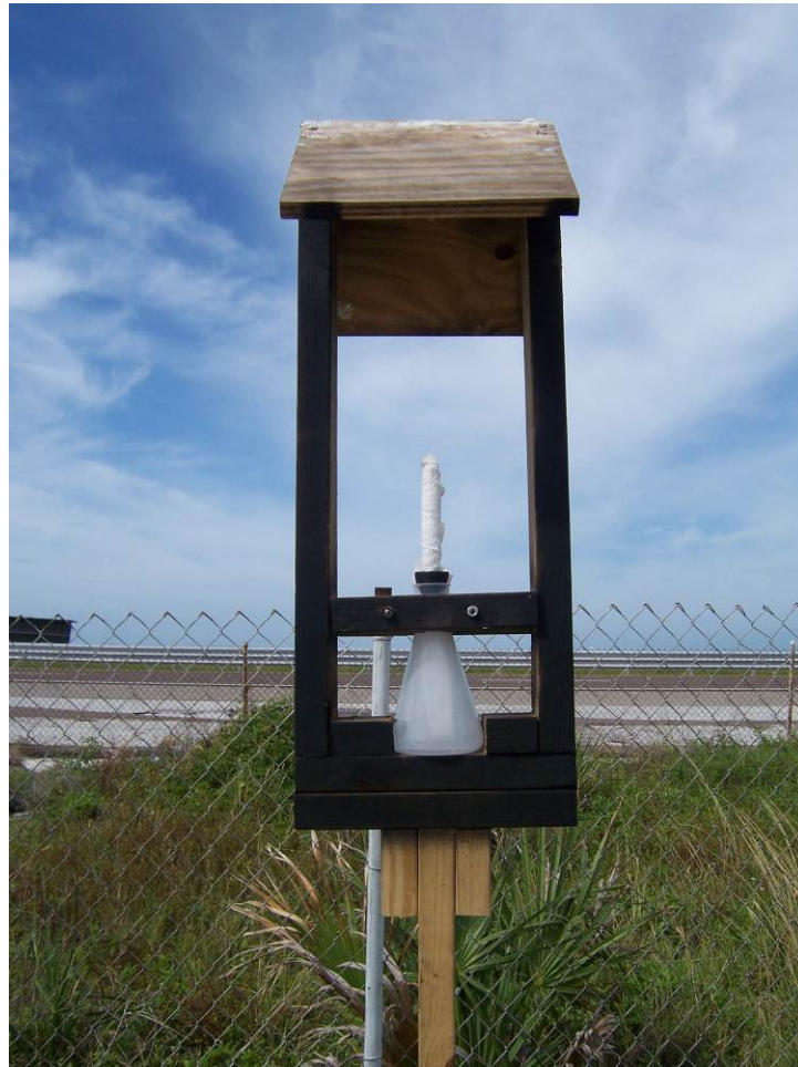
Figure 26 Wet Candle Setup for Determining Atmospheric Cl - Deposition Rate at SSK Facility
