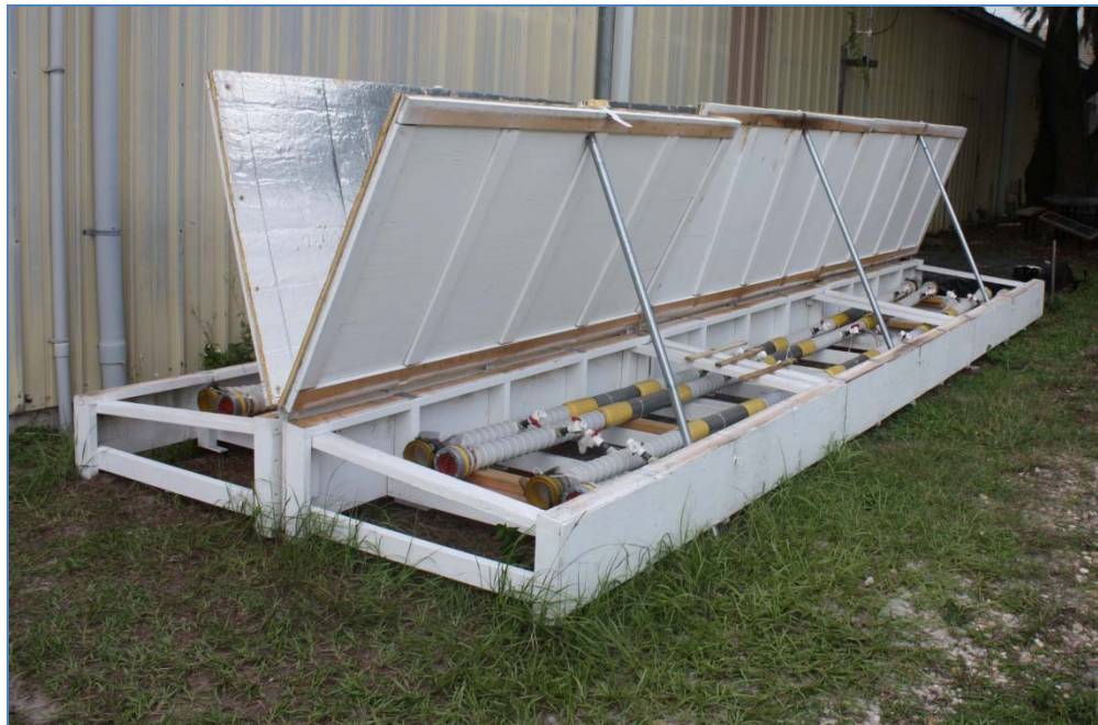
Figure C1 USF Duct Facility in the Open Position
