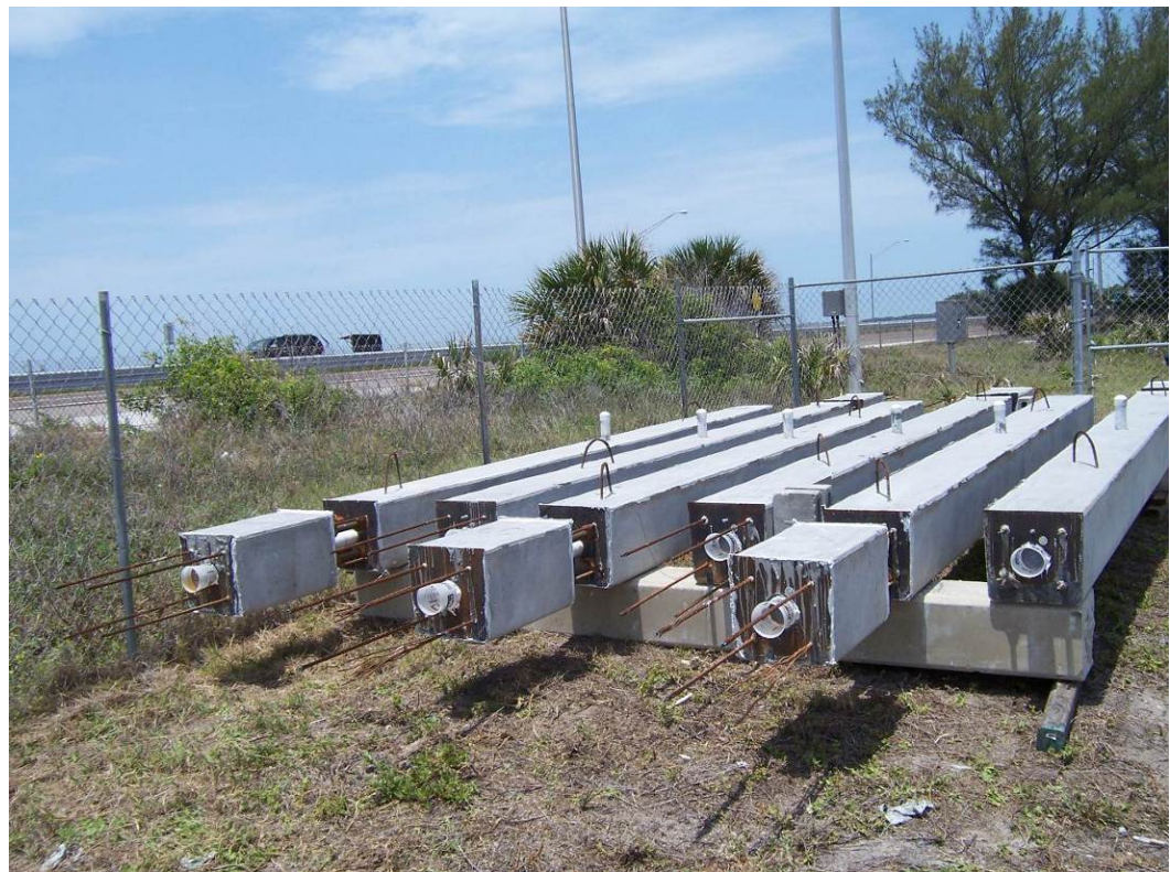
Figure 11 De-tensioning Pile System at Marine Location (SSK)
