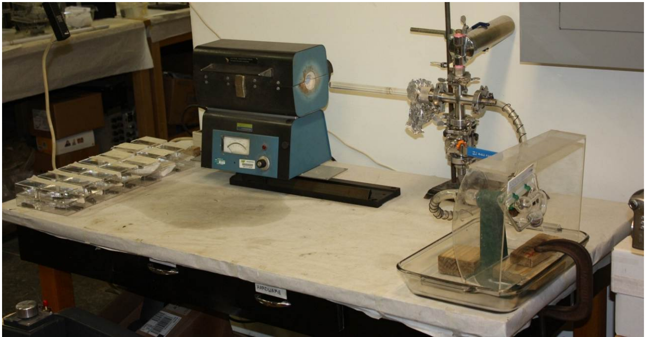
Figure 37b Hydrogen Concentration Measurement Setup
