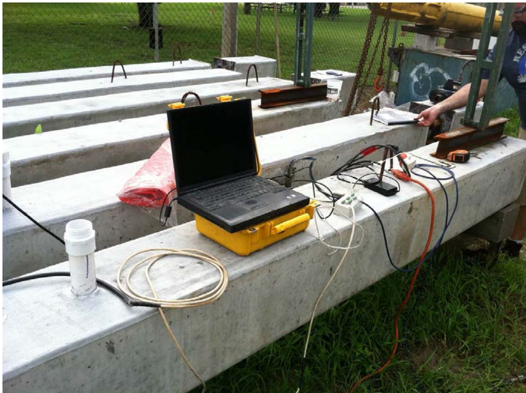
Figure 24 On-Site Testing Evaluation Setup for Stressing Operation Test
