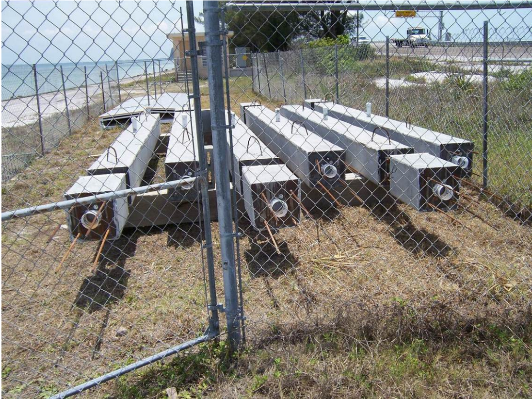
Figure 12 De-tensioning Pile System at Marine Location (SSK)
