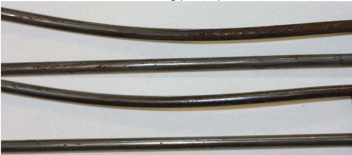
Figure 62 Specimen 106a 4 Week Salted and Wet Exposed (Top) and after Cleaning (Bottom)
