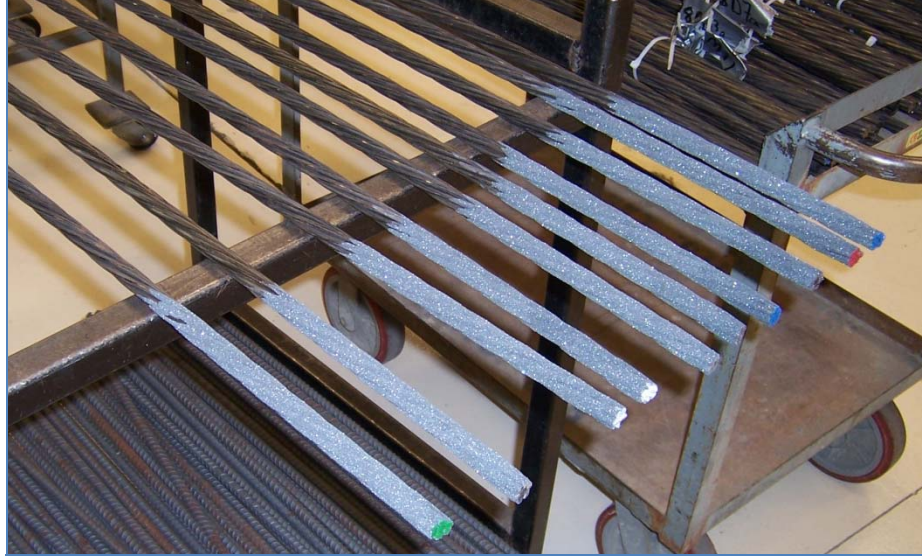
Figure C13 Sample Strands' Ends Coated in Grit Material Awaiting Tensile Testing
