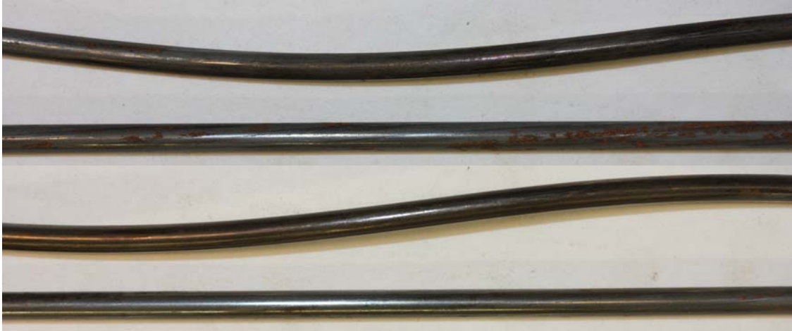
Figure 61 Specimen 97a 4 Week not Salted but Wet Exposed (Top) and after Cleaning (Bottom)
