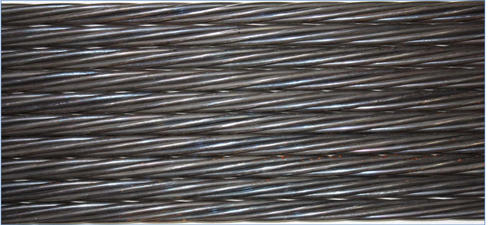
Figure C6 Typical As Received Condition of Strands Prior to Exposure
