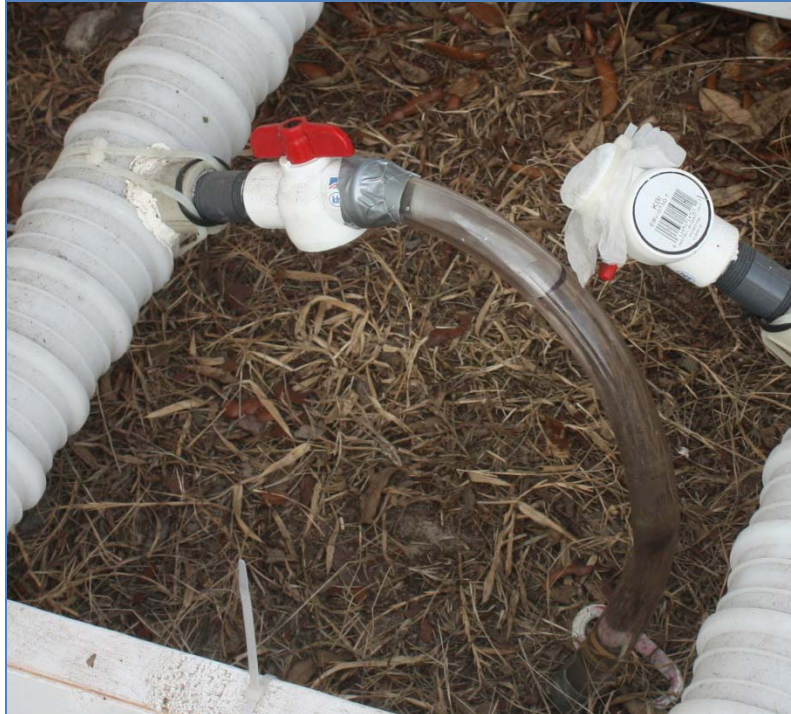
Figure C4 Water Reservoir Attached via Vent Port (left) and Closed Vent Port Covered with Bug Shield (Right)
