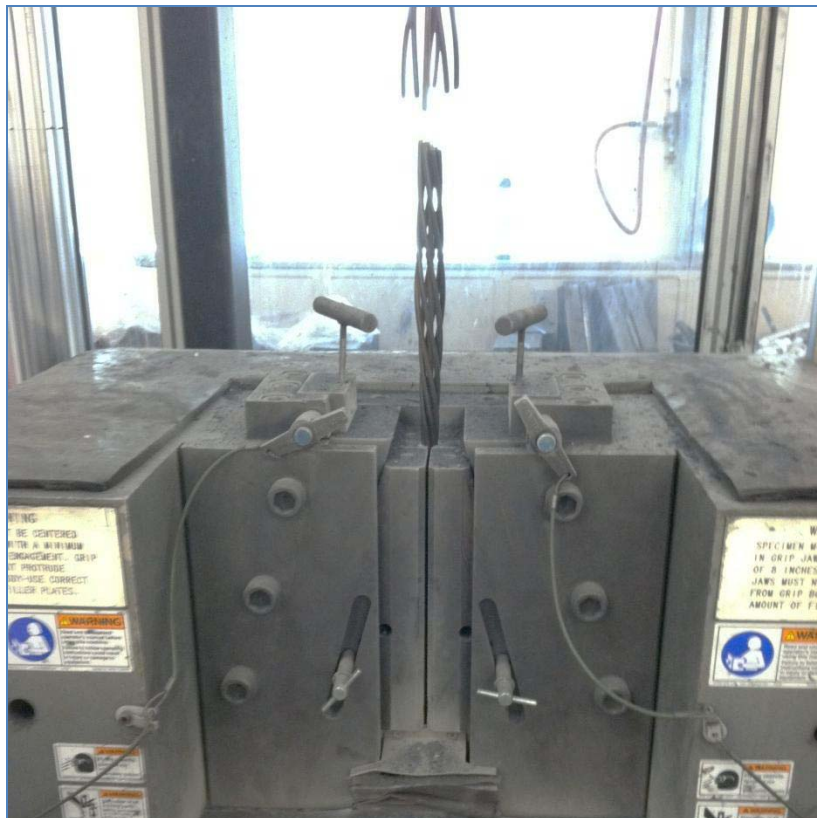
Figure C14 Sample Strand Break and Fully Engaged Grip
