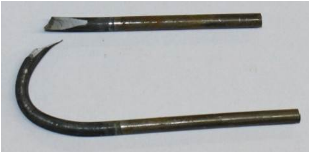
Figure 57 U-Bend Specimen Failed Due to Delayed Failure Hydrogen Embrittlement
