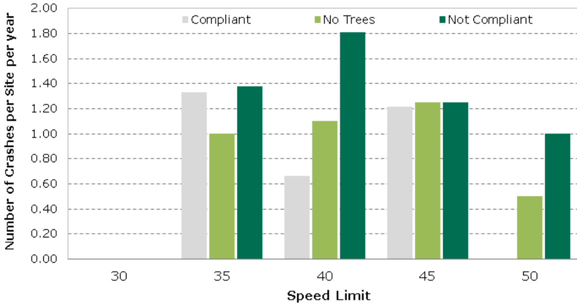
Figure 6-11. Comparison of Average Number of Crashes per Year per Intersection for Three Groups from 30 mph to 50 mph at Major Streets
