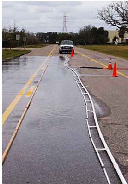
A truck towing the locked wheel skid tester prepares for a run through a water film on a prepared course.
