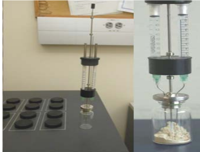
Figure 3.6: Ampoule and Typical Ampoule-Glass Container Configuration
