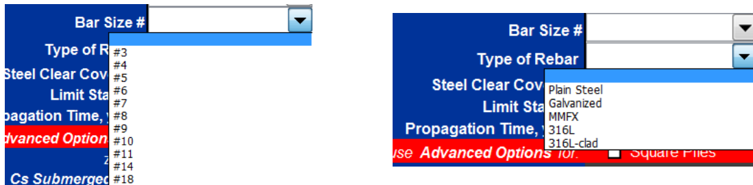
Figure A 8 Bar size options and type of rebars incorporated in the program
