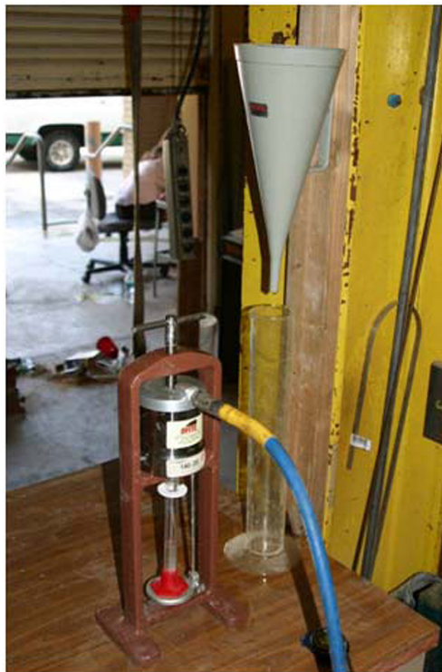
The API filter press apparatus (lower left) and the Marsh cone viscometer (upper right) used in this study.
