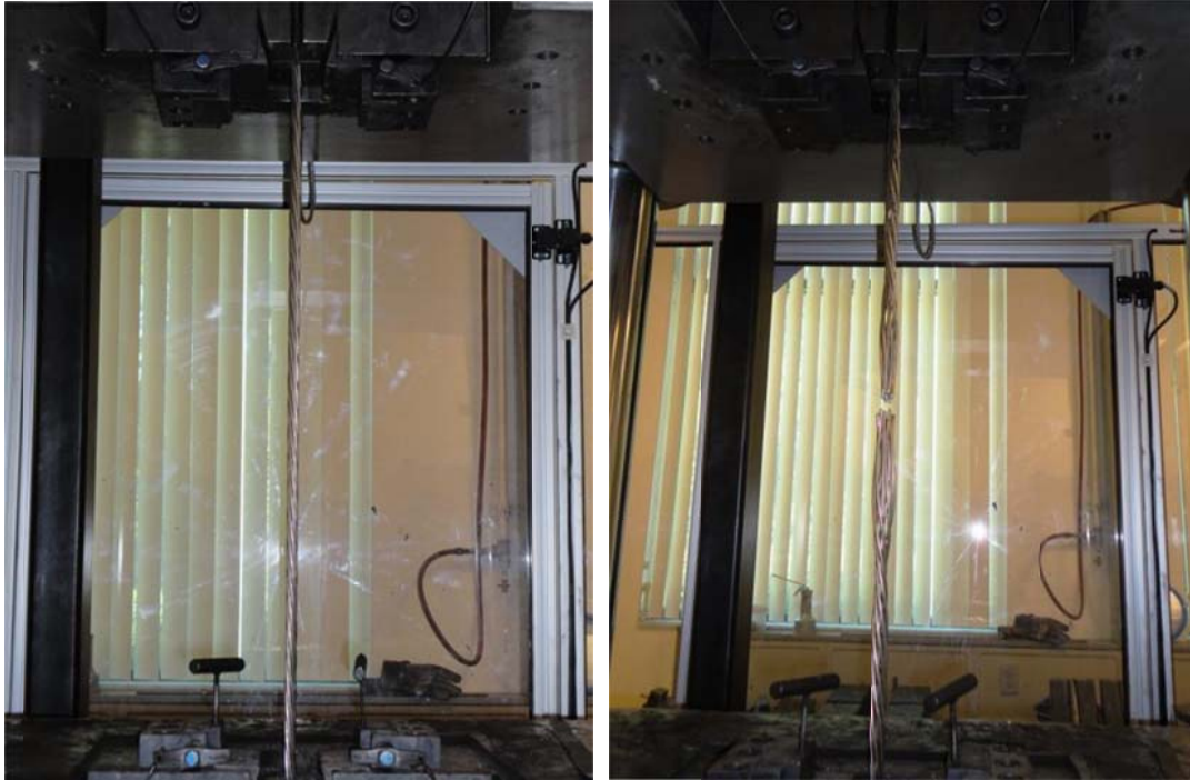
Figure 4.11 Testing after extensometer removal (left); after failure (right).
