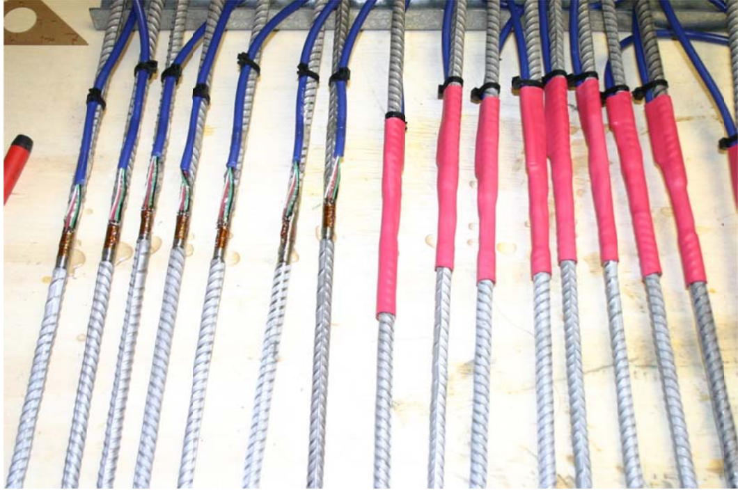
Figure 5.3 Stainless steel sister bar gages prepared for embedment.
