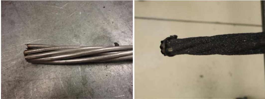
Figure 4.7 Unraveled XM-29 strand (left) tie wire-restrained XM-29 with silicon grit.
