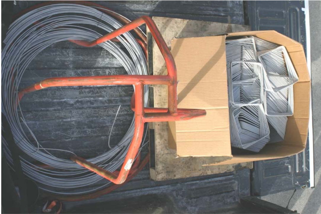
Figure 5.2 80 ksi Grade 304 stainless steel wire used for spirals (as-received, left) and fabricated into spirals (right).
