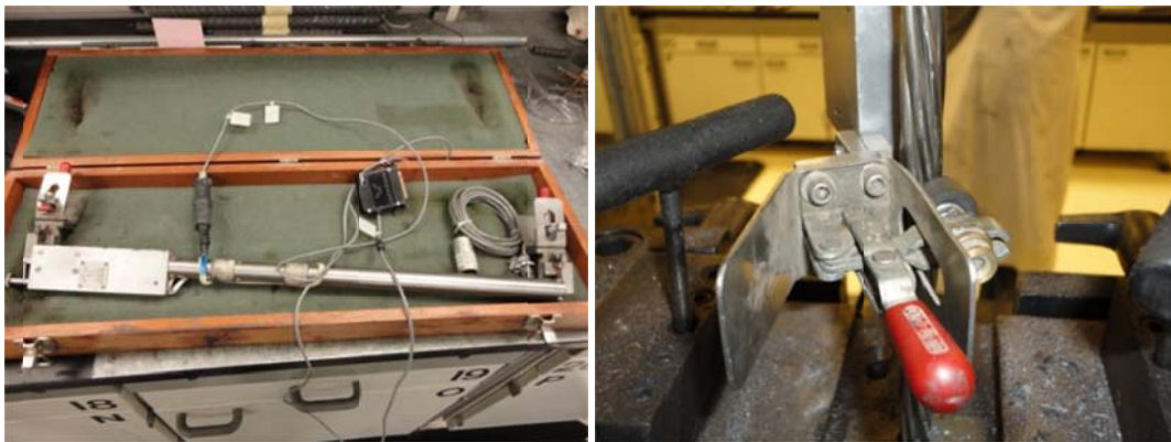
Figure 4.10 24in extensometer (left); close-up of extensometer strand clamp (right)
