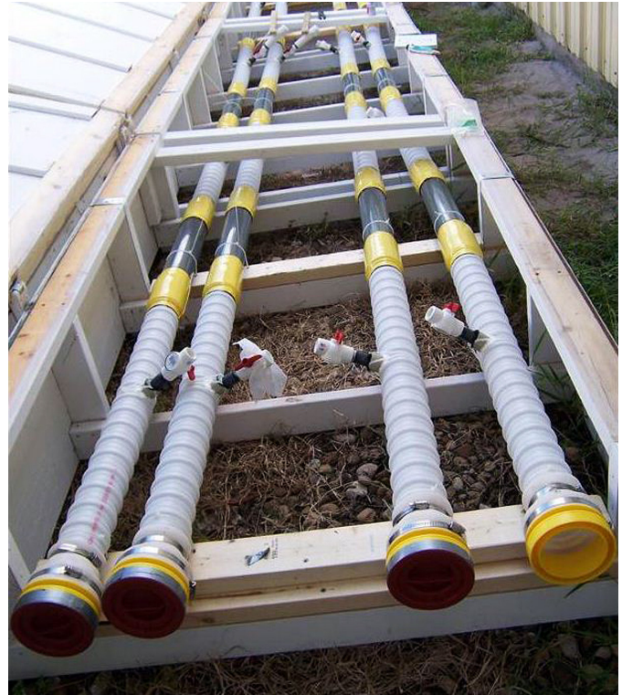
The experimental set-up for this project tested tensioning strands in wet and dry conditions at both inland and seaside locations.
