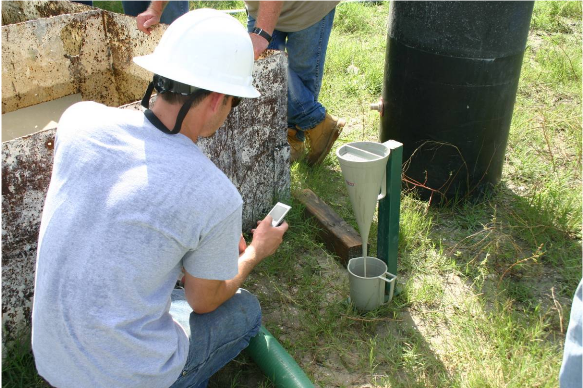
Figure 4.26. Viscosity testing directly after mixing with mulit-gang educator system.
