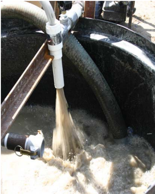
Figure 2.14. Vacuum-feed eductor used to mix bentonite slurry in previous study (Mullins, 2005).
