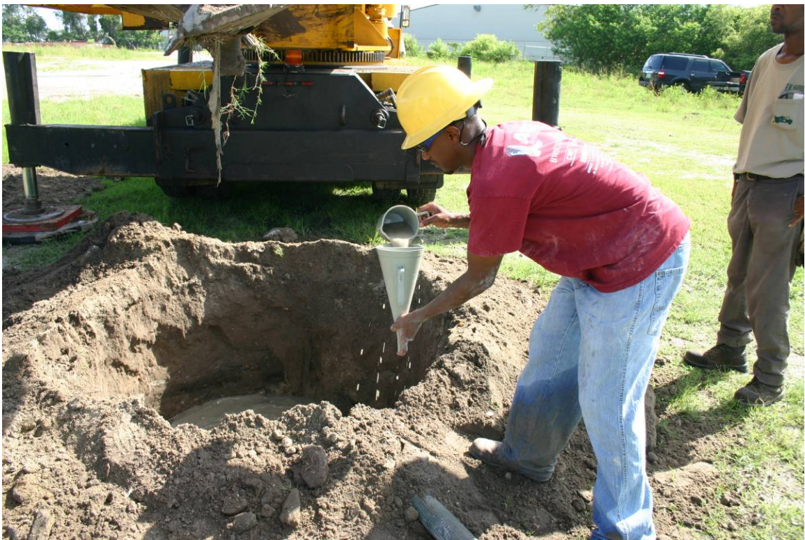
Figure 4.27. Viscosity testing at excavation.
