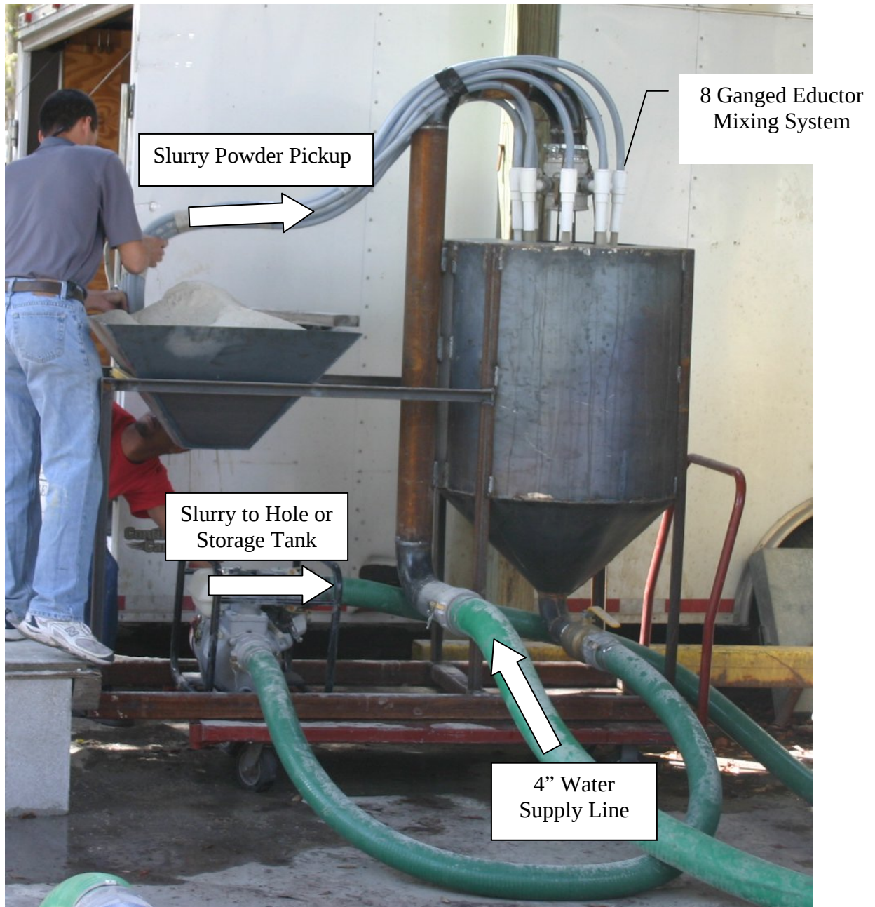
Figure 4.15. Multi-gang eductor system.
