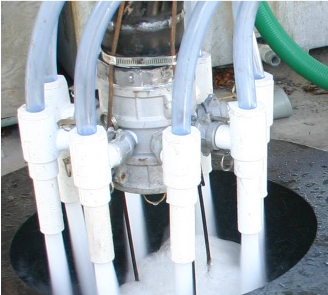
Figure 5.2. Eductors equipped with quick-connect fittings for easy reconfiguration (shown 220 GPM total ; 27.5 GPM per eductor).
