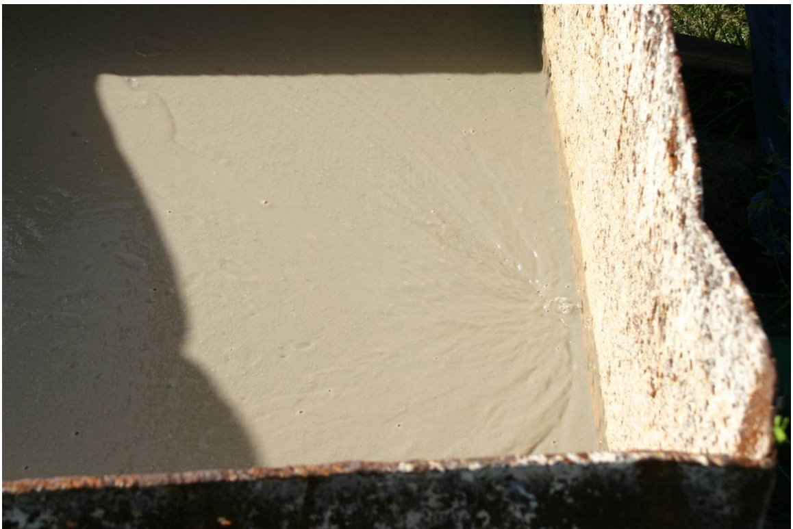
Figure 4.25. Initial slurry mixture with 8 eductors.
