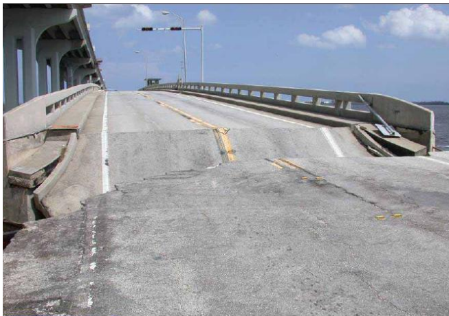
Figure 2.19. Damage to bridge approach slabs in Florida during 2004 hurricane season (Pavlov 2005)
