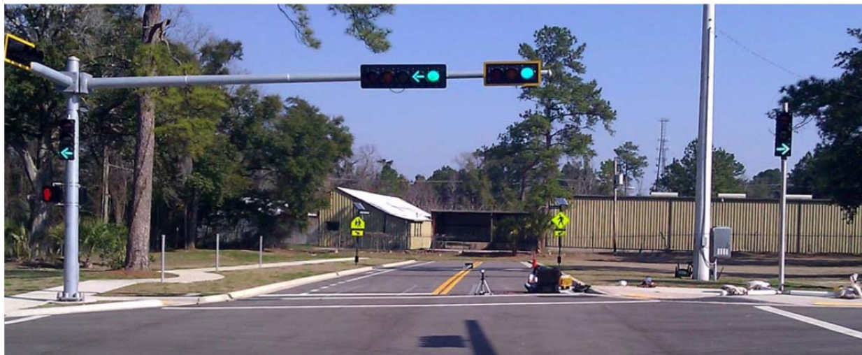
Figure 29. The test intersection shown with both supplemental signals enabled. The supplemental signal on the right is supported by an aluminum tripod
