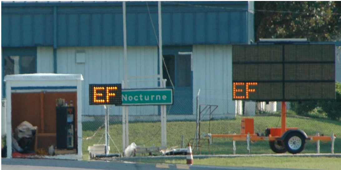
Figure 64. Photograph showing the setup of the field. 16.8" sign on the left, 18" sign on the right.
