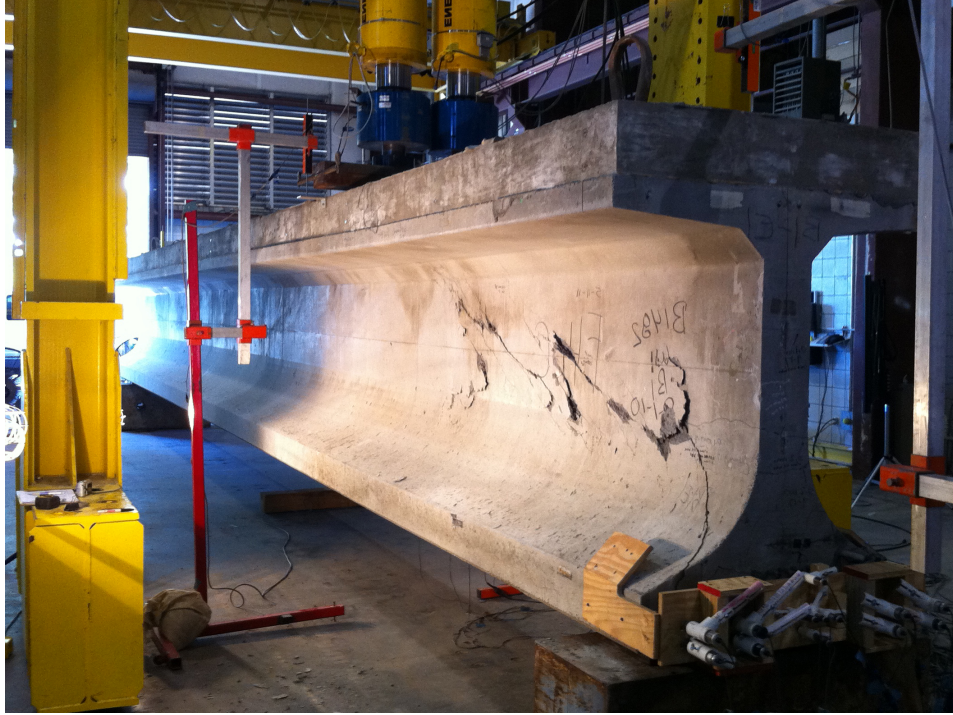
Figure 1.2: Concrete failure in structural testing
