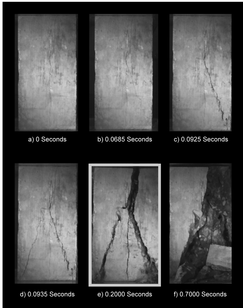
Figure 4.15: Column failure under regular friction
