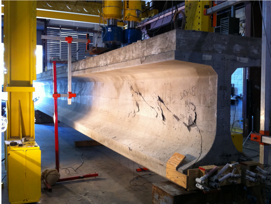
Figure 1.2: Concrete failure in structural testing
