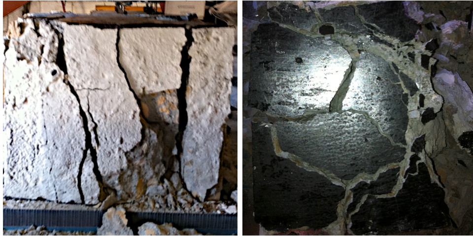
(a) Vertical cracks (b) Cracked top surface Figure 4.13: Fracture pattern of test group cubes (reduced friction)
