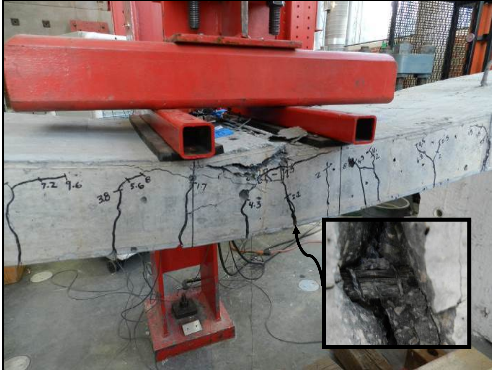
Figure 5.224: Specimen BR1, crushing of concrete in compression
