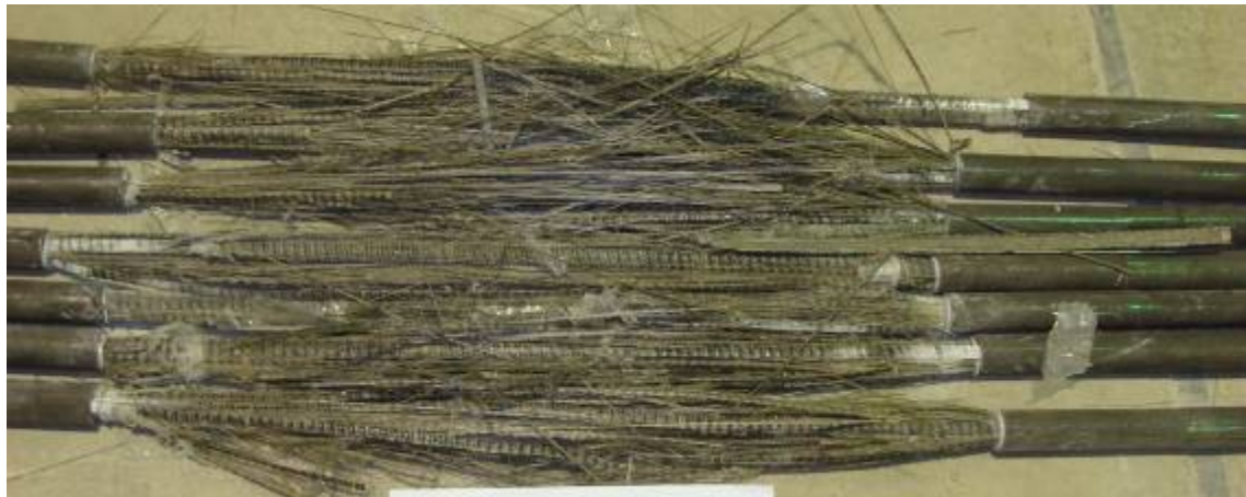
Figure 5.164: Mode of failure of BASA BFRP bars of 16 mm in diameter
