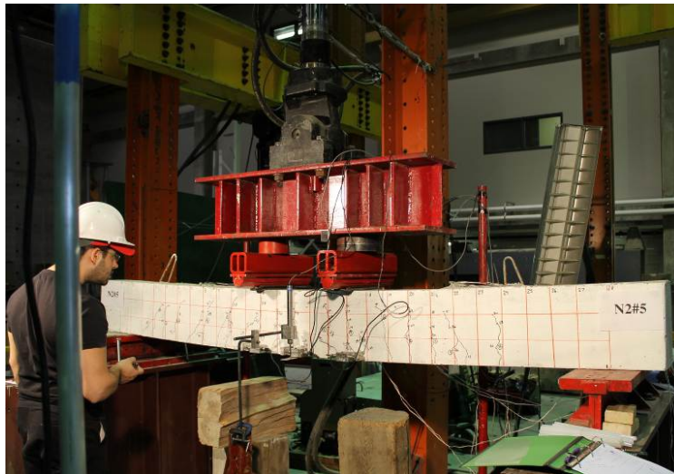
Figure 5.207: Test setup during a beam test
