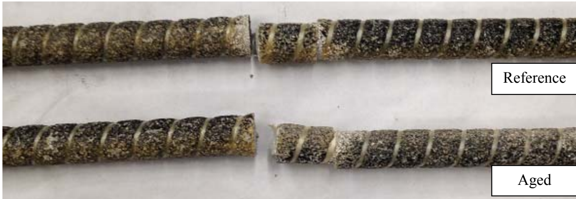
Figure 5.165: Reference and aged BFRP bars No.5 after shear tests
