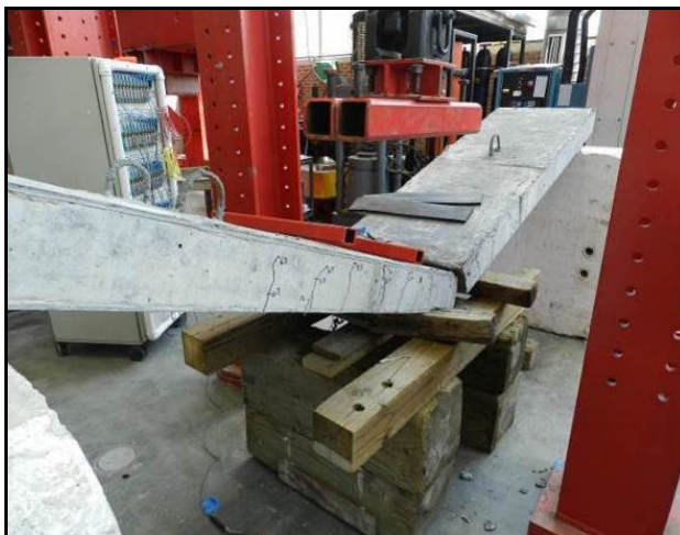
Figure 5.222: Specimen UR1 following rupture of the BFRP Bars
