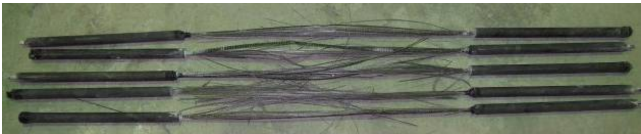
Figure 5.159: Mode of failure of BASA BFRP bars of size 8 mm (code 43 and 51)
