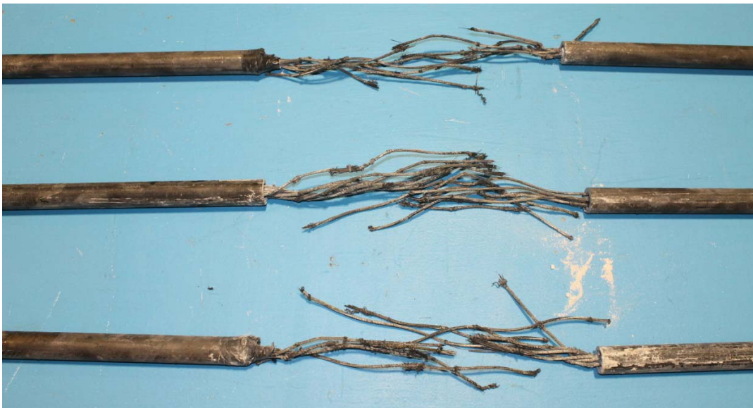
Figure 4.30: Mode of failure of conditioned specimens at 22° C with 3,000 hr
