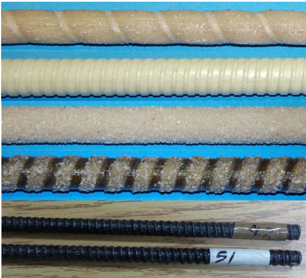
Figure 2.3: Different surfaces types of FRP bars
