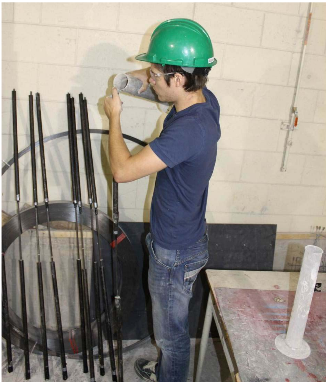
Figure 5.17: Filling the anchorage with cement grout
