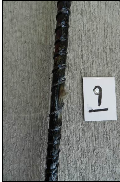
Figure 5.155: Specimen J9, failure at middle
