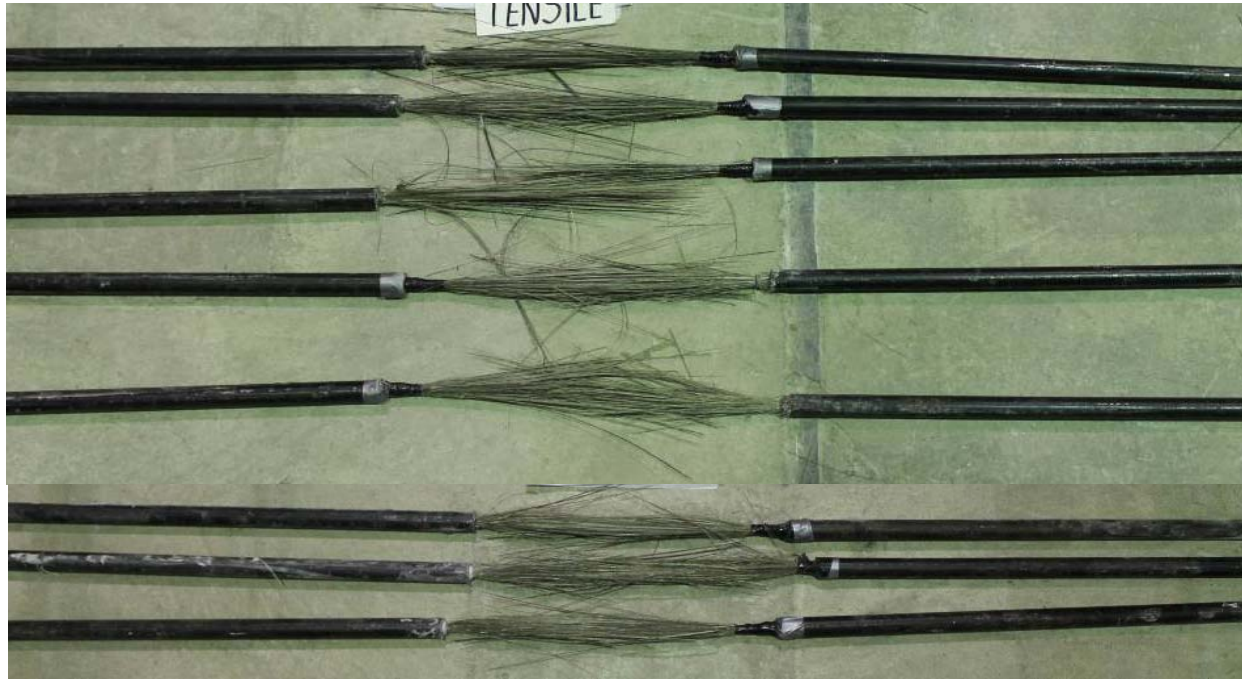
Figure 5.157: Mode of failure of prestressing BFRP bars of 7-mm in diameter
