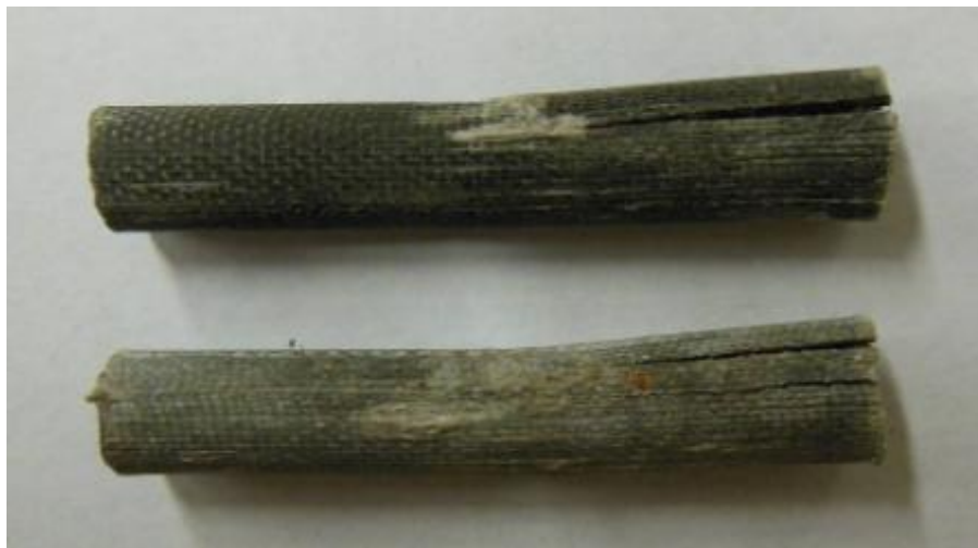
Figure 5.168: Interlaminar shear failure prestressing BFRP bars 7-mm
