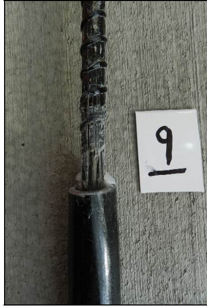
Figure 5.156: Specimen J2, failure near grip
