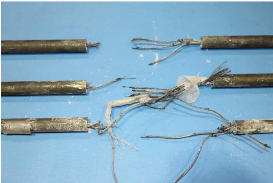
Figure 4.26: Mode of failure of conditioned specimens at 40°C after 1,000 hr
