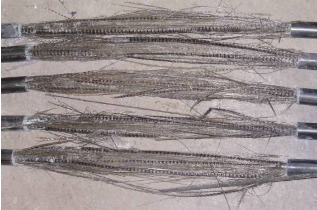
Figure 5.162: A typical mode of failure of BASA BFRP bars 12 mm (code 43) (Reference)
