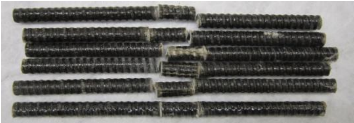
Figure 5.172: A typical shear failure of the tested unconditioned specimens
