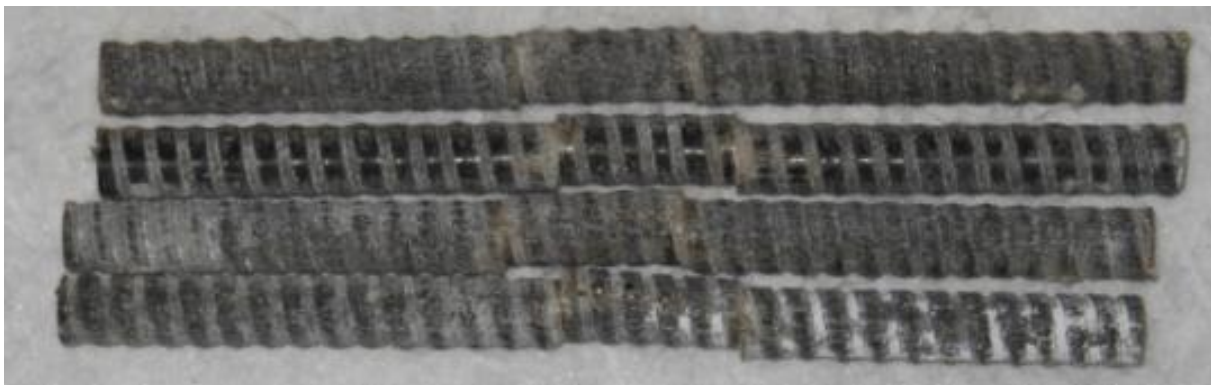
Figure 5.173: A typical mode of shear failure of the tested conditioned specimens
