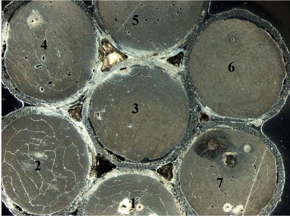
Figure 4.13: General view of carbon Rope cross-section by optical microscopy
