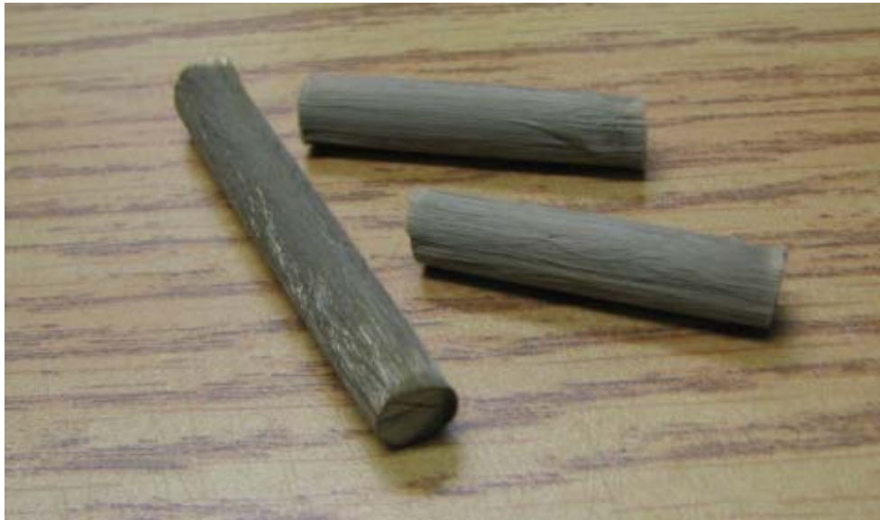
Figure 5.30: Prestressing BFRP 7-mm in diameter after pyrolysis
