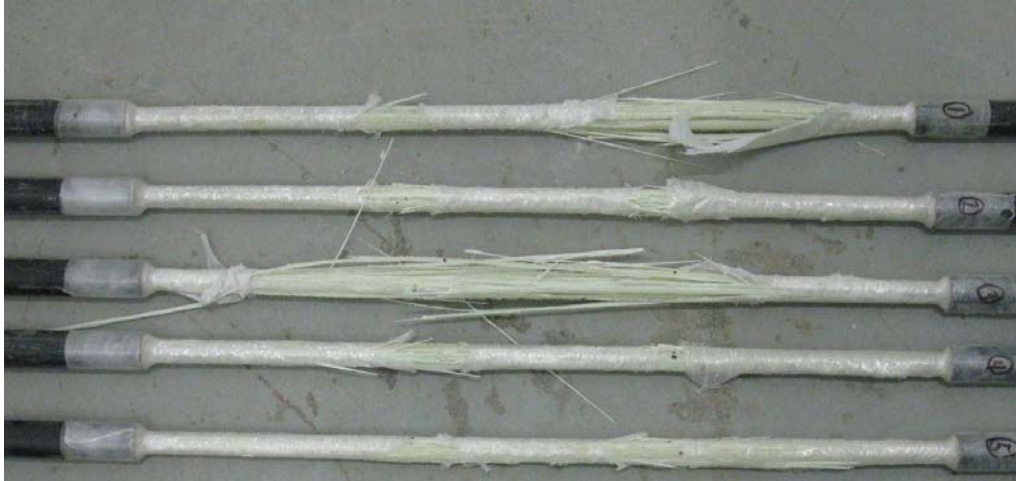
Figure 3.17: Typical mode of failure of the tested GFRP bars
