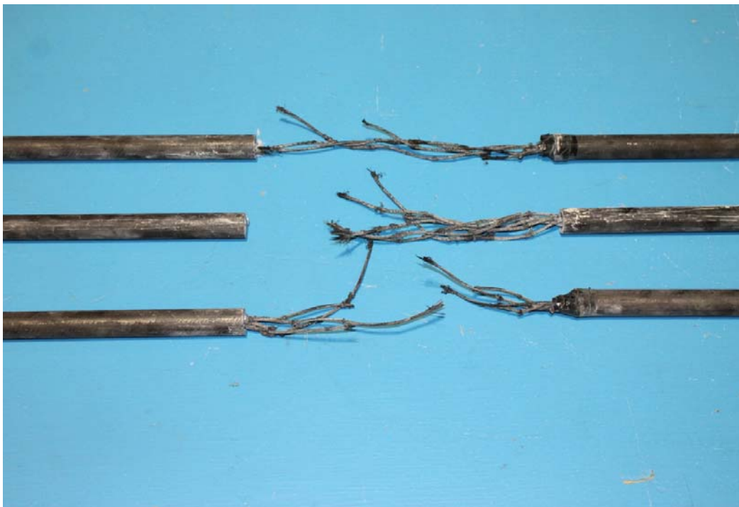
Figure 4.33: Mode of failure of conditioned specimens at 60°C with 3,000 hr
