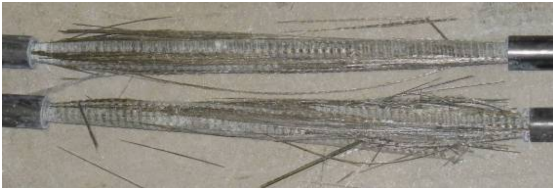
Figure 5.163: A typical mode of failure of BASA BFRP bars 12 mm (code 43) (Conditioned for 2 months (1440 hrs.))
