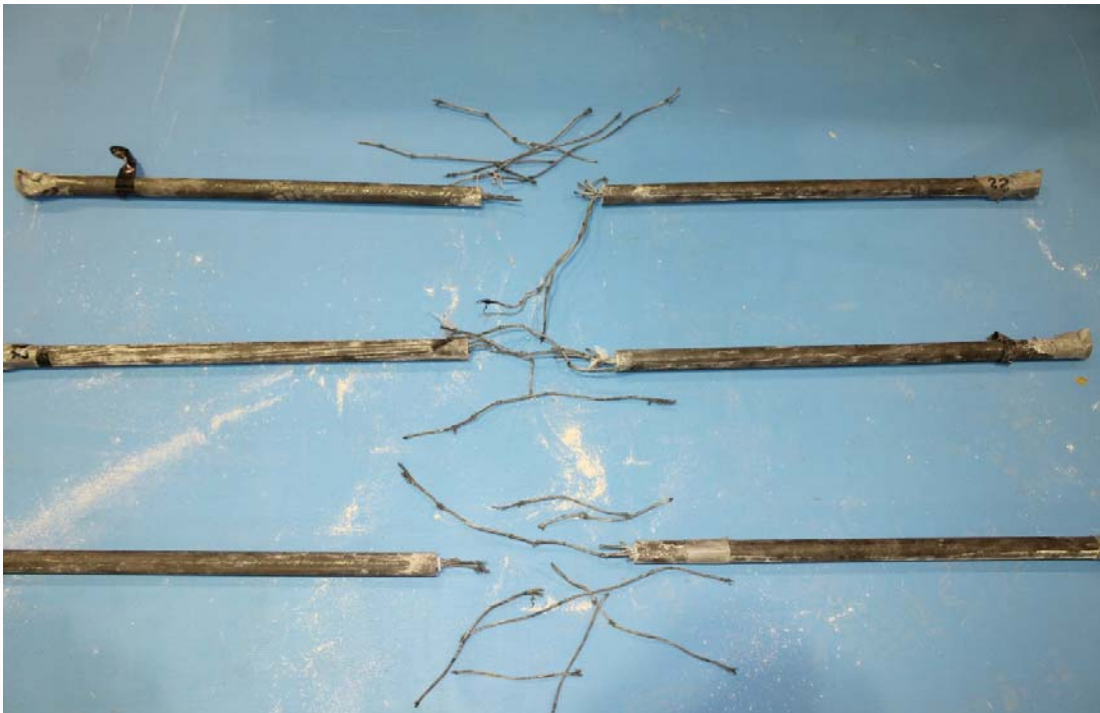
Figure 4.28: Mode of failure of conditioned specimens at 60°C with 1,000 hr
