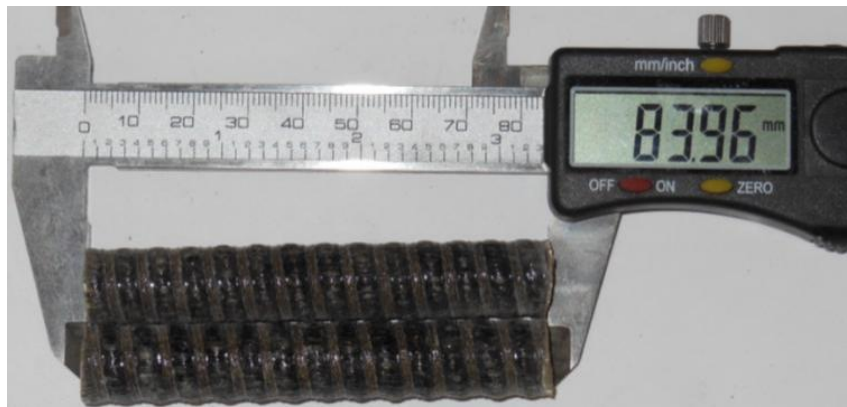
Figure 5.180: BASA BFRP bars of sizes 12 mm (code 43)
