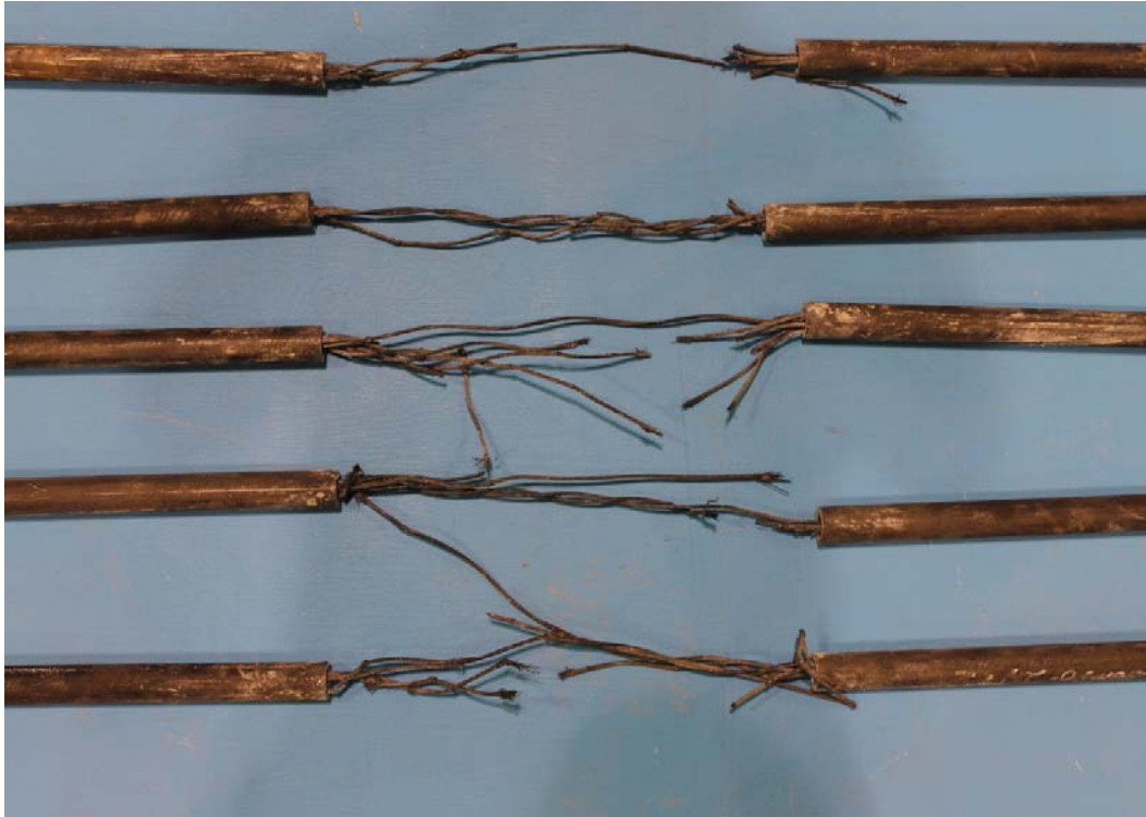
Figure 4.29: Mode of failure of reference specimens
