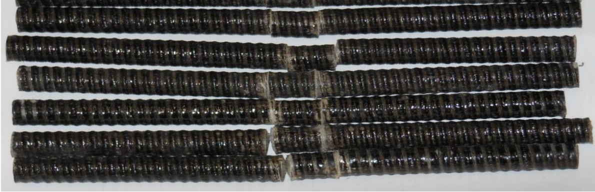
Figure 5.181: Transverse shear failure of the tested BASA BFRP bars
