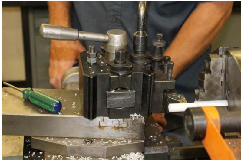
Figure 5.12: Fabrication of plastic rings
