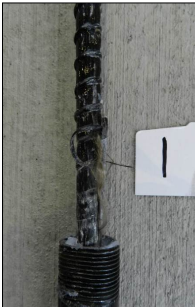
Figure 5.152: Specimen J1, failure near grip
