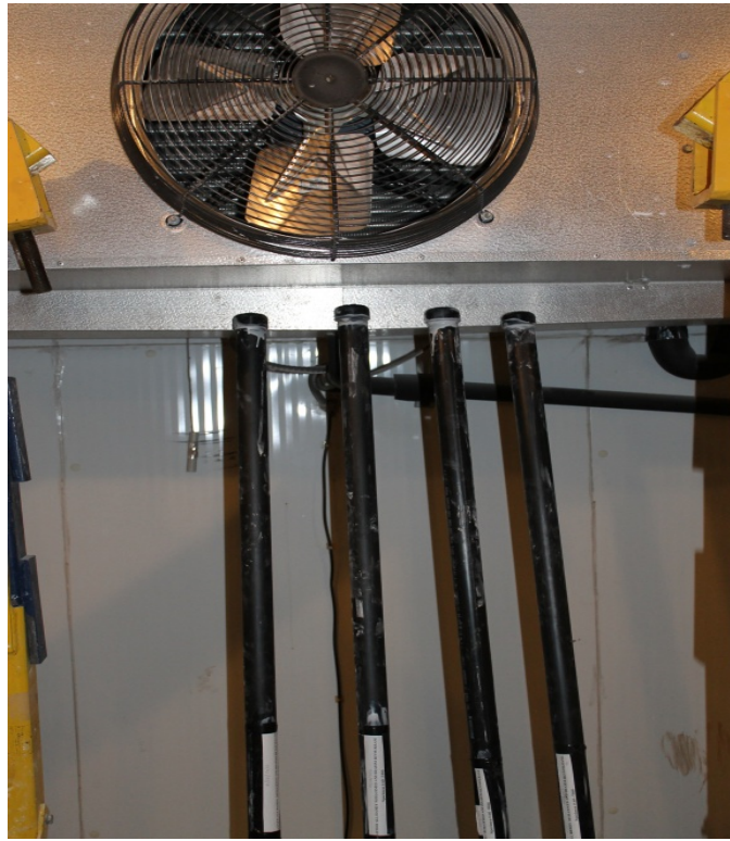
(a) Specimens inside the environmental chamber of 60 °C
