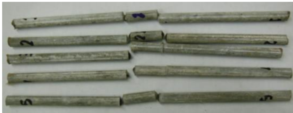
Figure 5.167: Transverse shear failure of prestressing BFRP bars 7-mm
