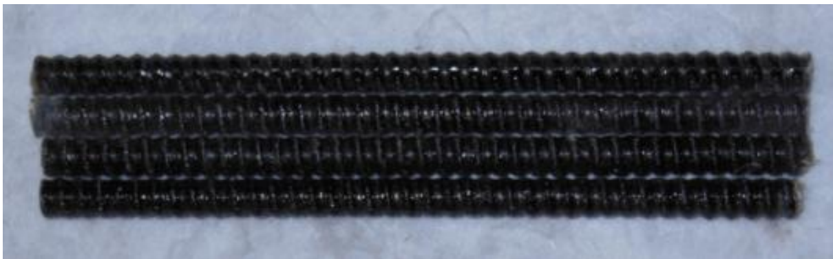
Figure 5.170: BASA BFRP bars of sizes 8 mm, BASA code 43 and 51 for transverse shear tests (Before conditioning)
