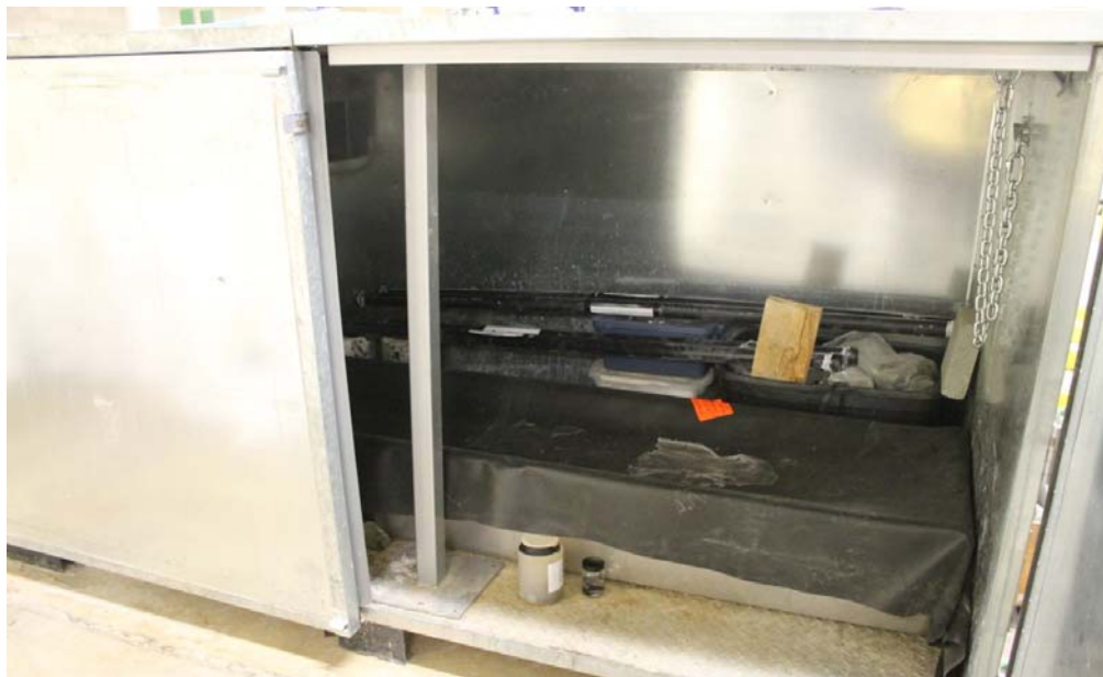
(b) Specimens inside the environmental chamber of 50 °C
