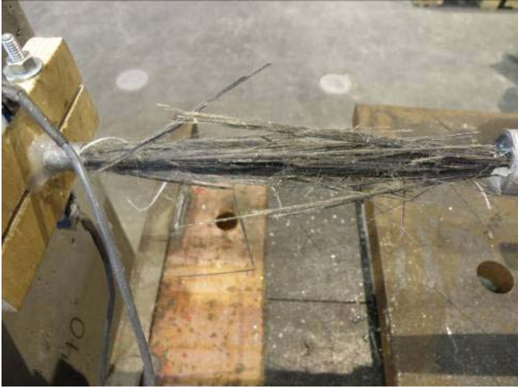
Figure 5.203: Observed failure of type A BFRP bars
