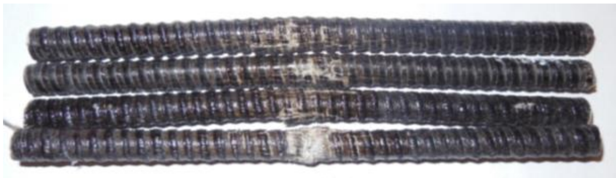
Figure 5.178: A typical mode of failure of the tested specimens (Compression failure)
