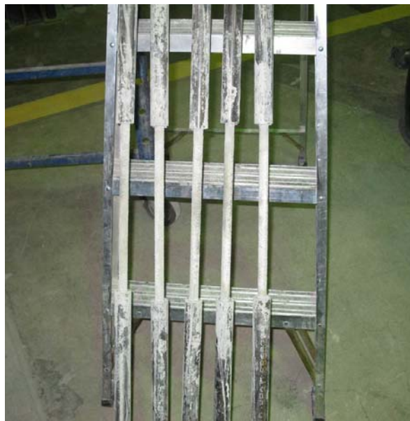
Figure 3.3: GFRP bars of No.5 (Grade II) after drying
