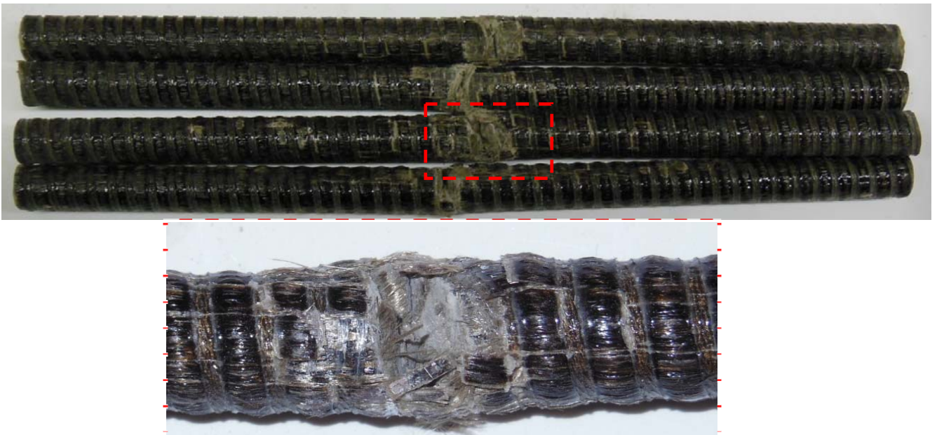
Figure 5.183: Typical flexure mode of failure of the tested BASA BFRP bars (compression failure)
