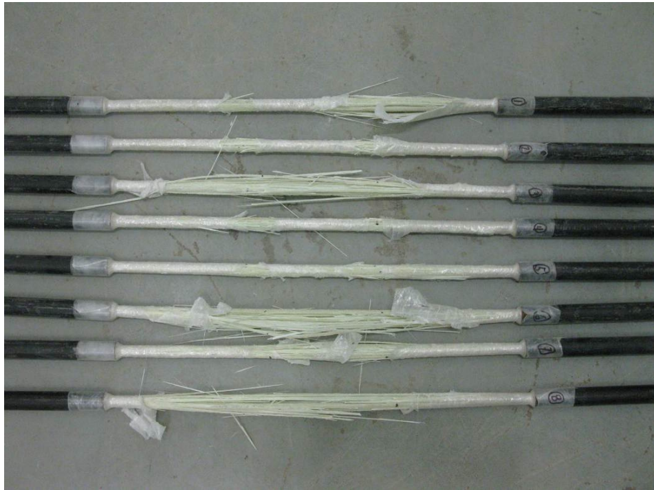
Figure 3.14: Mode of failure of GFRP bars No. 4 (Grade II)
