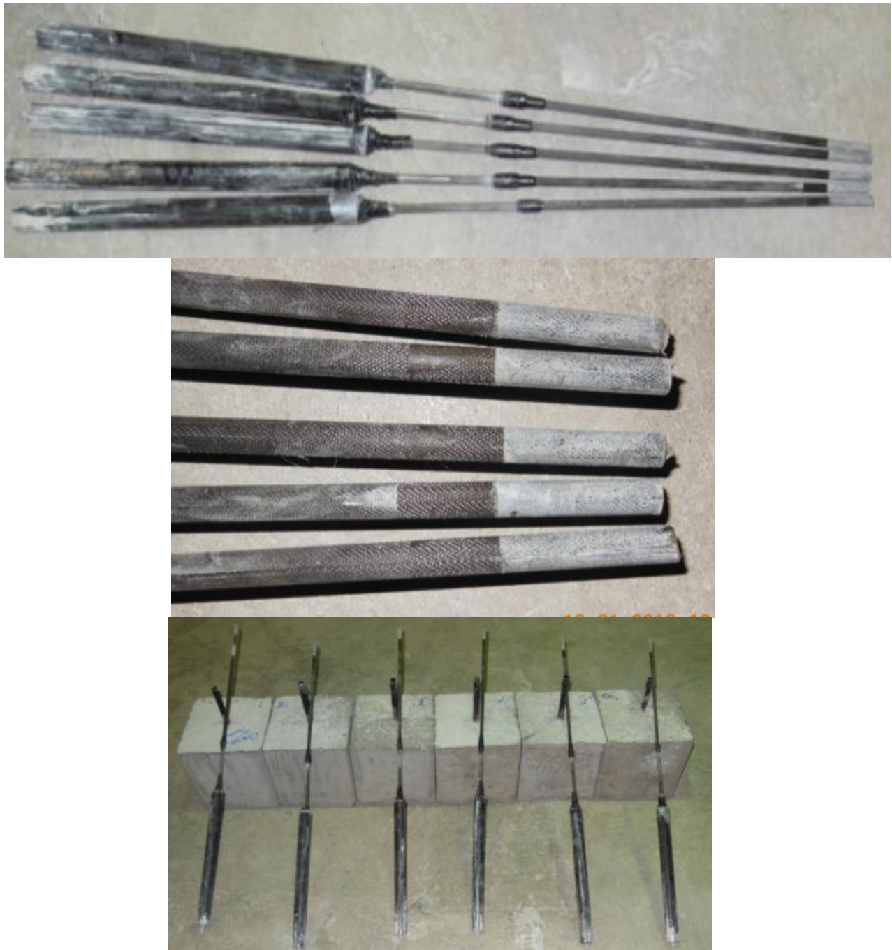
Figure 5.184: Mode of failure of the pullout specimens of prestressing BFRP bars 7-mm in diameter
