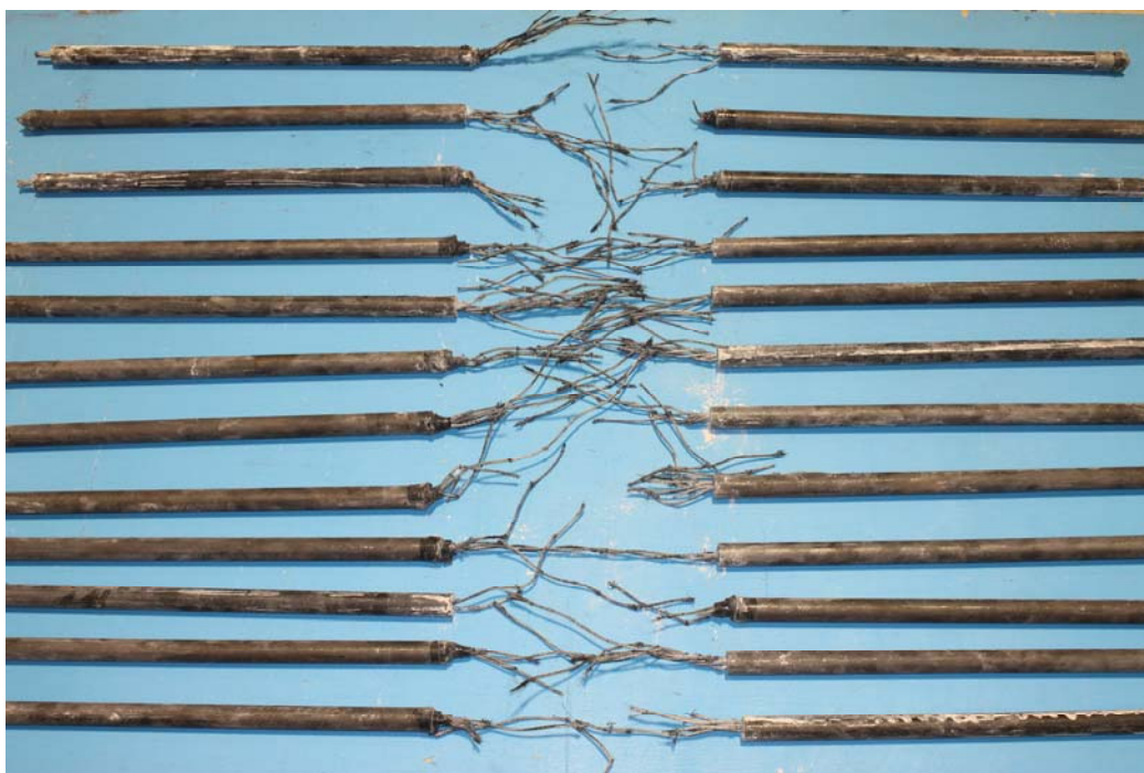
Figure 4.34: Mode of failure of conditioned specimens
