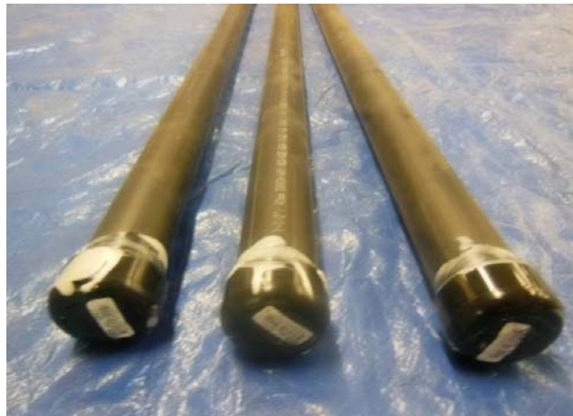
Figure 4.5: The ABS tubes and plastic caps
