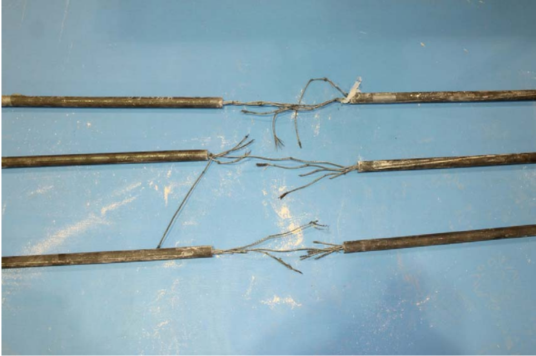
Figure 4.27: Mode of failure of conditioned specimens at 50°C with 1,000 hr
