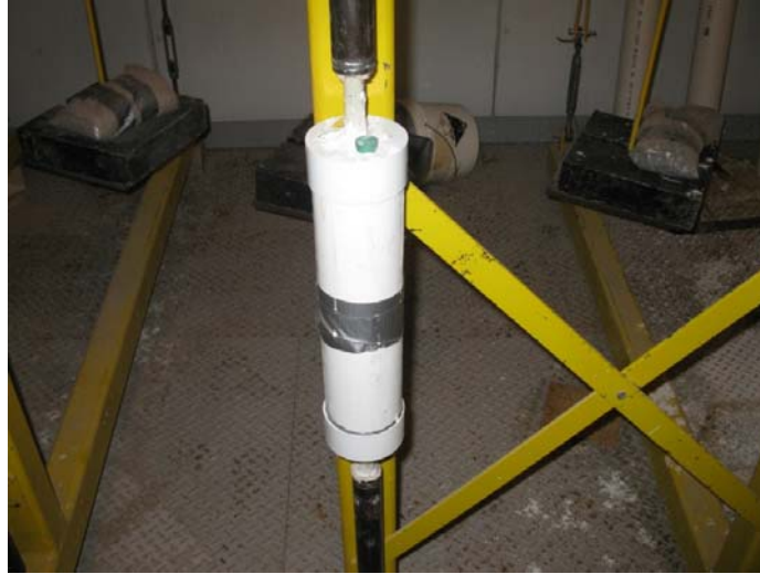
Figure 3.5: Test specimen with PVC cylinder filled with alkaline solution
