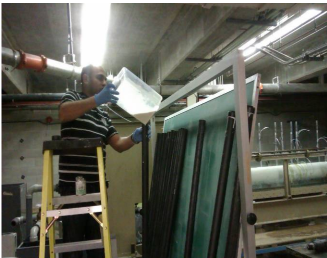
Figure 4.6: Filling the tubes with alkaline solution
