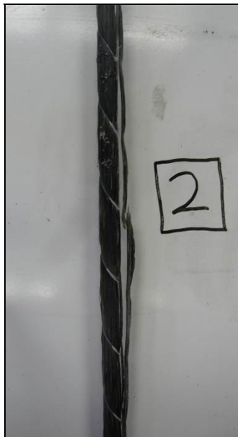
Figure 5.153: Specimen J8, failure at middle
