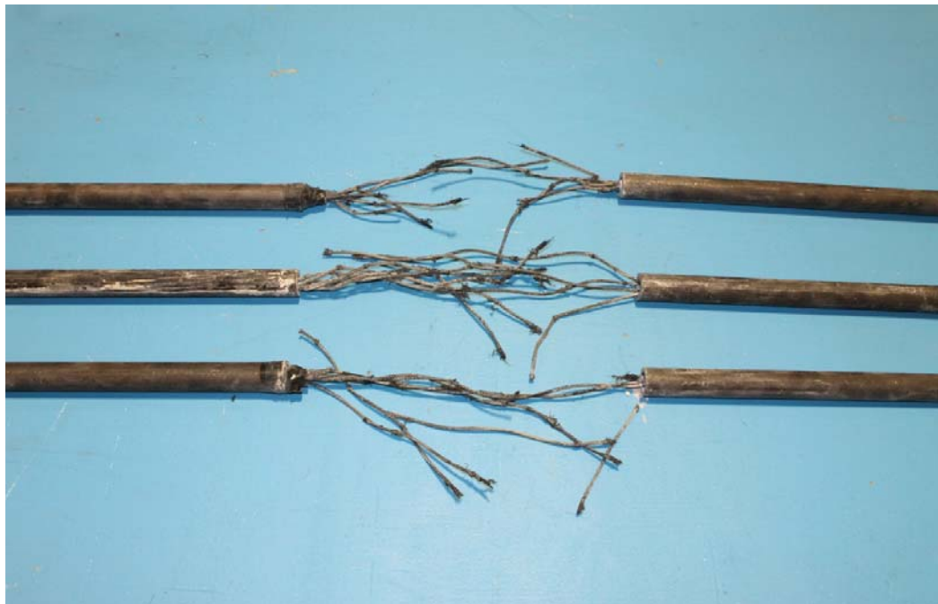
Figure 4.32: Mode of failure of conditioned specimens at 50° C with 3,000 hr
