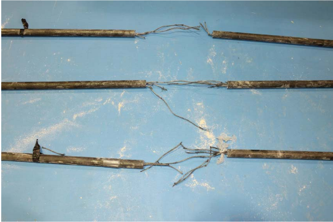
Figure 4.25: Mode of failure of conditioned specimens at 22°C after 1,000 hr
