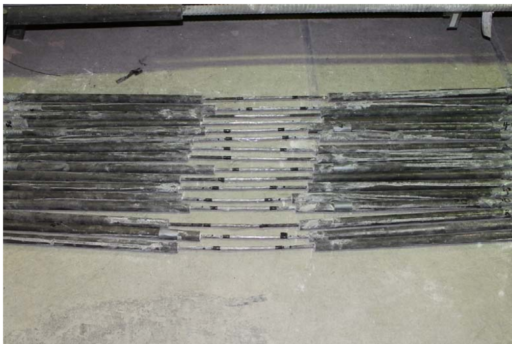
Figure 4.11: Test specimens attached with steel tubes
