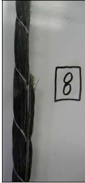
Figure 5.150: Specimen I8, typical failure of type I bars
