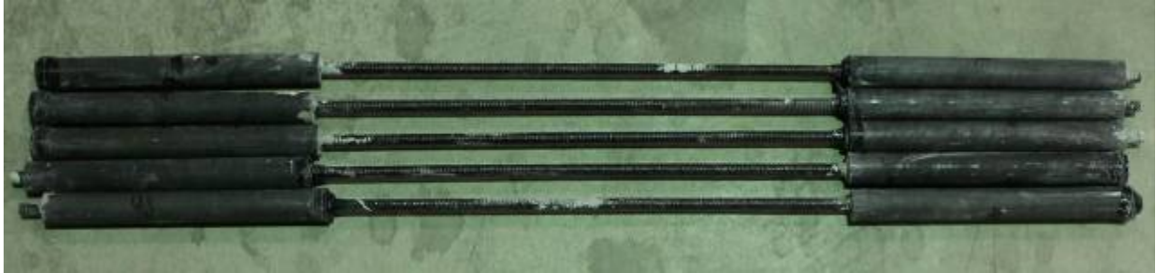
Figure 5.158: BASA BFRP bars of sizes 8 mm (code 43 and 5) before testing
