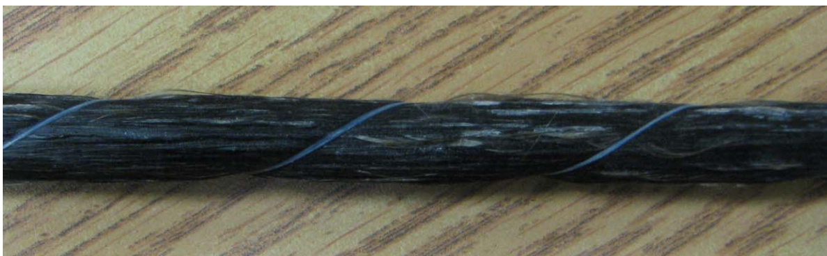
Figure 5.5: TECH BFRP bar of 12 mm- in diameter
