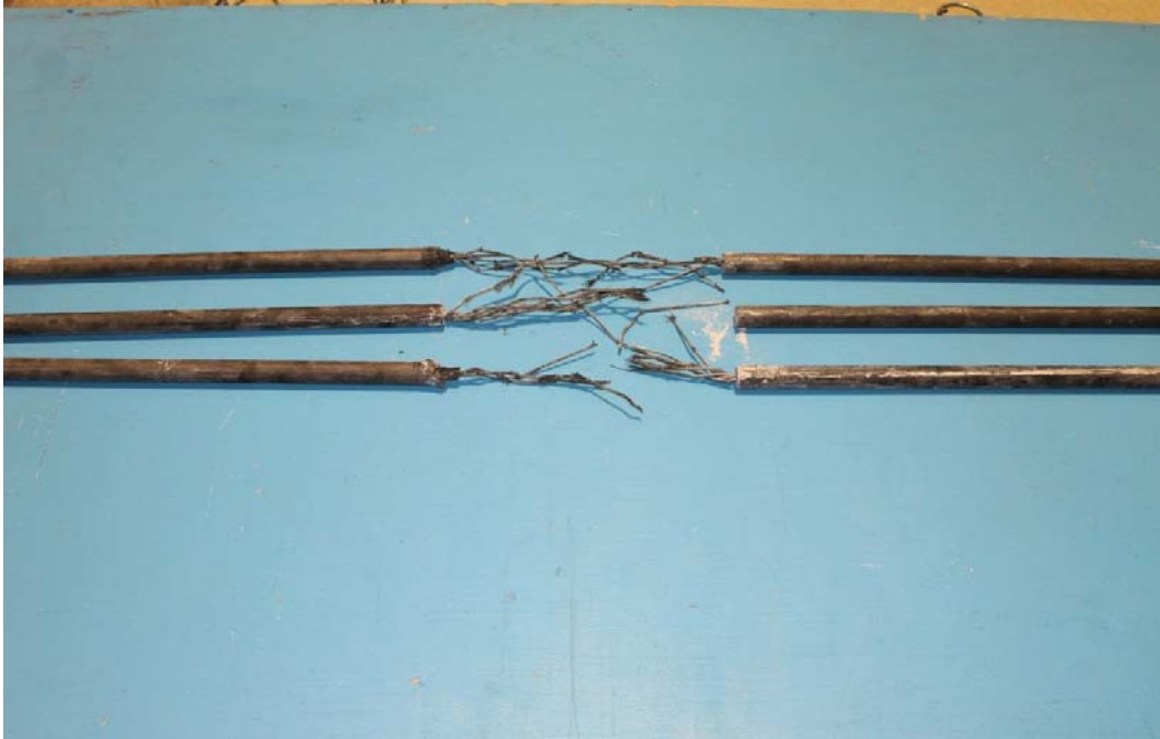
Figure 4.31: Mode of failure of conditioned specimens at 40° C with 3,000 hr
