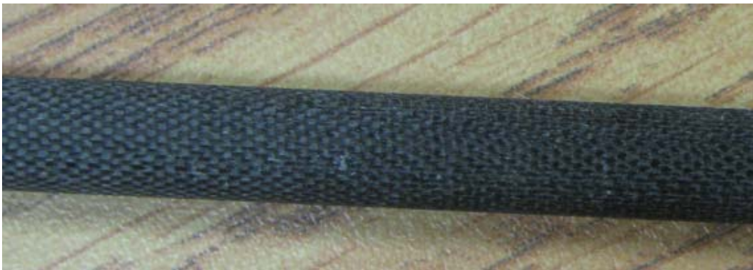
Figure 5.8: Prestressing tendon BFRP bar of 7 mm- in diameter
