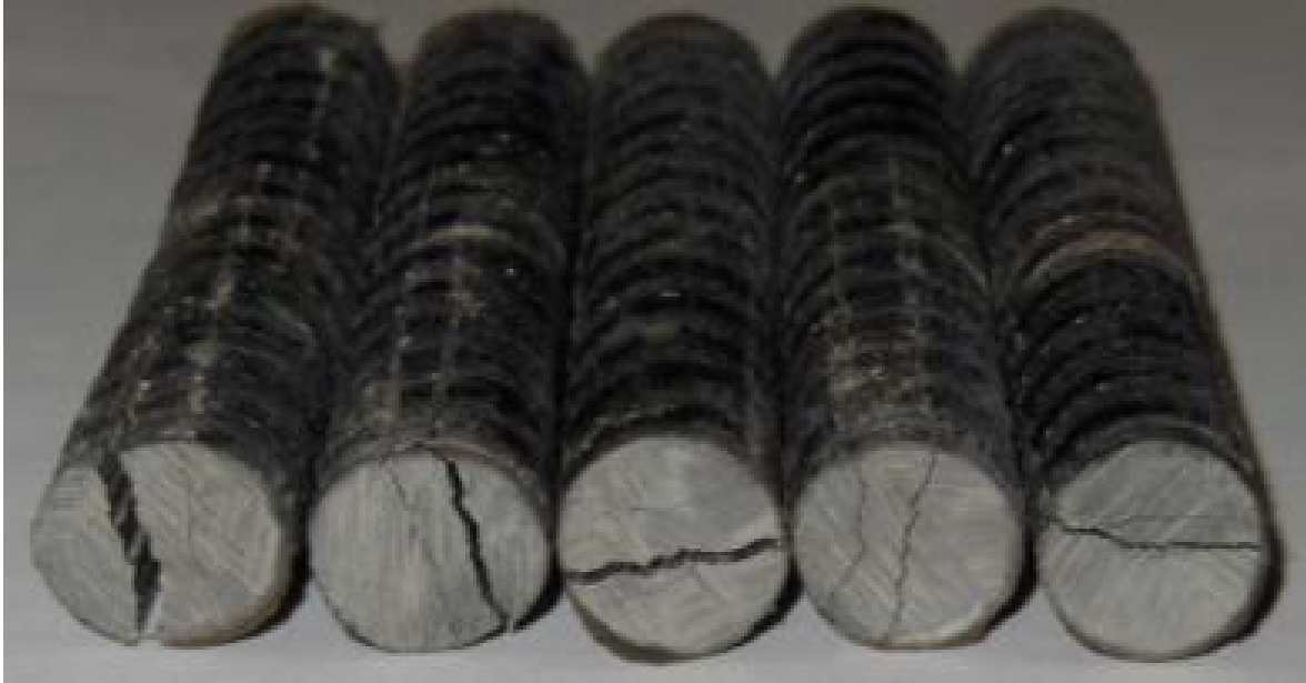
Figure 5.176: A typical apparent horizontal shear failure of the tested BASA BFRP bars
