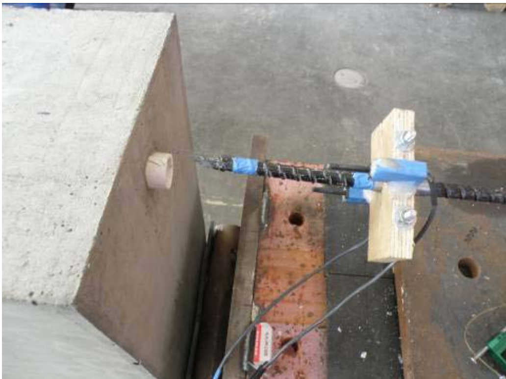
Figure 5.204: Rupture of type J BFRP bar
