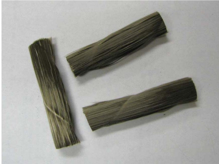
Figure 5.29: TECH BFRP 12-mm samples after pyrolysis
