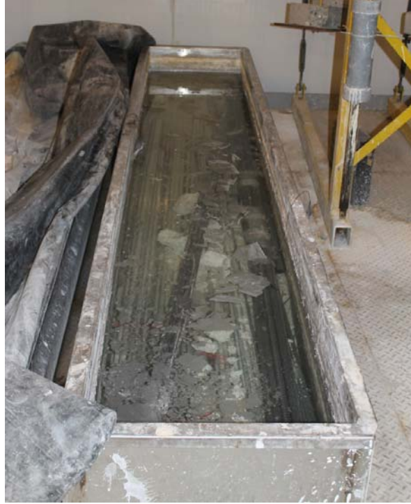
Figure 5.28: BFRP bars in conditioning at different environmental chambers
