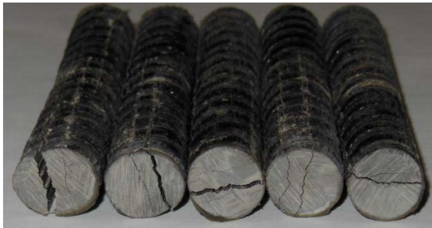
Figure 5.182: Apparent horizontal shear failure of the tested BASA BFRP bars
