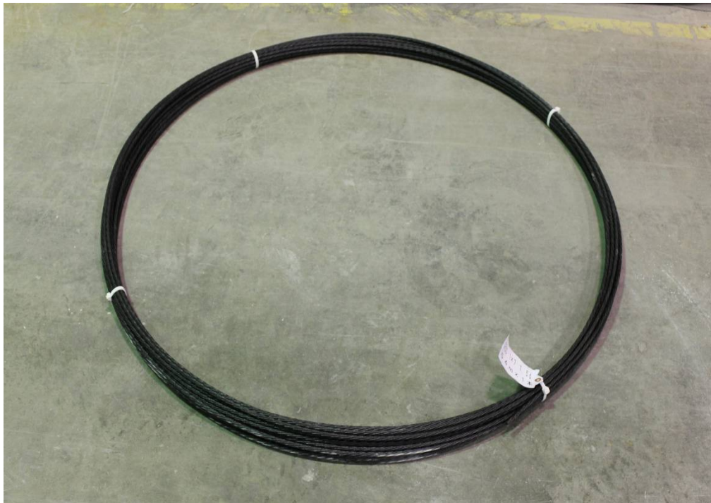
Figure 4.2: CFCC Tokyo Rope cable as received
