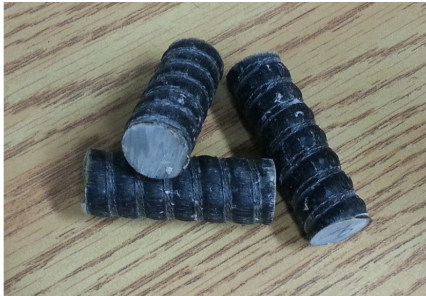
Figure 5.11: BASA-BFRP bars of 16 mm- in diameter
