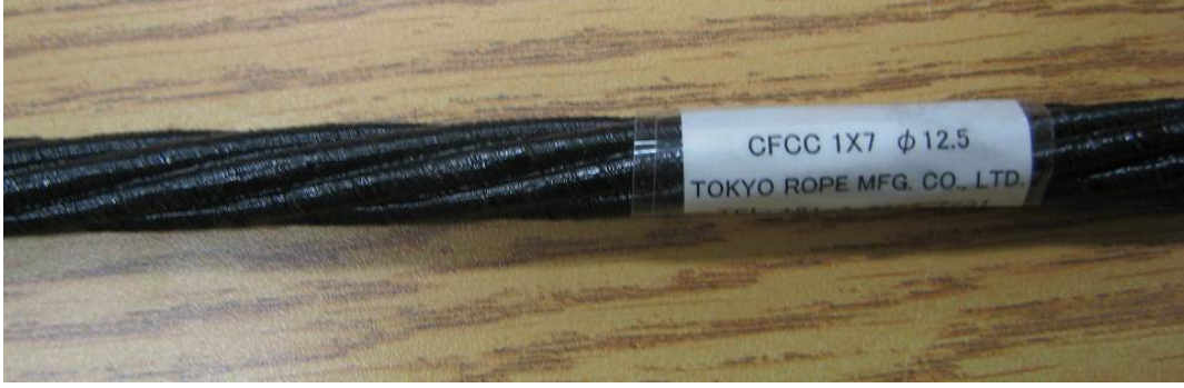
Figure 4.1: Carbon Tokyo Rope (CFCC 1X7)
