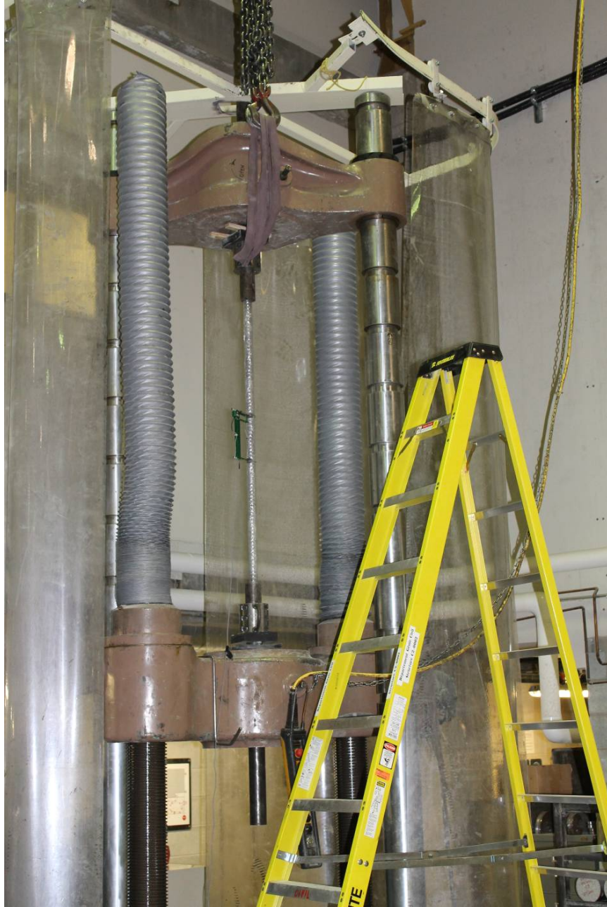
Figure 5.18: Tensile strength test setup
