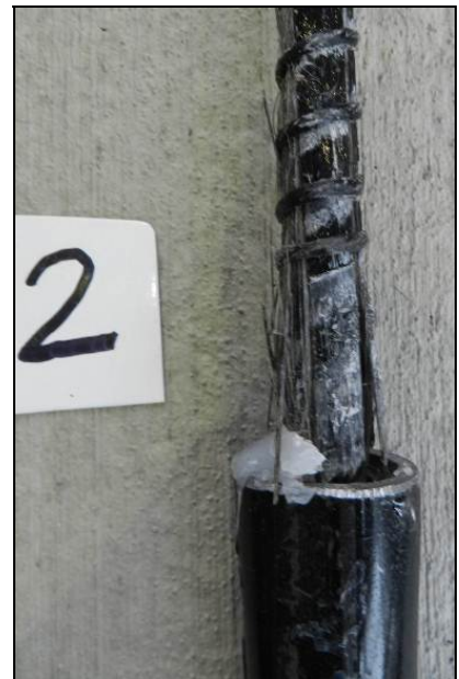
Figure 5.154: Specimen J9, failure near grip
