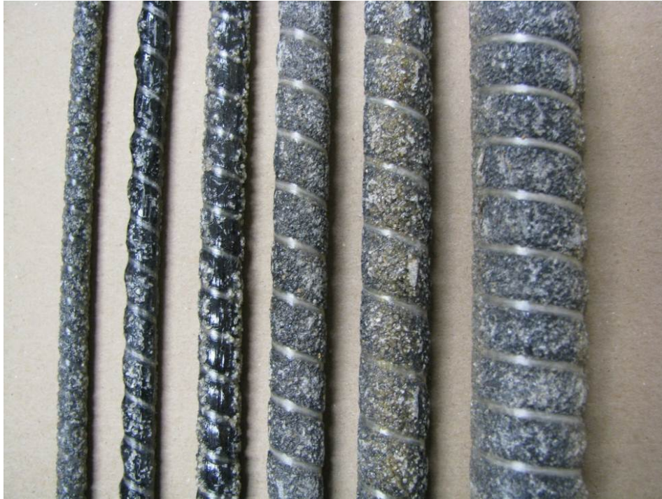
Figure 5.1: BFRP bars Type A (from left to right 6, 8, 10, 12, 16, and 25 mm-designated diameter)
