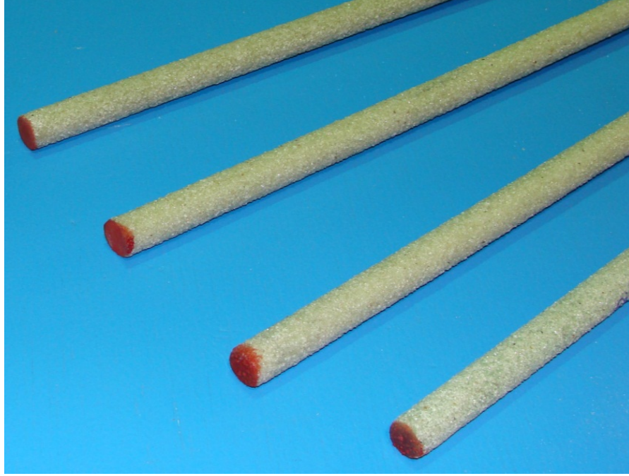
Figure 3.1: Sand coated GFRP bars
