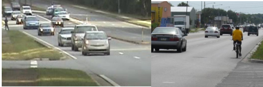
Figure 11 Outside through lane usage in the absence of bicyclist (left) and in the presence of bicyclist (right)
