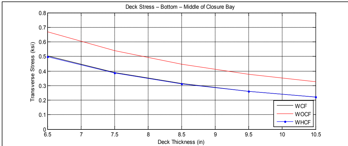
Figure A-46. Transverse deck stresses at Bottom -middle of closure pour vs. deck thickness for bridge SR-589 over Waters Avenue
