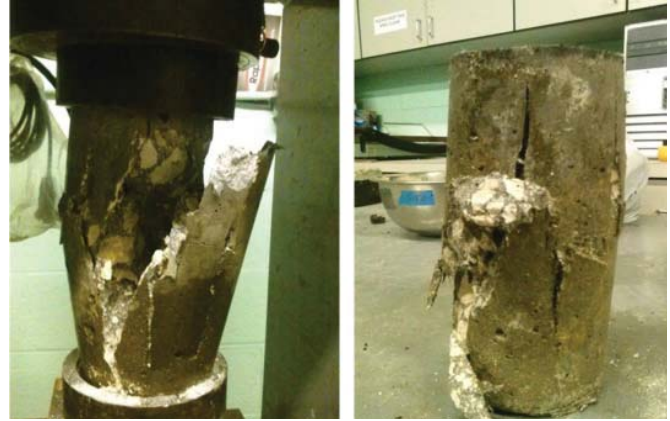
Concrete failure after compressive strength tests. Left: plain concrete. Right: Fiber reinforced concrete.
