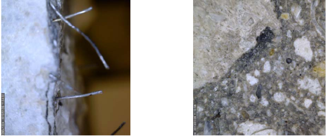
Figure 4.7 - Pull out of steel fibers. The holes on the right indicate pull out locations
