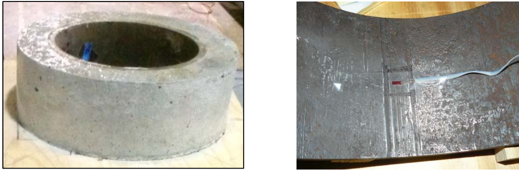
Figure 3.12 - Restrained shrinkage specimen and strain gages
