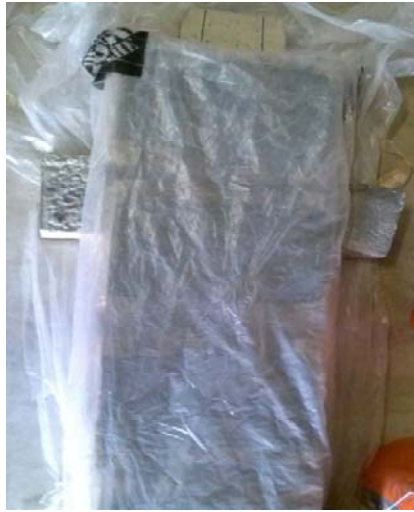
Figure 3.4 - Specimen protection and curing
