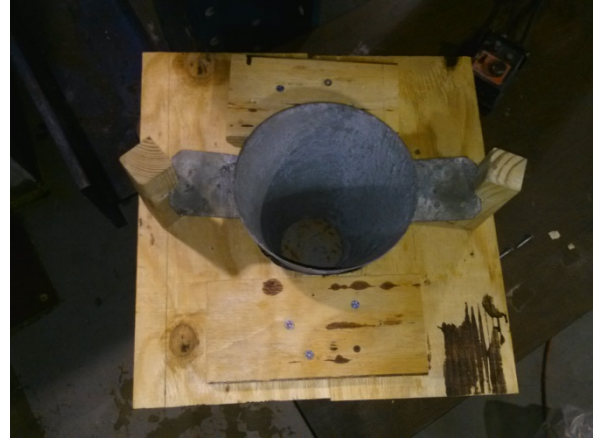
Figure 3.2 - Unit weight and time of flow measurements
