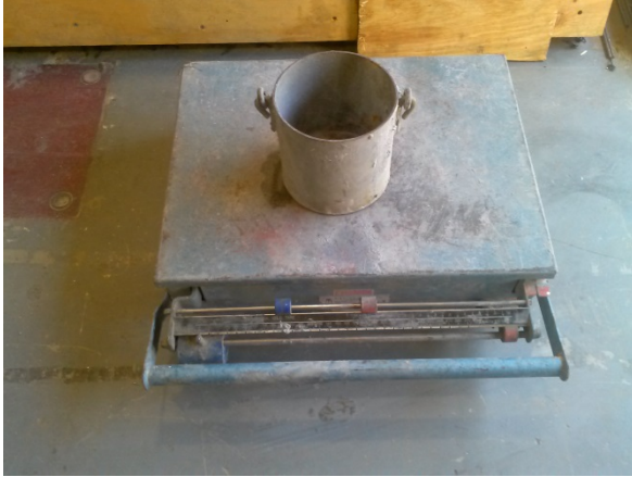
Figure 3.2 - Unit weight and time of flow measurements
