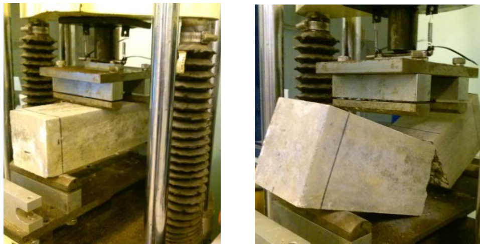
Figure 3.7 - Loading of specimen to failure
