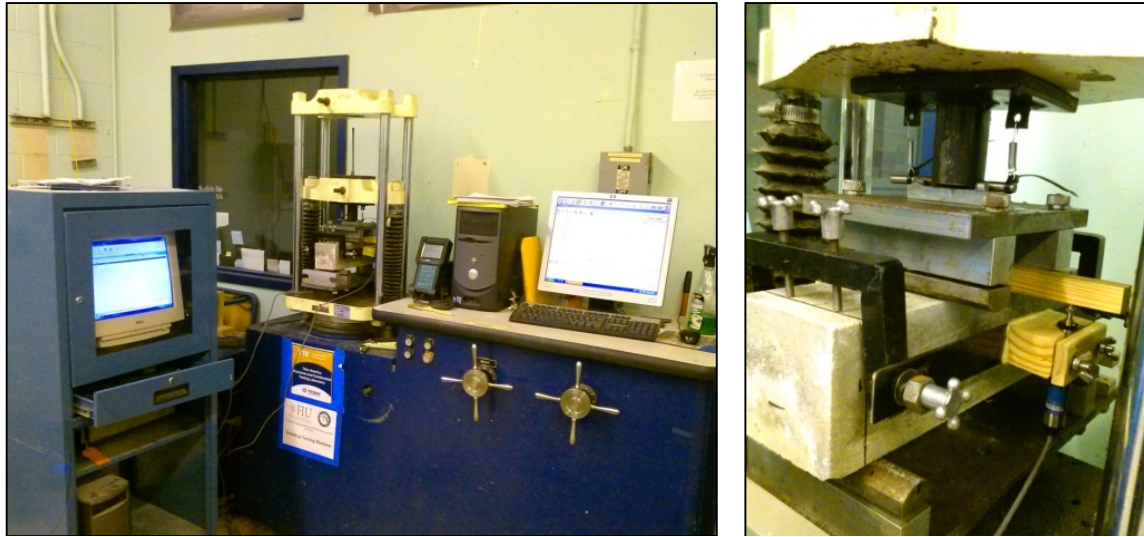
Figure 3.6 - Flexural test setup
