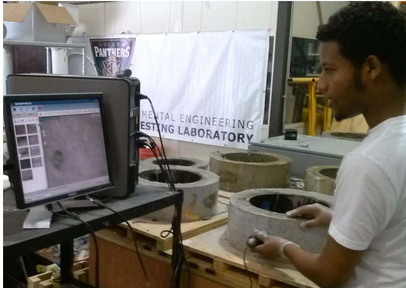
Figure 3.14 - Inspection of physical cracks
