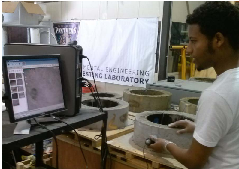
Figure 3.14 - Inspection of physical cracks
