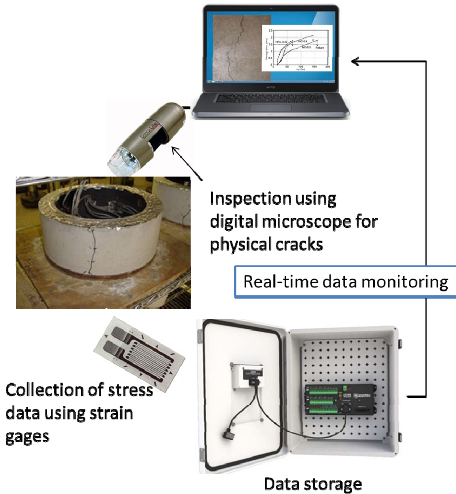
Figure 3.13 - Schematic of restrained shrinkage test
