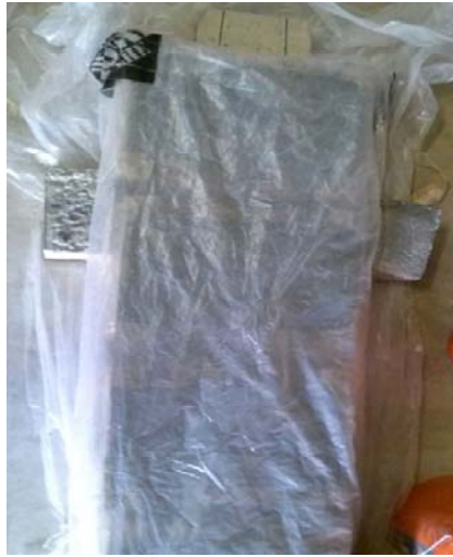
Figure 3.4 - Specimen protection and curing
