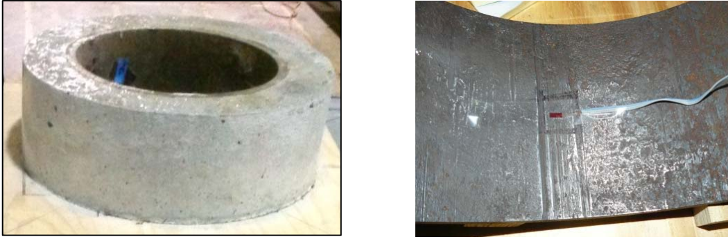
Figure 3.12 - Restrained shrinkage specimen and strain gages
