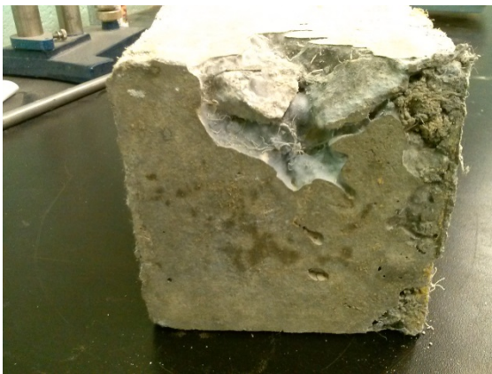
(a) pockets due to fiber balling
