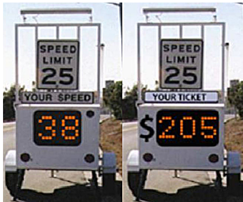
Focus groups assessed hybrid signs, for example, comparing the impact of showing a fine to showing driver speed.
