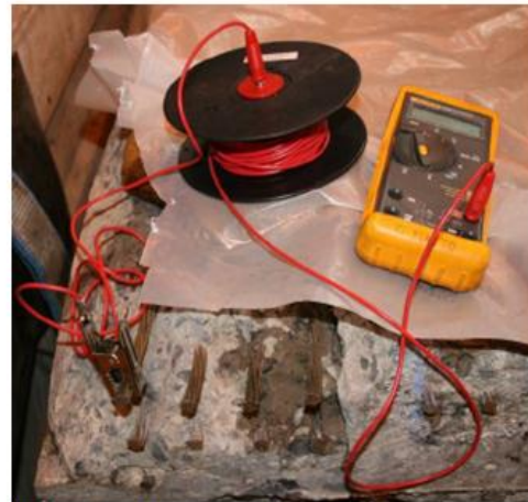
Electrical connection to strands
