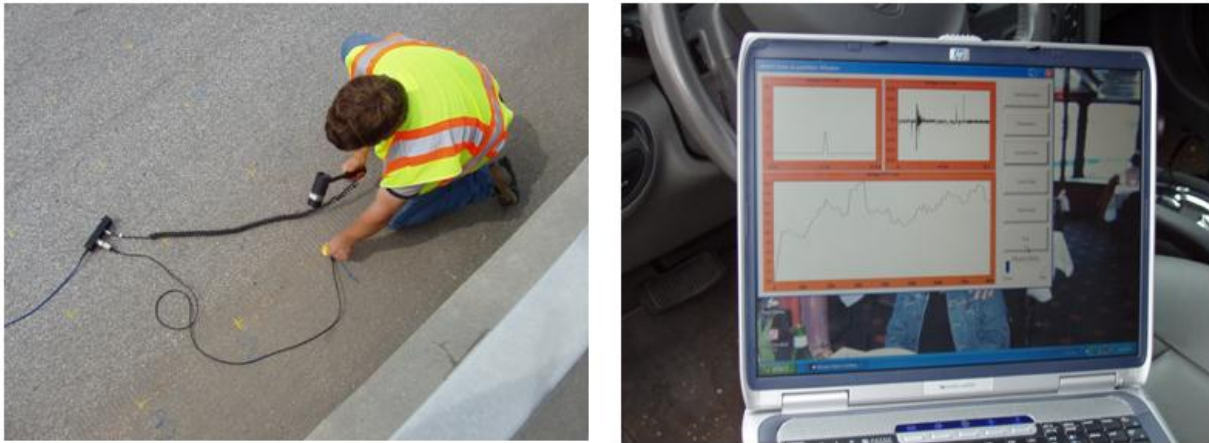
Figure A.19: Impulse response test equipment (left) and data acquisition software showing sensor outputs and computed mobility signal
