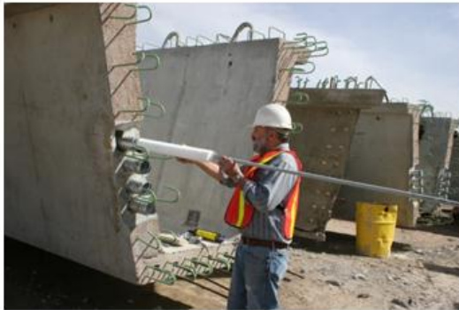
Figure A.17: Insertion of void (left) for Olson NCHRP idea 102 grant for impact echo scanning sensitivity research and grout/void defect plan built for south wall of PT bridge girder (right).
