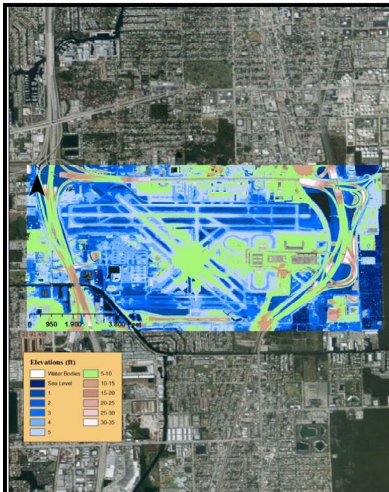
**Figure 34: Illustration of Fort Lauderdale Hollywood International Airport. LiDAR map shows runways are currently above SLR projections; however drainage areas are not above SLR projections (areas in dark blue color are less than 1 ft SLR and medium blue color are less than 3 ft SLR)**
