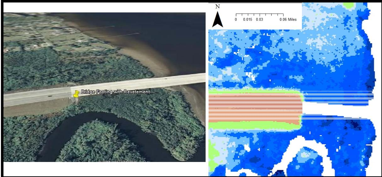
**Figure 28: Aerial photograph of the north end of the I-75 bridge (to the left) and FAU LiDAR map (to the right). The aerial shows the low-lying mangrove areas aside the bridge. As shown in the FAU LiDAR map, the ramp is well above the SLR projections. Note the bridge will show white like water bodies, because it is narrow in relation to the bridge.**
