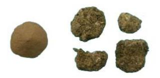
Fly ash (left) is more uniform in shape, while bottom ash (right) is more irregular. They differ in many other properties. Shown at the same size for comparison, bottom ash particles, averaging about a micron and ranging up to 50 mm, tend to be much larger than fly ash particles.
