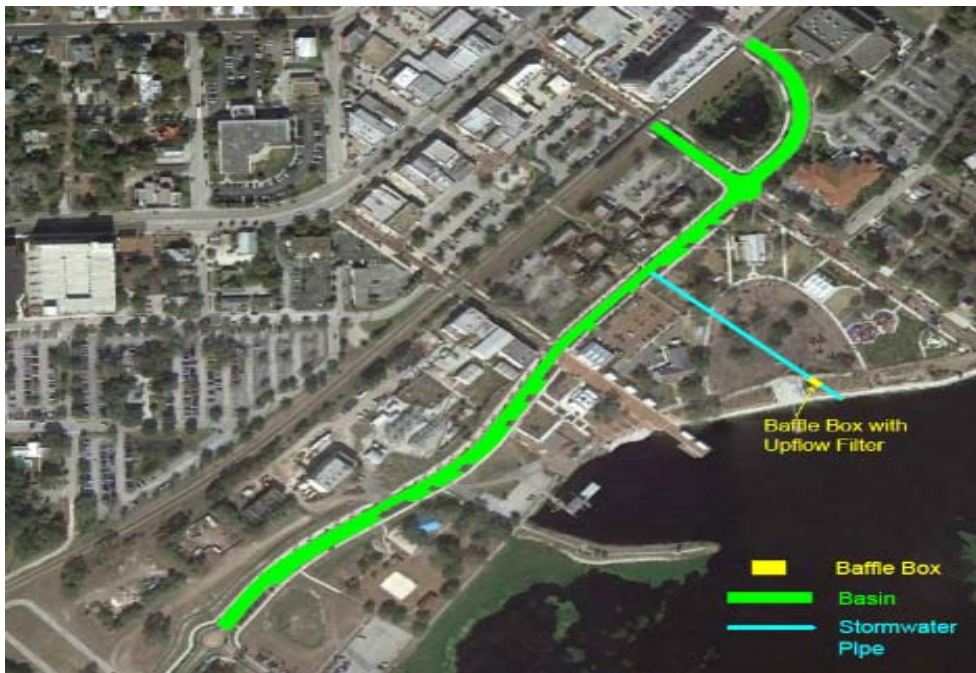
Figure 6-10 Impervious Catchment Area to On-line Sorption Filter
