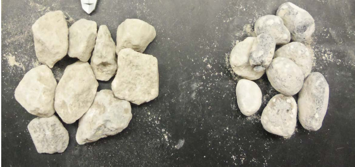
Figure 3.6: RCA Before (Left) and After (Right) L.A. Abrasion Test
