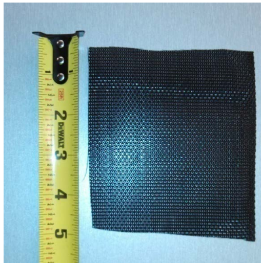
Figure 5.5: Photograph of Geotextile
