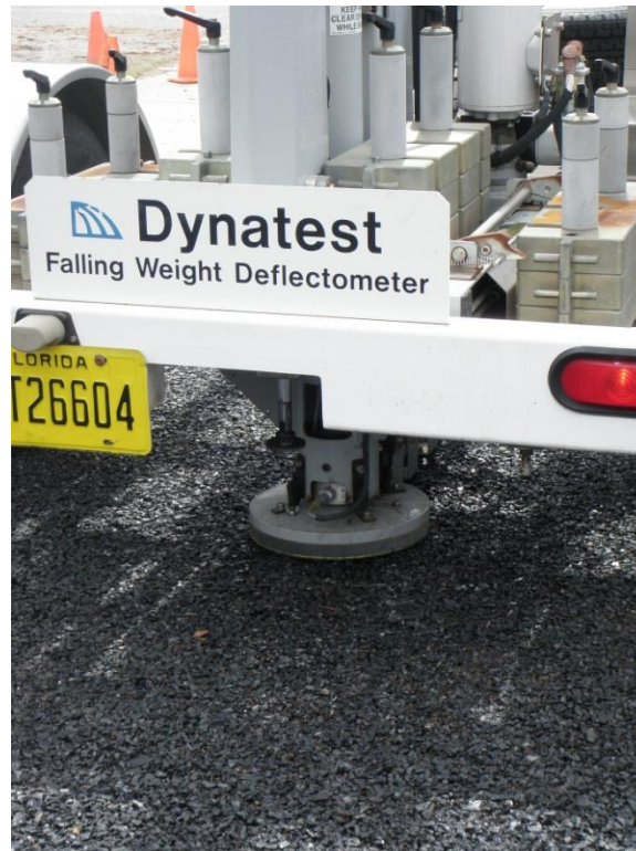
Figure 28: FWD test equipment on FlexiPave section
