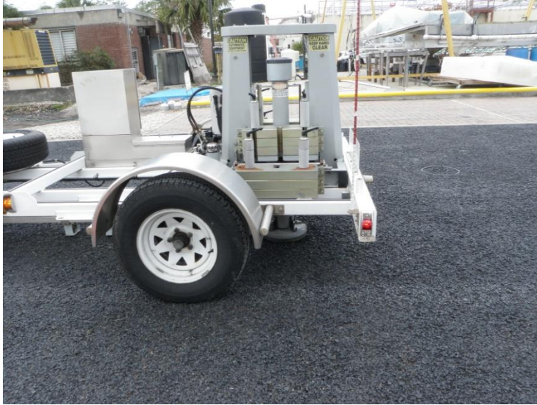
Figure 29: FWD conducting test on FlexiPave section
