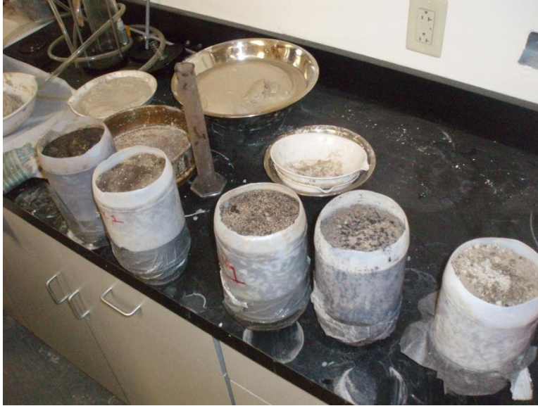
Figure 24: Half gallon containers draining by gravity
