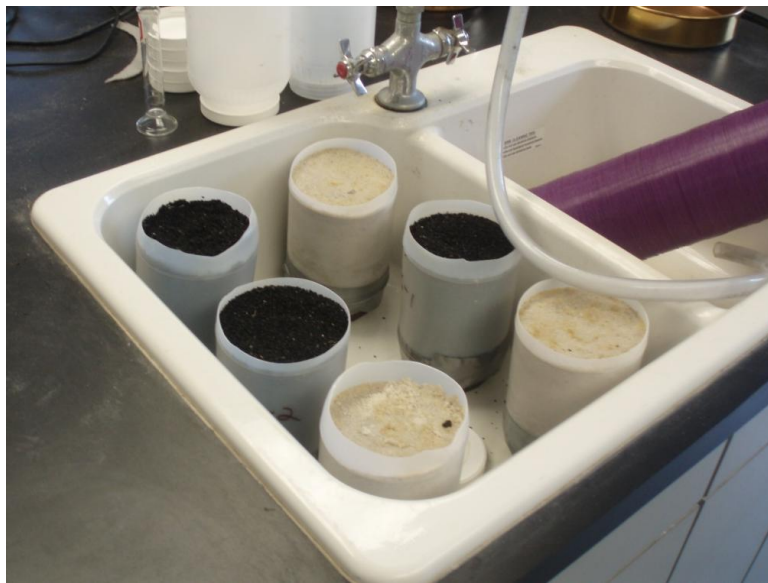
Figure 17: Half Gallon Jars draining by gravity
