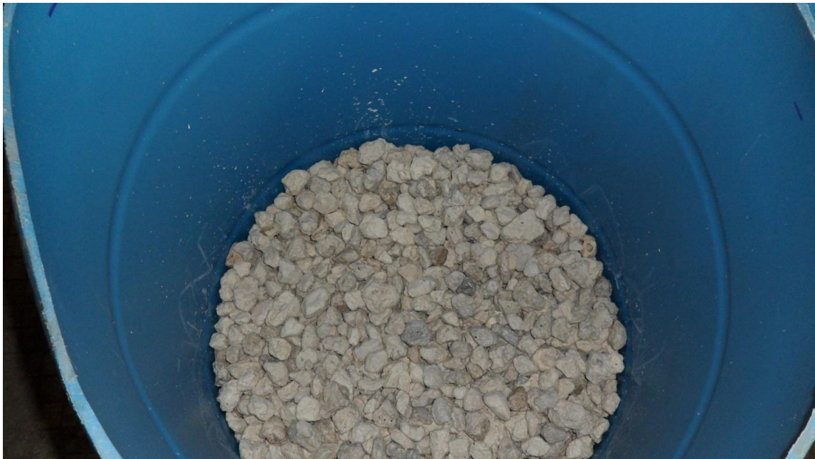
Figure 24: 4 Inches of #57 Stone Compacted
