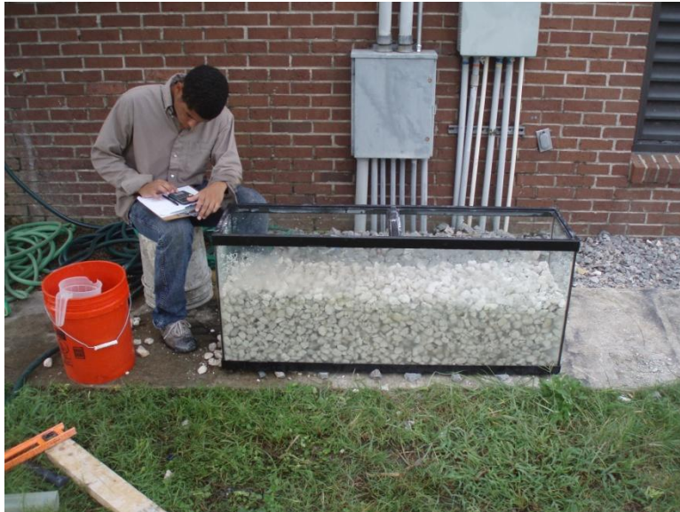
Figure 15: Number 4 Aggregates tested in large glass aquarium (12" x 19" x 47")
