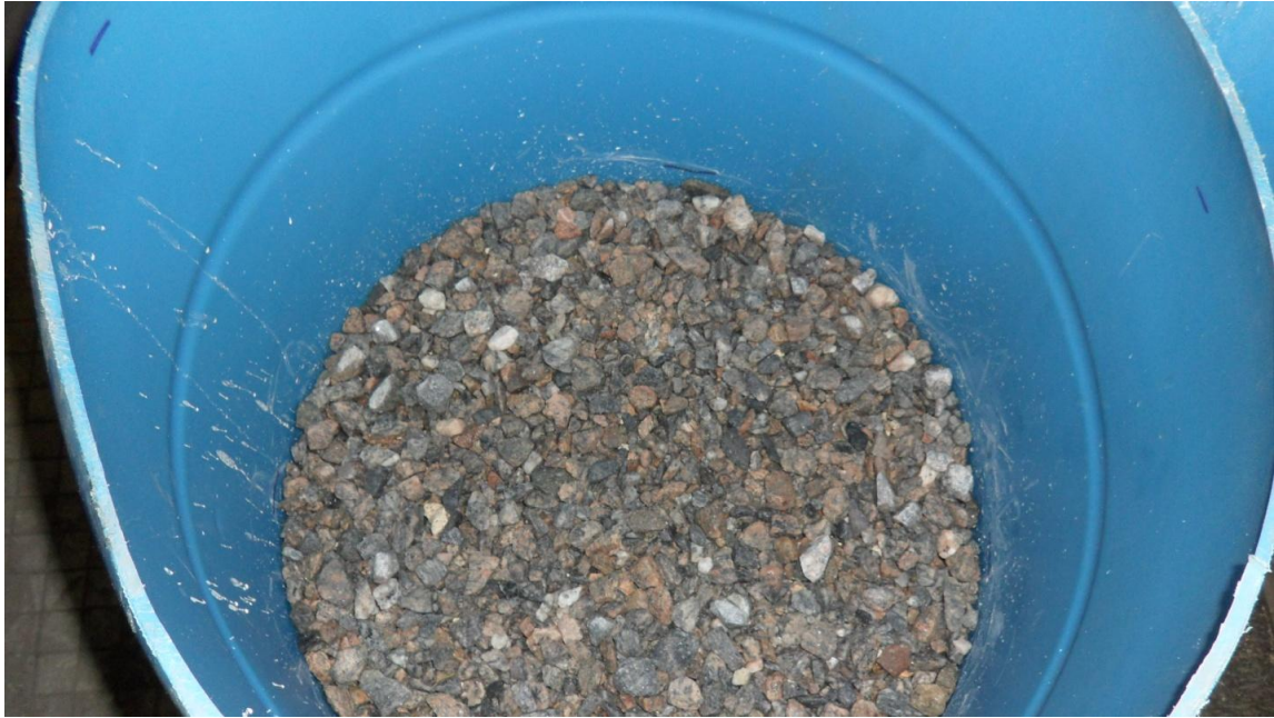
Figure 23: 5 Inches of #4 Stone Compacted
