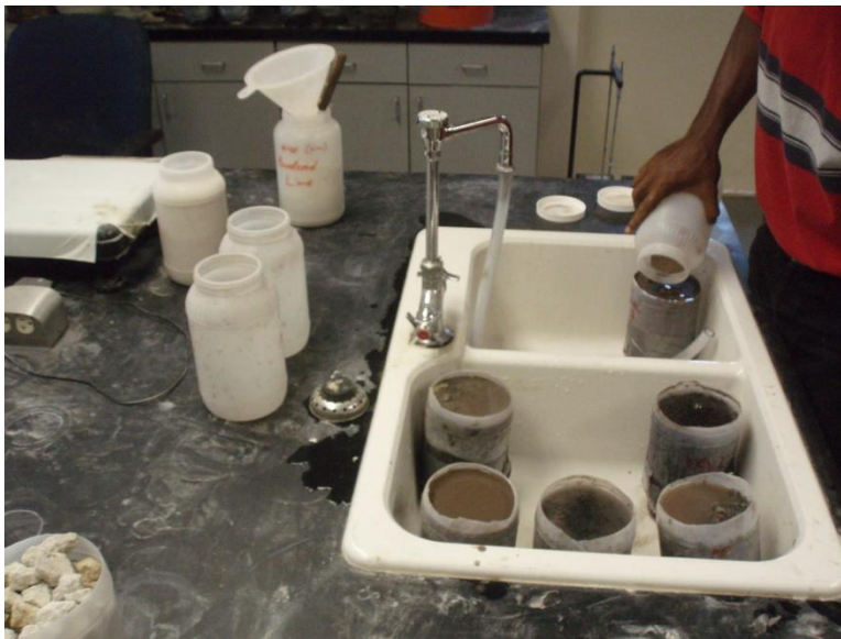
Figure 13: Half Gallon containers being loaded with sediments
