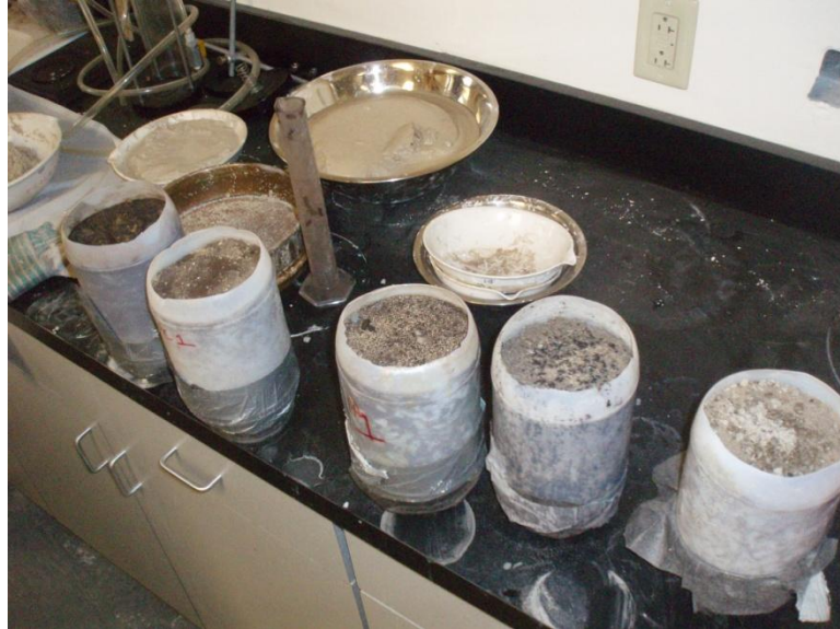
Figure 25: Half Gallon containers draining by gravity
