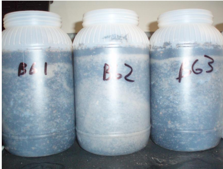
Figure 22: Half Gallon container for component testing of Porous Asphalt
