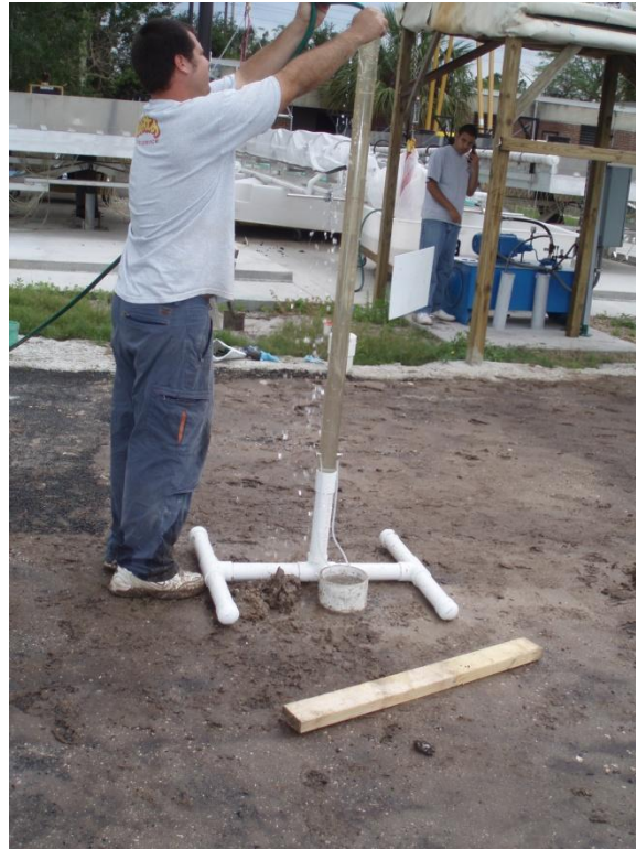
Figure 12: Post sediment loading ERIK testing on “deep” infiltrometer
