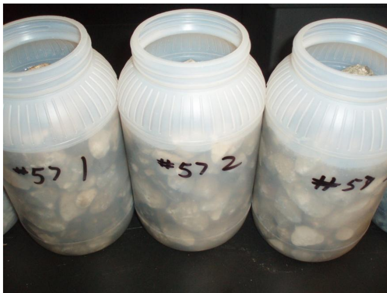
Figure 21: Half Gallon container for component testing of Porous Asphalt
