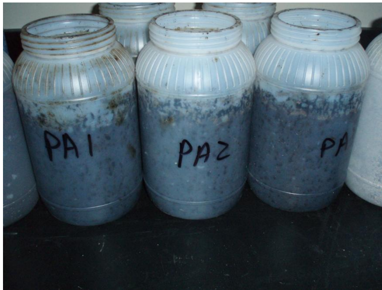
Figure 20: Half Gallon container for component testing of Porous Asphalt
