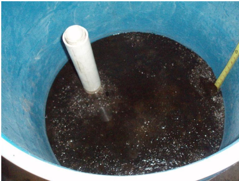
Figure 28: Sediment being washed into the porous asphalt system
