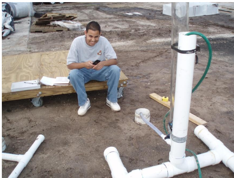
Figure 12: Post sediment loading ERIK testing on “deep” infiltrometer
