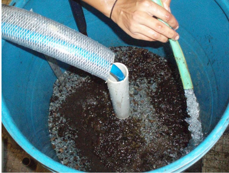
Figure 45: Washing loaded sediments into pores while pumping infiltrated water out through well pipe
