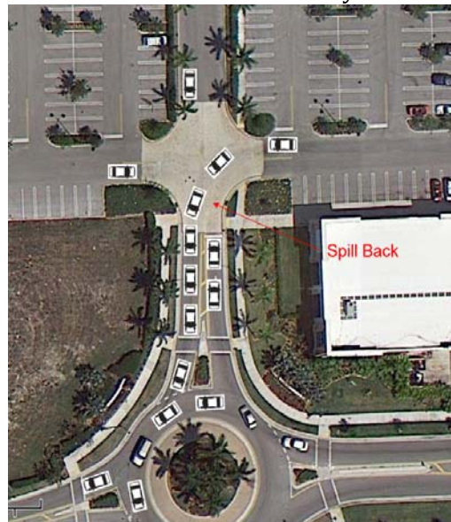
Figure 56. Roundabout Observation on Spill Back of Entering Traffic into an Adjacent AWSC Intersection (NE 10th Ct. and SW 152 nd Ave., Miami)
