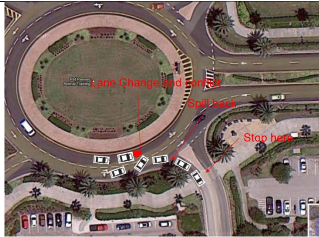
Figure 59. Roundabout Observation with Spill Back from Driveway into Circulating Lanes (Causeway Blvd. and Mandalay Ave., Pinellas County)
