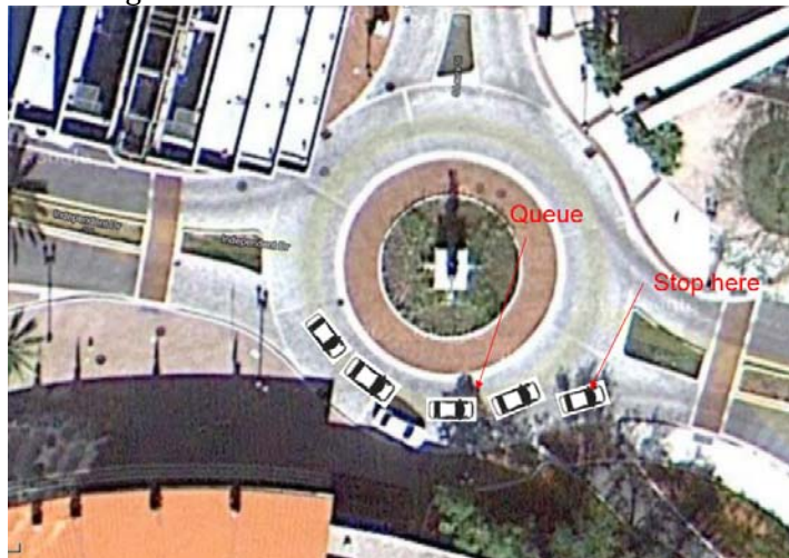
Figure 58. Roundabout Observation with Driver Violation of Traffic Rules (Independent Dr. and S. Laura St., Duval County)
