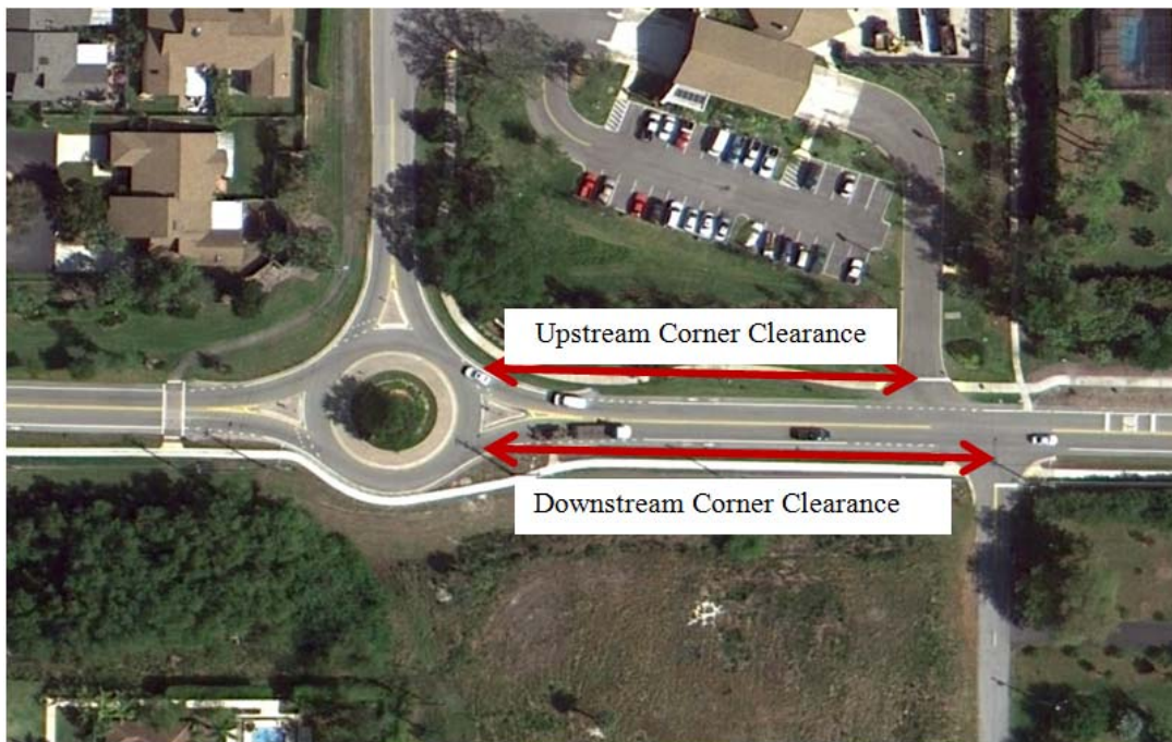
Figure 39. Upstream and Downstream Driveway Corner Clearances
