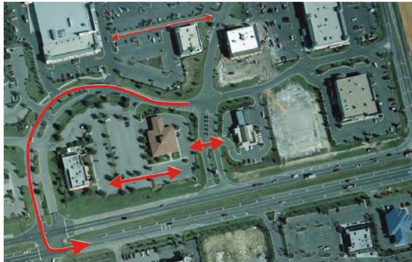
Figure 28. Joint and Cross Access (FDOT, 2008, p. 86)
