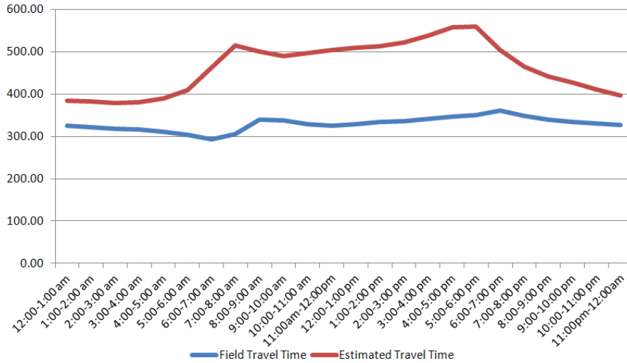
Figure 4-5 Comparison between Field Data and the Estimated Travel Time without Consideration of the “Yellow Flashing” Scenario
