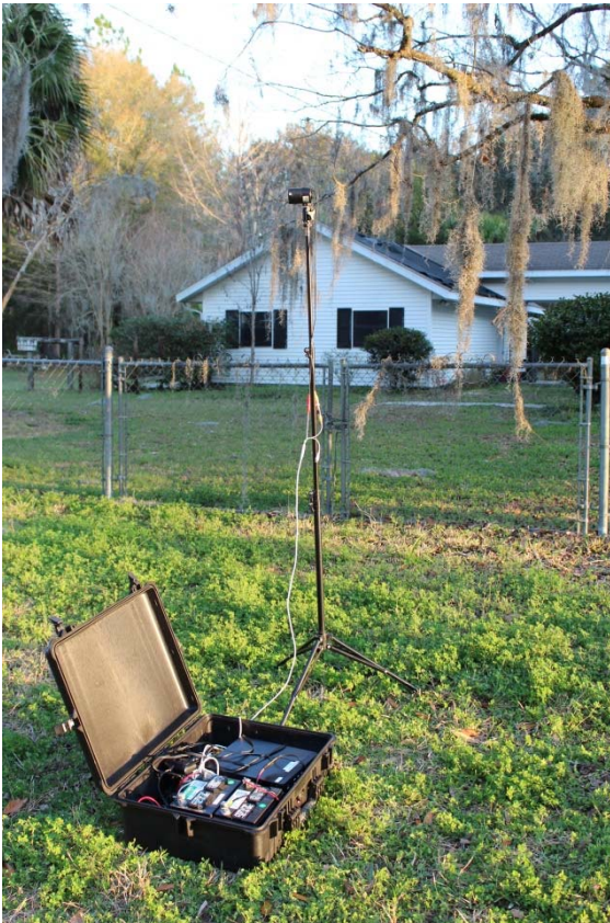
Figure 10. Video camera and external hard drive recorder setup used for data collection
