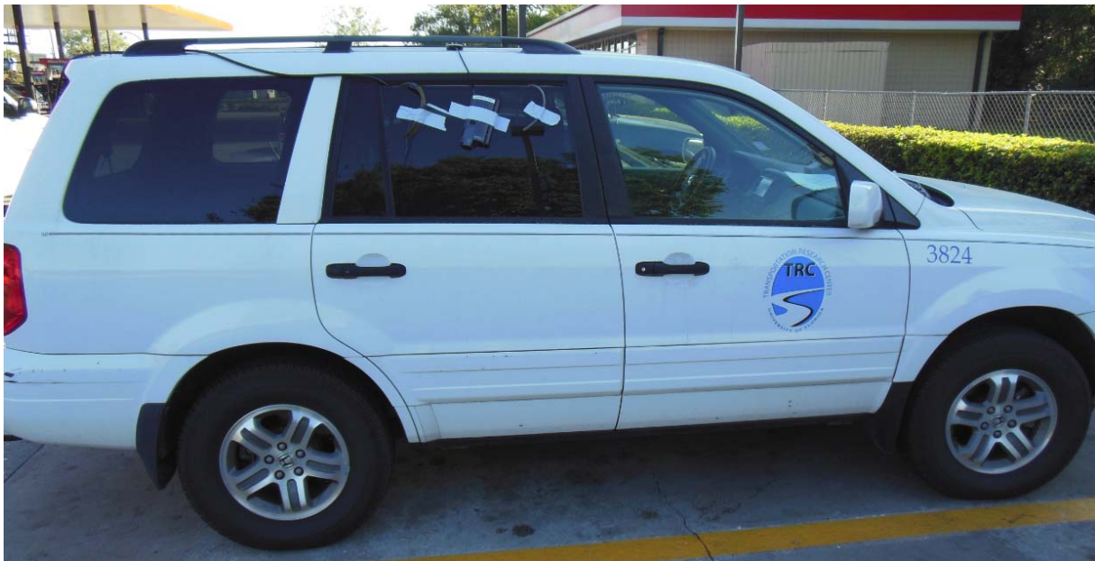
Figure 11. Instrumented Honda Pilot used to collect data inside work zone
