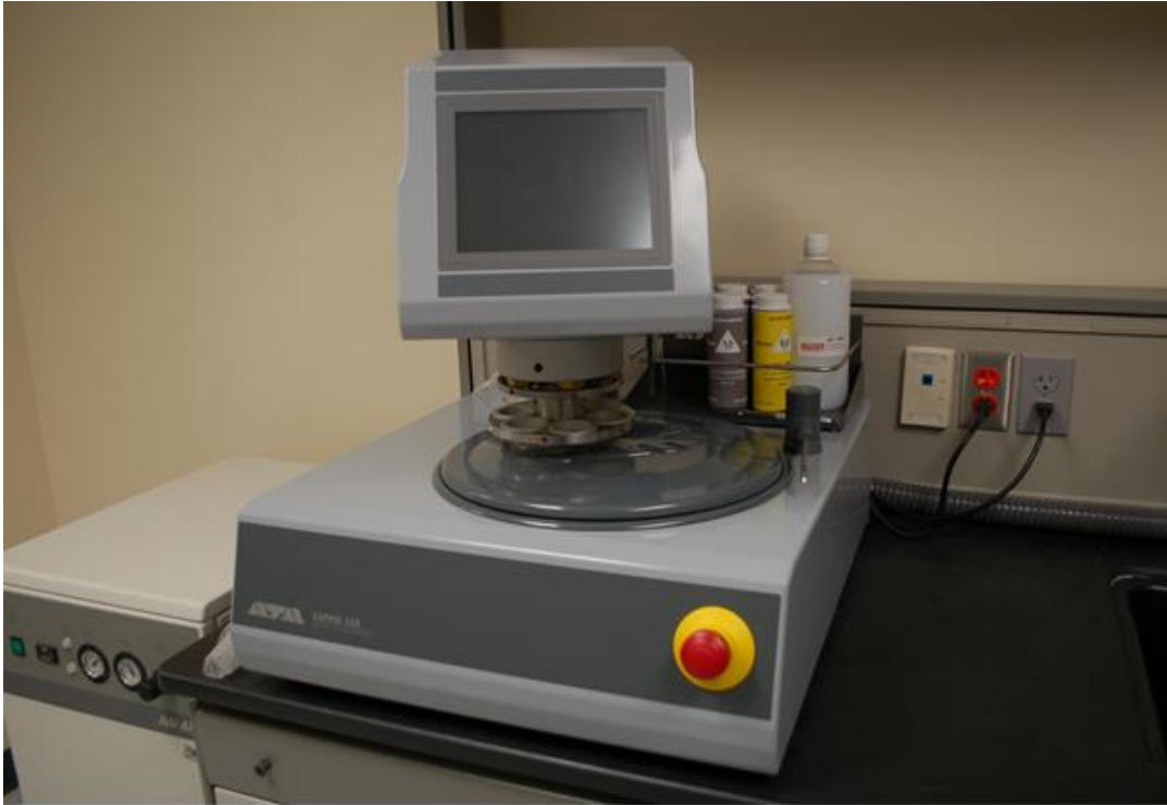
Figure 4-1: Saphir 550 Semi Automated Grinder Polisher
