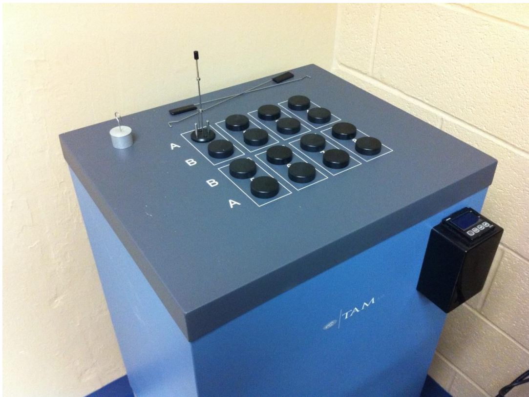
Figure 3-7: Tam Air Isothermal Calorimeter with Sample and Admix Ampoule Loaded
