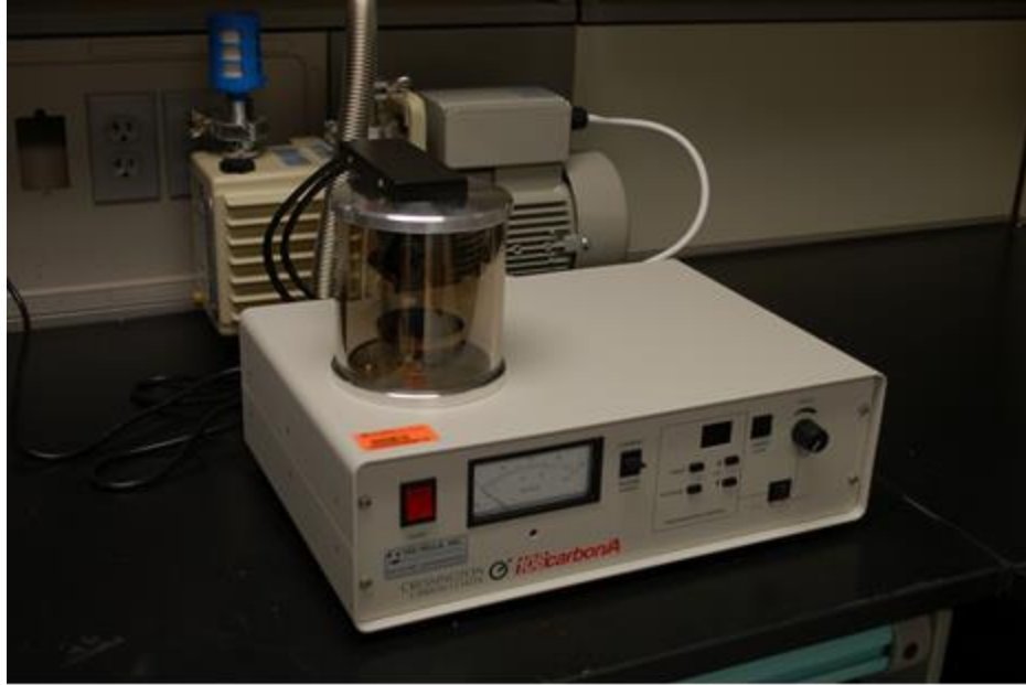
Figure 4-3: Evaporative Carbon Coater
