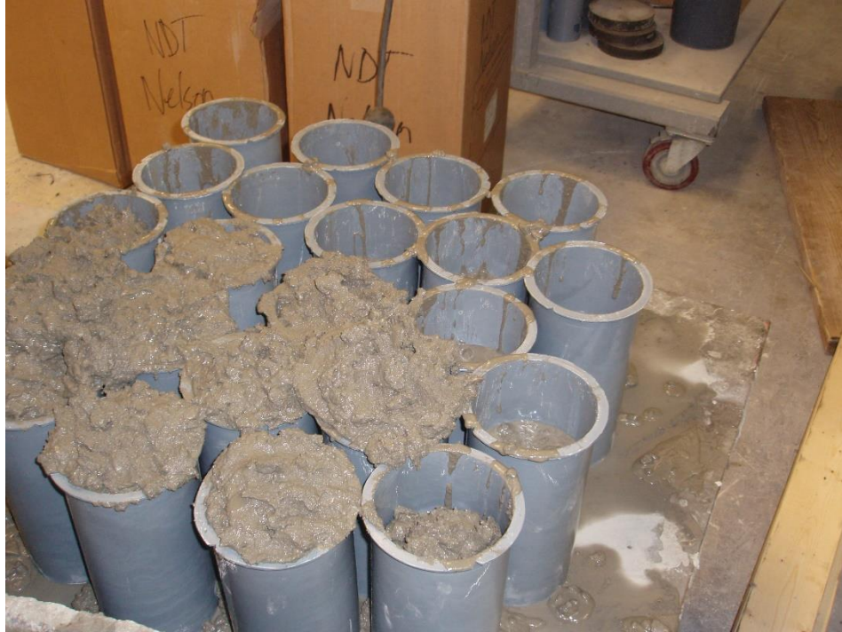
Figure 6-1: Preparation of Cylinders
