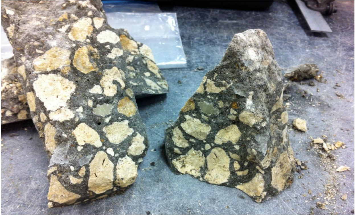
Figure 7-33: Crushed Cylinder Fragments
