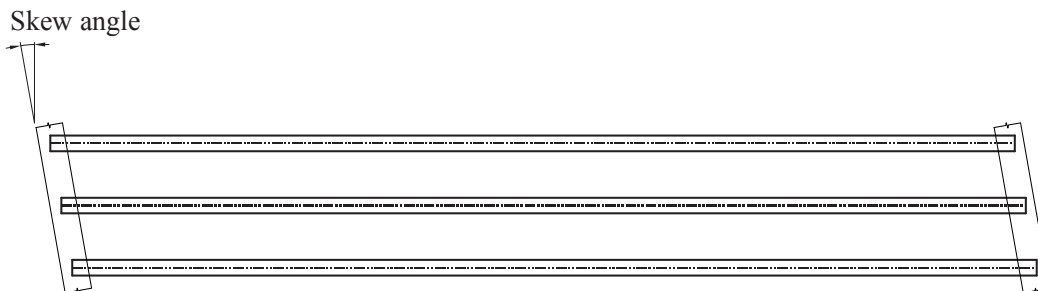
Figure 2.4 Definition of skew (plan view)
