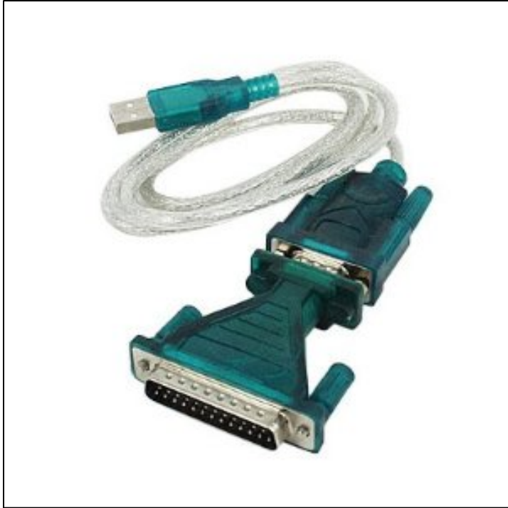
Figure 3-9. Method for converting a 25-pin RS-232 output to USB
