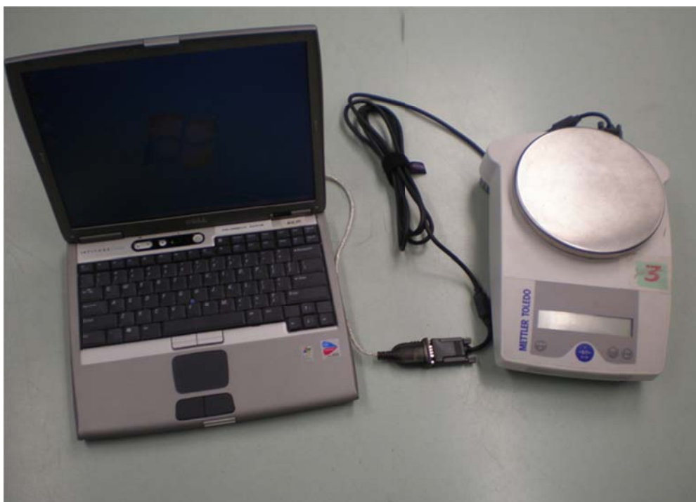
Figure 3-8. Photograph of laptop, serial converter, and additional cable connected to digital scale.
