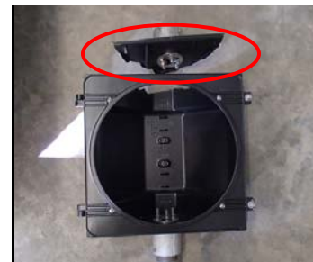
Figure A-28. SH2.3 failure mode, break off around top surface
