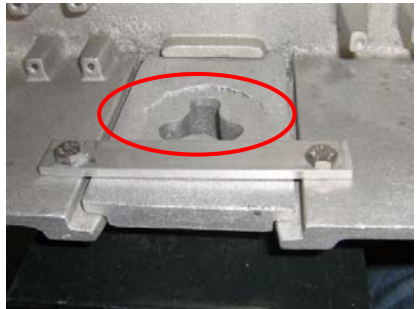
Figure A-72. DL2.3 failure mode, adapter hub failure
