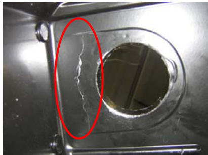
Figure A-22. SH1.1 failure mode, crack at top connection
