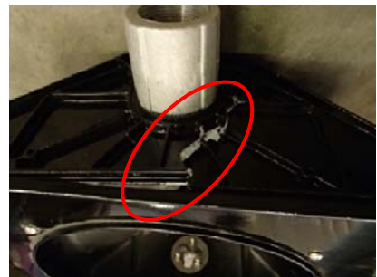
Figure A-32. SH3.3 failure mode, crack at top connection
