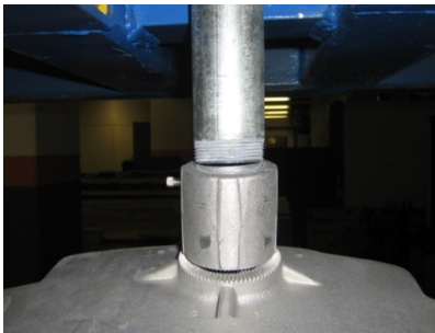
Figure A-14. DL2.1 failure mode, attachment hardware
