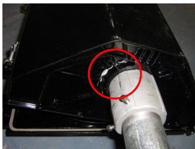
Figure A-87. SH3.2 failure mode, crack at top connection
