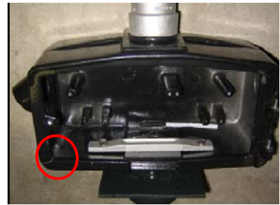
Figure A-68. DL1.3 failure mode, crack in bottom corner
