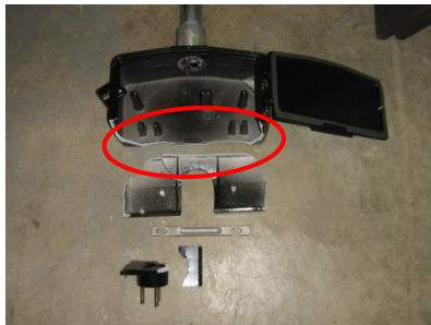
Figure A-66. DL1.1 failure mode, adapter hub, crack around bottom
