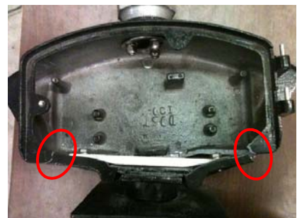
Figure A-4. DS1.3 failure mode, crack in bottom corner
