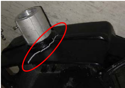
Figure A-18. DL3.1 failure mode, crack at top connection
