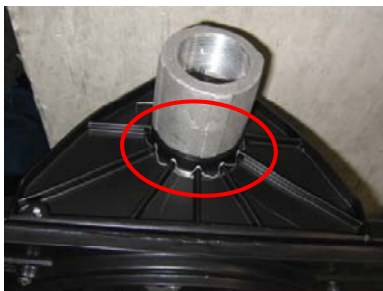
Figure A-26. SH2.1 failure mode, crack at top connection
