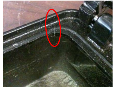
Figure A-20. DL3.3 failure mode, crack in top corner
