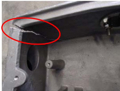
Figure A-11. DL1.2 failure mode, crack in top corner
