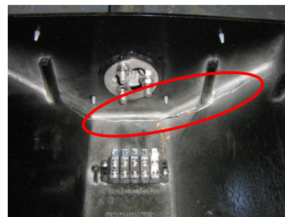
Figure A-88. SH3.3 failure mode, crack around top surface
