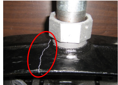
Figure A-76. DL3.3 failure mode, crack at top connection
