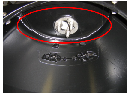
Figure A-92. SH4.3 failure mode, crack around top corner
