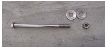
Figure B-14. Reinforcement attachment hardware
