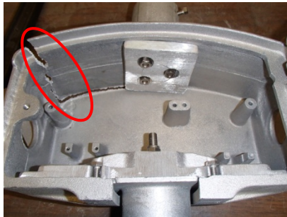
Figure A-99. RDS1.2 failure mode, crack in top corner
