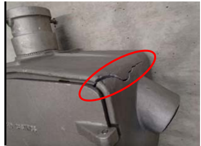
Figure A-12. DL1.3 failure mode, crack in top corner
