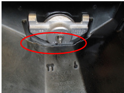
Figure A-106. RSH1.1 failure mode, crack in top of signal
