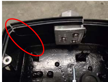
Figure A-47. RDL1.2 failure mode, crack starting in top corner
