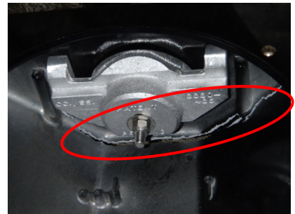
Figure A-112. RC1.3 failure mode, cracking in signal
