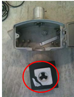
Figure A-7. DS2.2 failure mode, adapter hub failure
