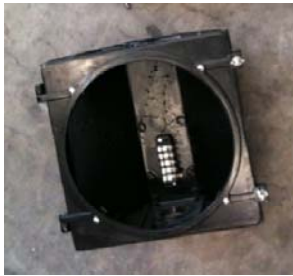
Figure B-1. 12 inch aluminum signal head
