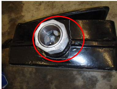
Figure A-103. RDL1.2 failure mode, crack around top reinforcement
