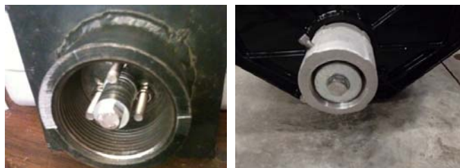
Figure 3-8. Use of washers in reinforced disconnect and signal head testing (photos courtesy of author)
