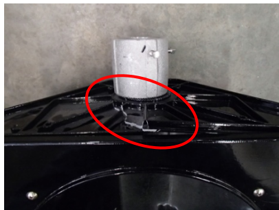
Figure A-31. SH3.2 failure mode, crack at top connection
