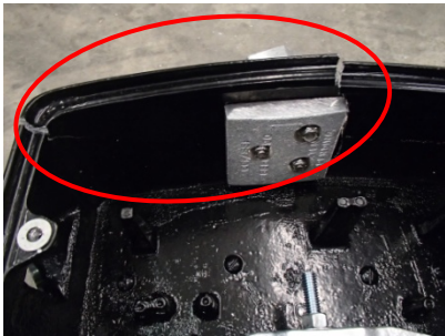
Figure A-54. RC1.1 failure mode, crack around top
