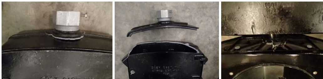
Figure 4-11. Combination failure modes, flexure (photos courtesy of author)
