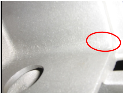
Figure A-70. DL2.1 failure mode, crack in top corner
