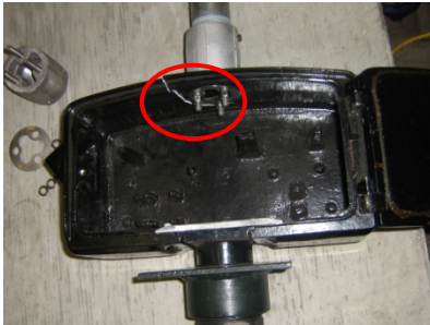
Figure A-74. DL3.1 failure mode, crack at top connection
