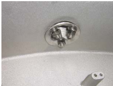
Figure A-15. DL2.2 failure mode, attachment hardware
