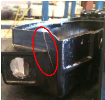
Figure A-2. DS1.1 failure mode, crack in bottom corner
