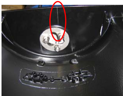
Figure A-34. SH4.1 failure mode, crack at top connection
