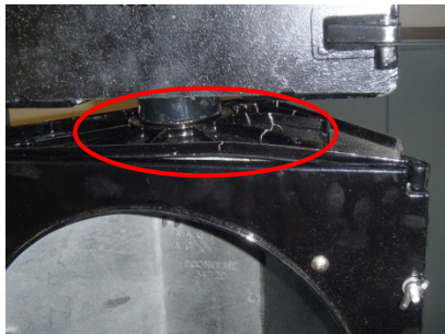
Figure A-110. RC1.1 failure mode, crack in top of signal
