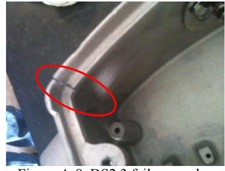
Figure A-8. DS2.3 failure mode, crack in top corner
