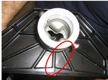
Figure A-23. SH1.2 failure mode, crack at top connection
