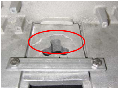
Figure A-71. DL2.2 failure mode, adapter hub failure
