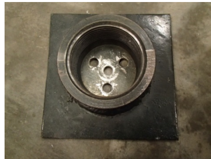
Figure B-6. Tri-stud to pipe adapter for bottom of disconnect box
