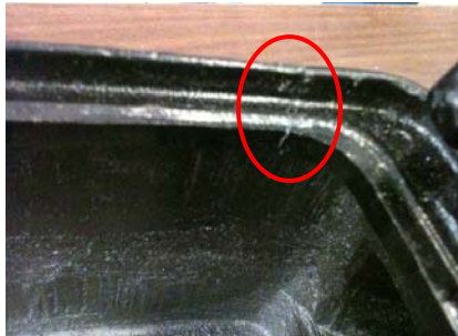
Figure A-19. DL3.2 failure mode, crack in top corner
