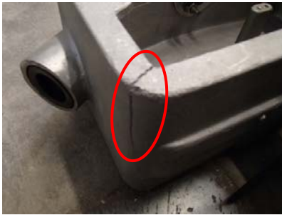
Figure A-10. DL1.1 failure mode, crack in bottom corner
