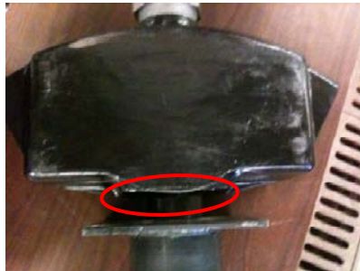
Figure A-59. DS1.2 failure mode, crack around bottom
