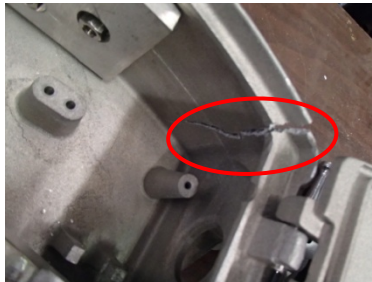
Figure A-43. RDS1.2 failure mode, crack in top corner
