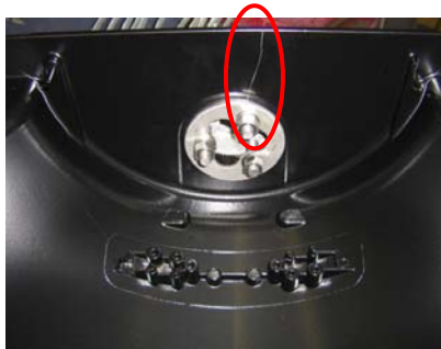
Figure A-35. SH4.2 failure mode, crack at top connection
