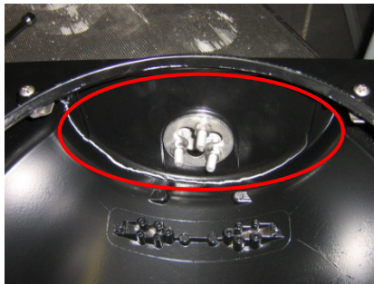
Figure A-91. SH4.2 failure mode, crack around top surface
