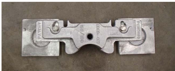
Figure B-11. Large disconnect reinforcement, bottom
