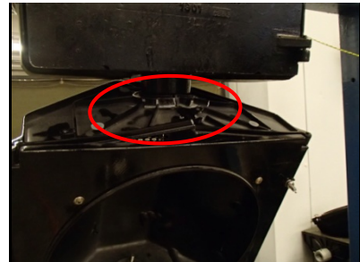
Figure A-40. C1.3 failure mode, crack at top of signal
