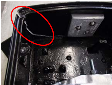
Figure A-46. RDL1.1 failure mode, crack starting in top corner
