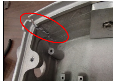
Figure A-44. RDS1.3 failure mode, crack in top corner
