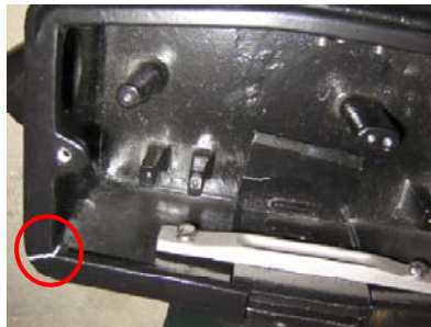
Figure A-67. DL1.2 failure mode, crack in bottom corner
