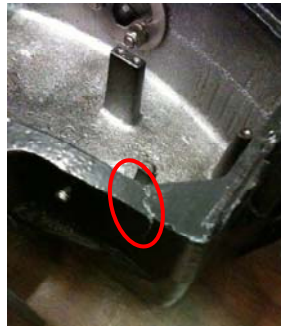
Figure A-3. DS1.2 failure mode, crack in bottom corner
