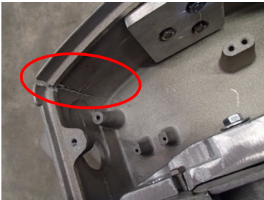
Figure A-42. RDS1.1 failure mode, crack in top corner
