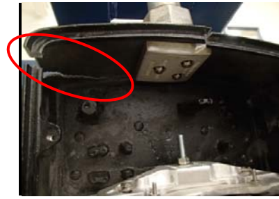
Figure A-48. RDL1.3 failure mode, crack starting in top corner
