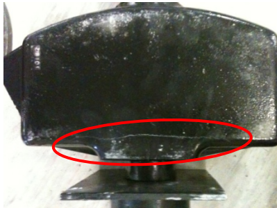
Figure A-58. DS1.1 failure mode, crack around bottom
