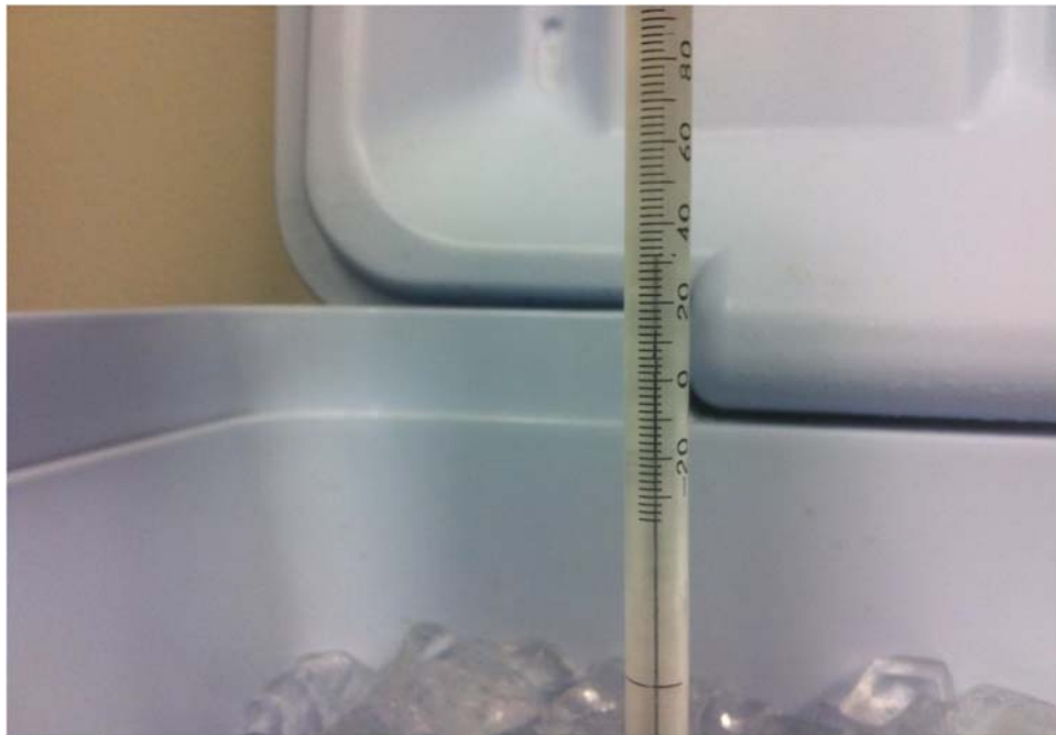
Figure 4-12. Temperature reading on a mercury thermometer in ice water.
