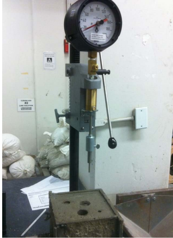
Figure 3-2. Humboldt Acme penetrometer and mortar container.
