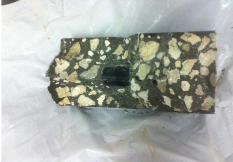
Figure 4-18. A section of broken 4"×8" specimen containing Intelli-Rock temperature sensor.
