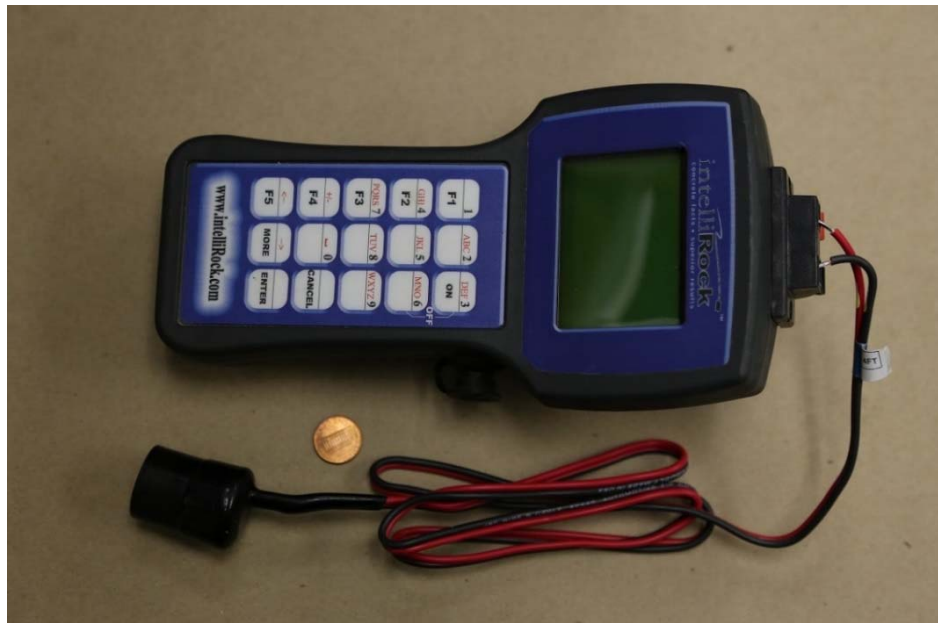
Figure 4-3. Temperature sensor and hand-held reader of the Intelli-Rock maturity system.
