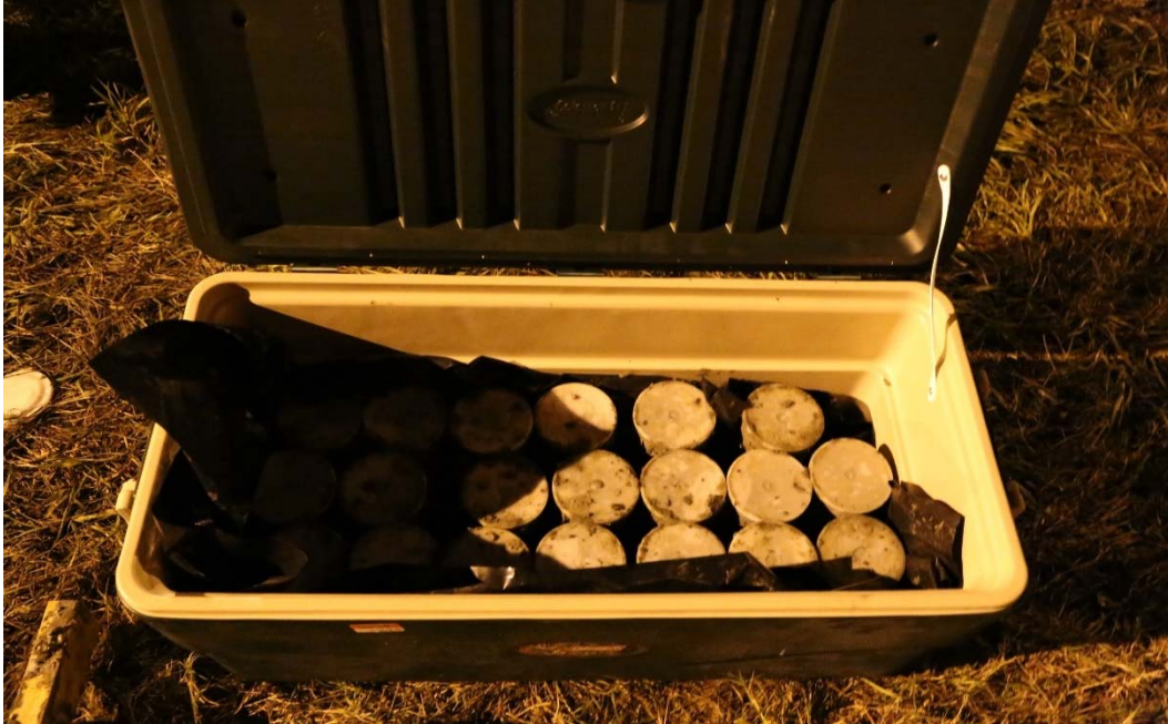
Figure 6-4. Curing of the specimens produced from the slab concrete.
