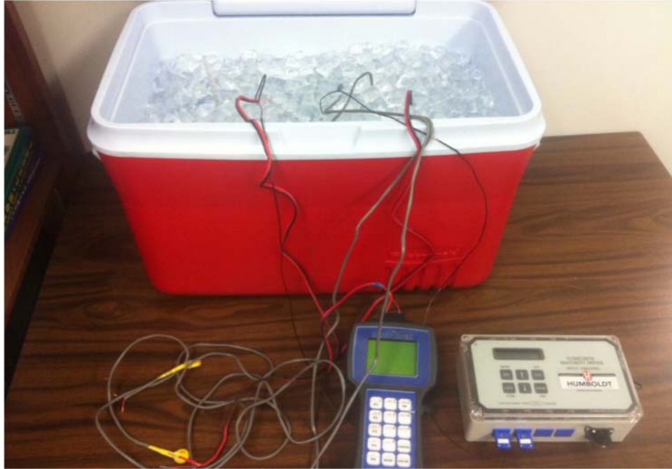
Figure 4-11. Different temperature sensors placed in ice water.
