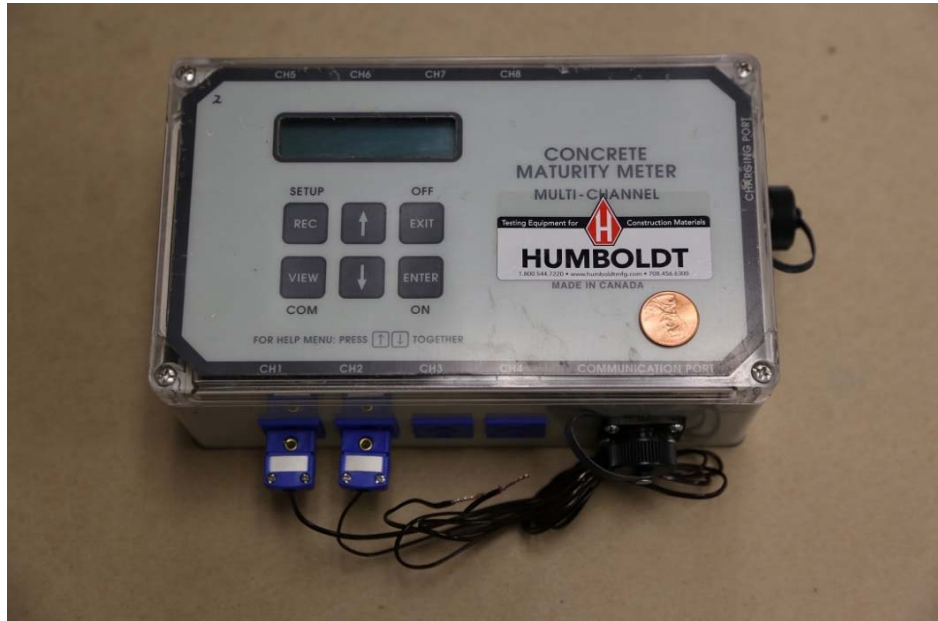
Figure 4-1. Humboldt 4101 maturity meter with thermocouple wires.
