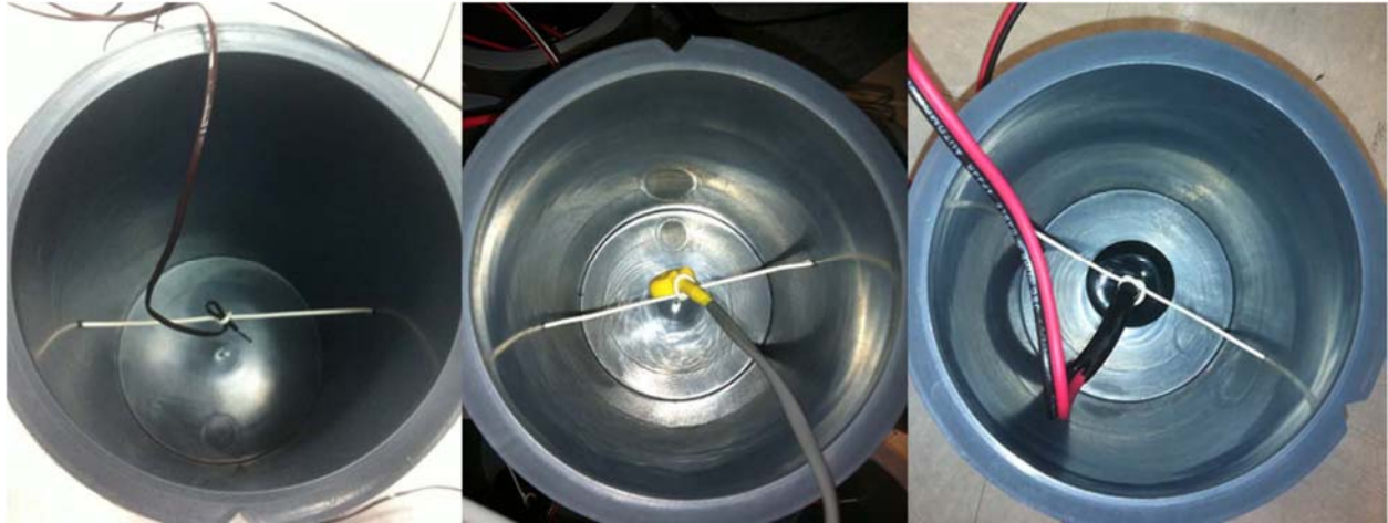
Figure 3-1. Pre-installed temperature sensors in the 4"×8" cylinder molds.
