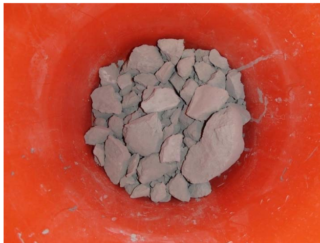
Figure 93—Pre-hydrated grout chunks removed before mixing
