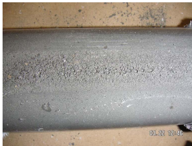
Figure 50—Porous surface observed in top half of tube containing PT1-2 at MWD
