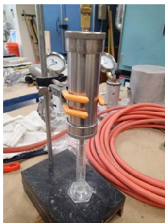
Figure 29—Pressure bleed test setup used during MITT
