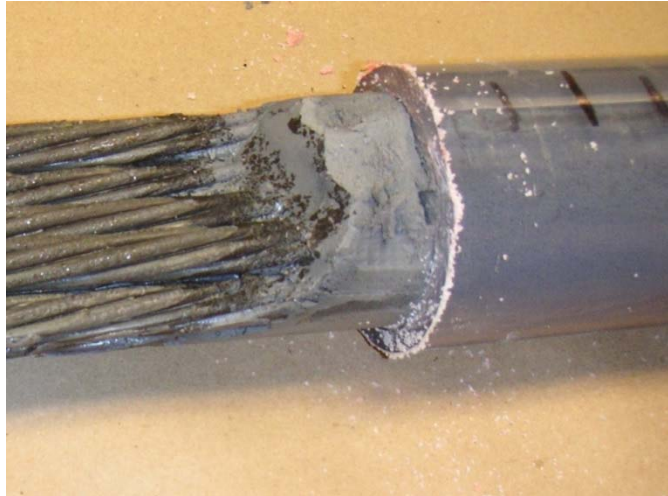
Figure 60—Soft grout found at top of tube containing PT4-1 in which the grout hose was filled with 2 gallons of water prior to injection
