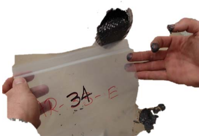
Figure 108—PT4-6 Soft Grout
