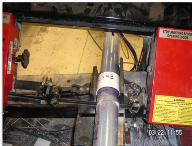
Figure 12—Saw-cut tubes for sampling
