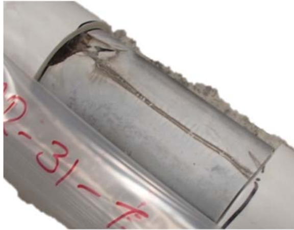
Figure 115—Segregation canal at top of cross-section
