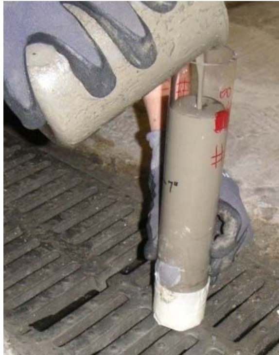
Figure 30—Pouring grout into cylinder for sedimentation test
