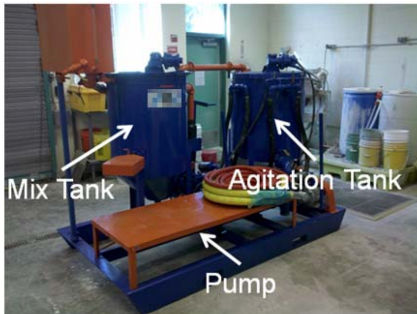
Figure 6—Colloidal grout plant with various parts labeled
