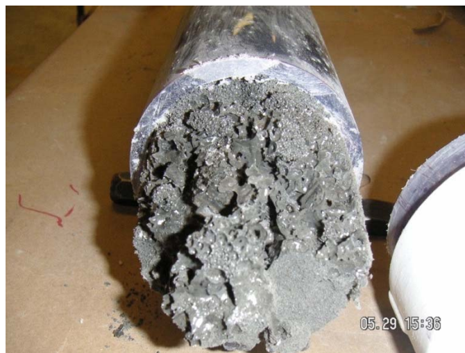
Figure 51—Porous grout observed in PT1-2 at 1.15·MWD
