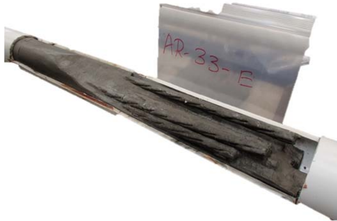
Figure 114—C675-35 large void due to bleed water
