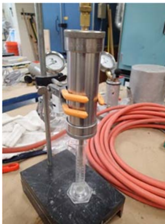
Figure 29—Pressure bleed test setup used during MITT
