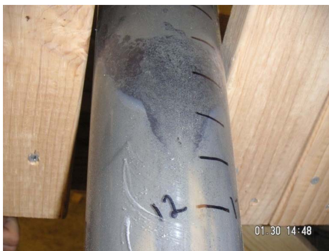
Figure 65—Grout coating interior wall of clear PVC tube
