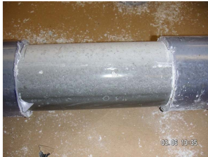
Figure 13—Tube wall removed for sampling
