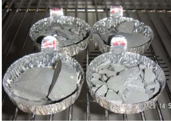
Figure 18—Grout samples drying in oven for moisture content test
