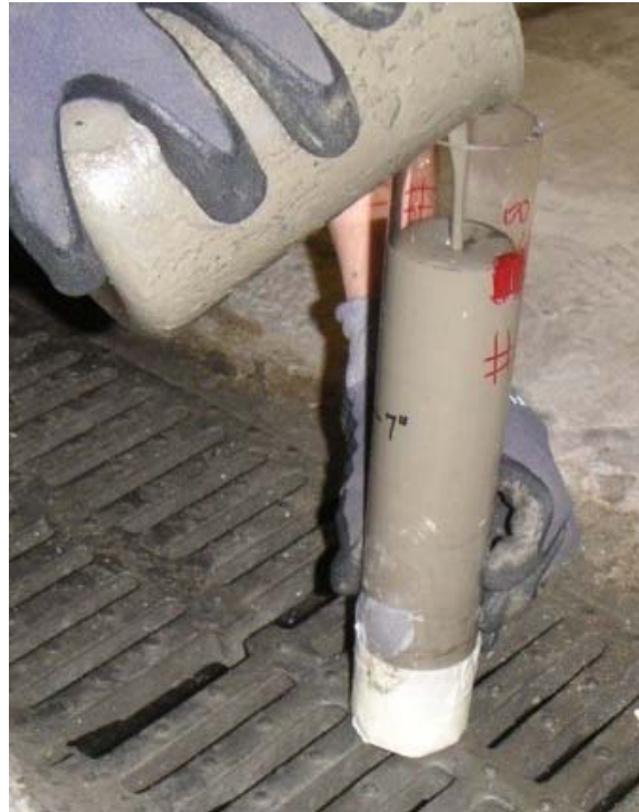
Figure 30—Pouring grout into cylinder for sedimentation test
