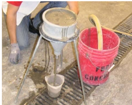
Figure 26—Flow cone used to determine fluidity of grout samples during MITT
