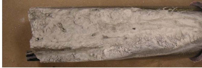
Figure 61—Top of tube injected with material C45; grout is white and hard
