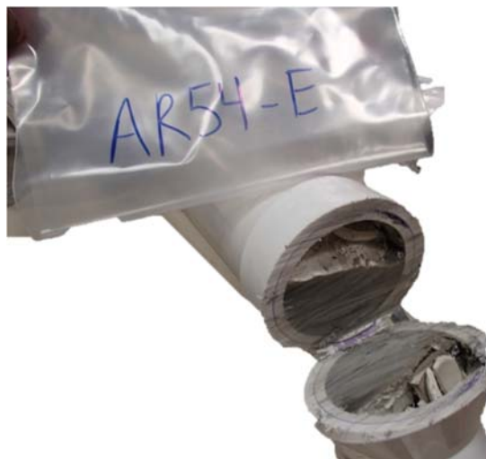
Figure 111—C35-0 soft grout
