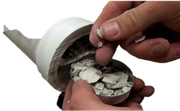
Figure 112—C35-0 soft grout
