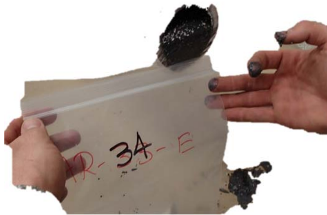
Figure 108—PT4-6 Soft Grout
