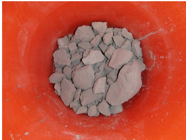
Figure 93—Pre-hydrated grout chunks removed before mixing
