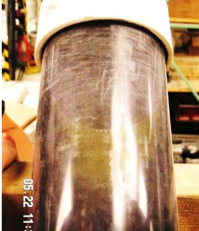
Figure 66—Bleed water visible in PT2-2 24 h after injection
