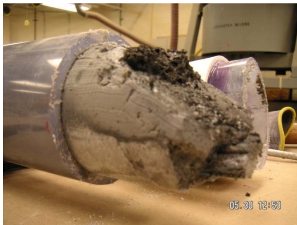
Figure 58—Soft grout and black material found in tubes injected with PT4-2 mixed at 1.15·MWD
