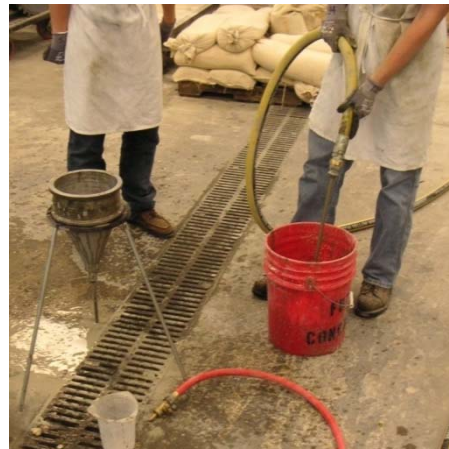
Figure 10—Discharging grout for testing prior to inclined tube injection
