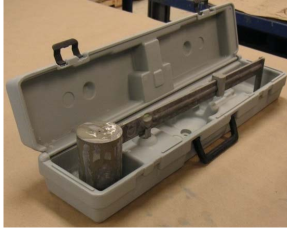
Figure 28—Mud balance used to determine wet density of grout samples during MITT
