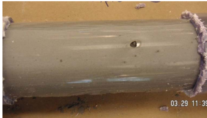
Figure 54—Smooth grout surface with air bubble observed in PT3-1 mixed at MWD
