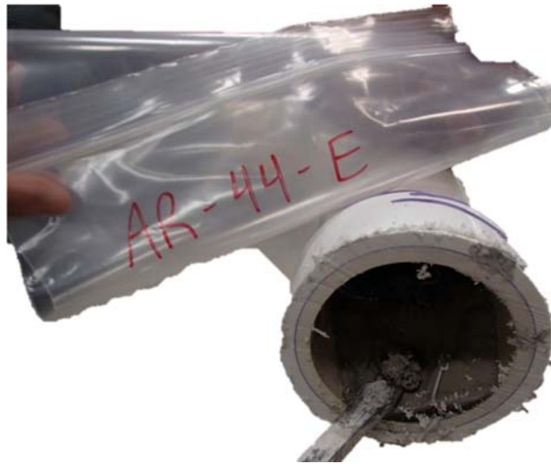
Figure 110—C675-45 soft grout
