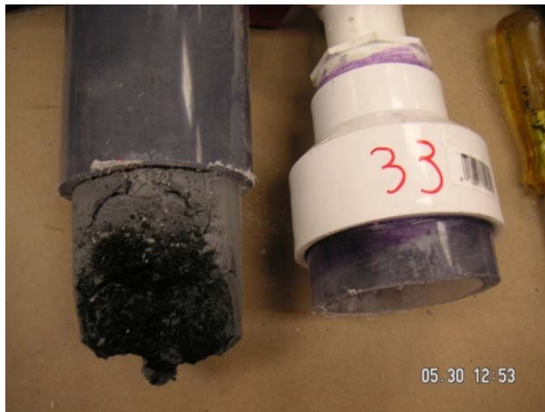
Figure 57—Black material and soft grout found in tubes injected with PT4-2 mixed at 1.15·MWD
