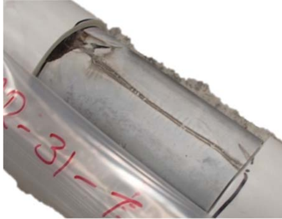
Figure 115—Segregation canal at top of cross-section
