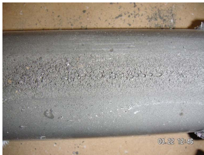
Figure 50—Porous surface observed in top half of tube containing PT1-2 at MWD
