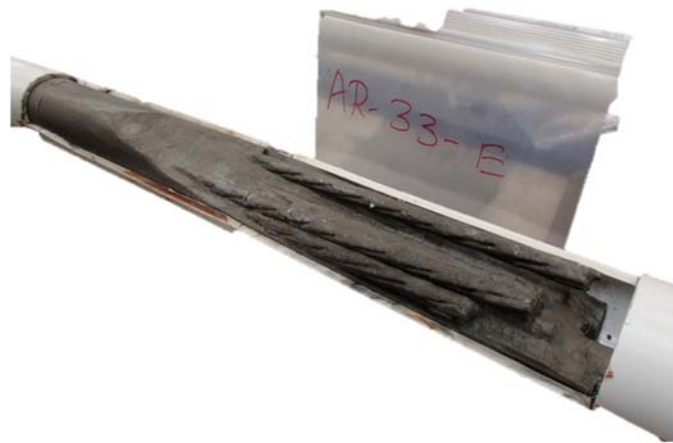
Figure 114—C675-35 large void due to bleed water
