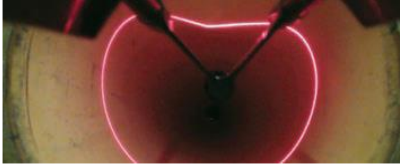
Figure 2-4: Laser Ring Profiler (from Maverick Inspection Ltd. )
