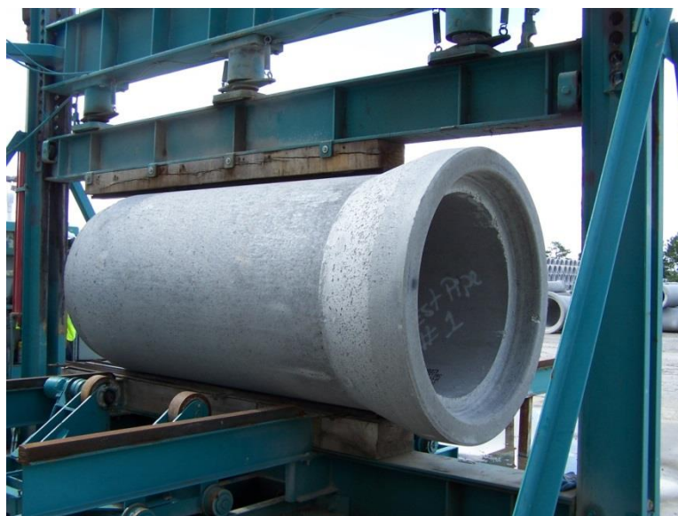
Figure 3-10: Introduction of Cracks on RCP by Means of Three-Edge Bearing Test Device
