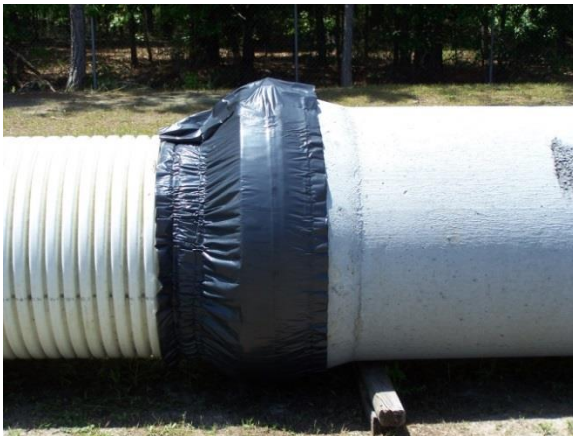
Figure 3-15: Dissimilar Pipe Coupler at PVC-to-RCP Junction
