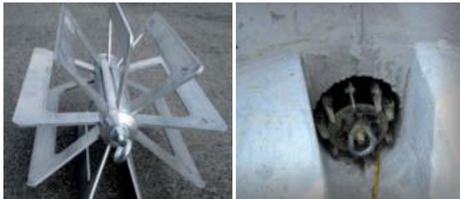
Figure 2-2: Image of Pipe Mandrel by Itself and within a Pipeline (from the Ontario Concrete Pipe Association)
