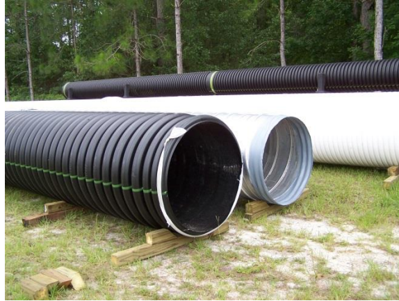
Figure 3-9: Positioned PVC, CMP, and HDPE Pipes
