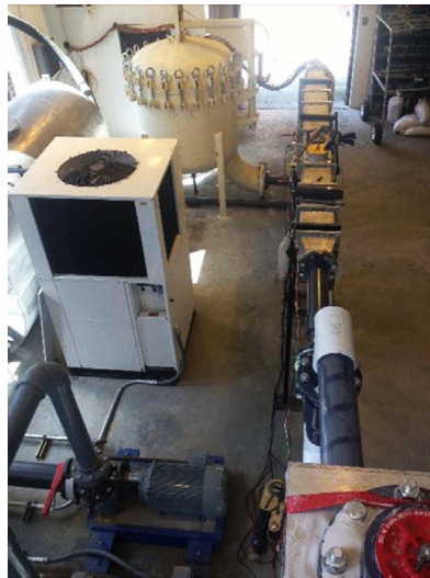
A bird's eye view of SERF. The test chamber is on the right; support devices, such as pumps and filters, are on the left.
