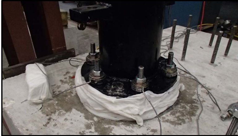
Figure 4-3. Grout pad and 2 in. cubes after wet-wrapping
