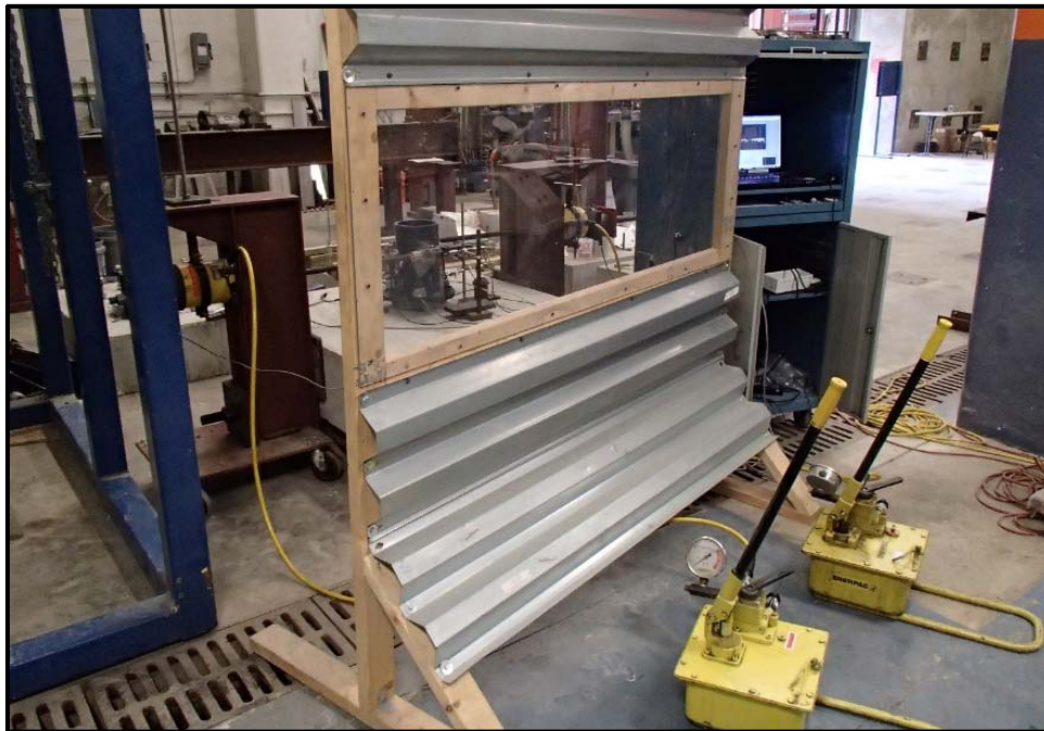
Figure 4-17. Hydraulic hand pumps used for torsion loading
