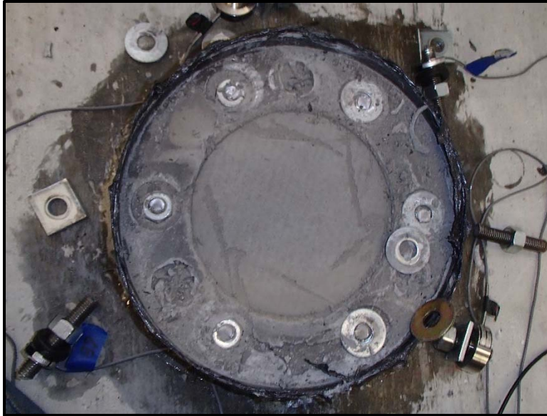
Figure 5-6. Post-test grout surface for T7 (FRP-retrofitted 4d_b base plate stand-off)
