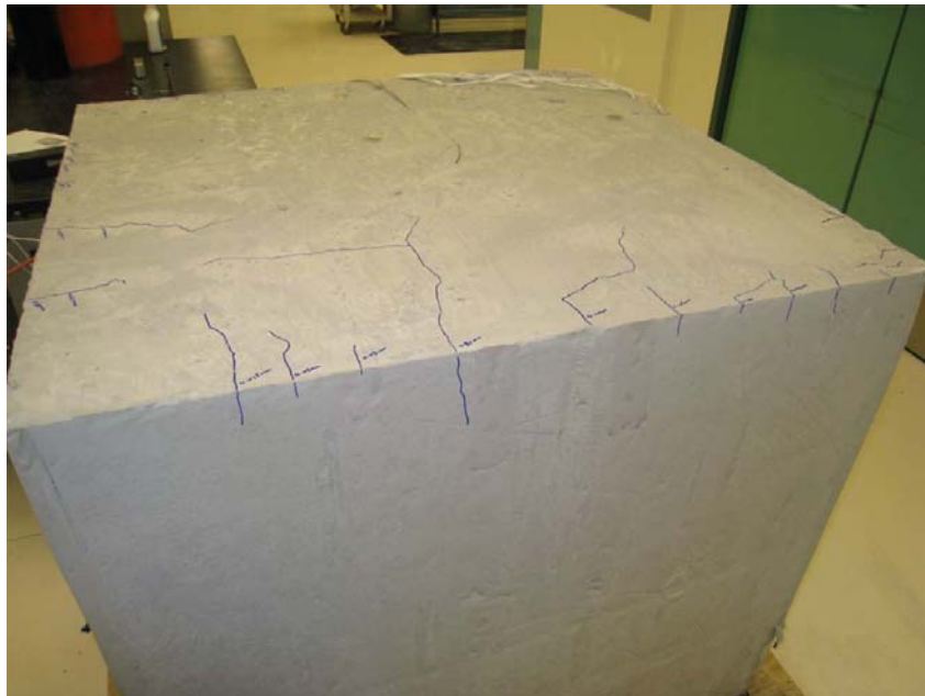
Figure 2-7. Typical location and distribution of cracking found in experimental blocks (Lawrence et al., 2012).
