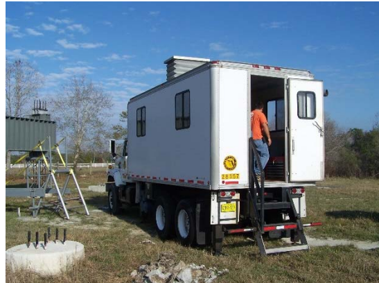
Figure 3-19: PMT test in center of field shaft footprint
