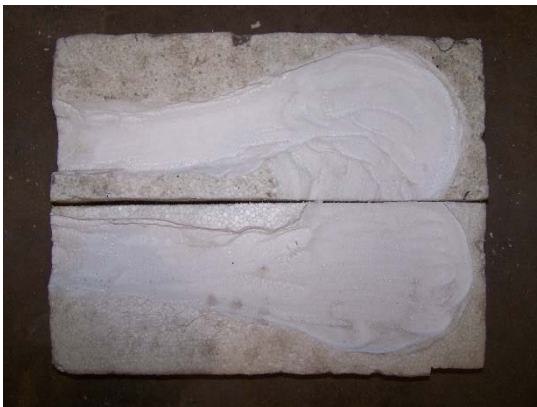
Figure 3-36: Styrofoam used to prevent flexible hose from becoming embedded in shaft
