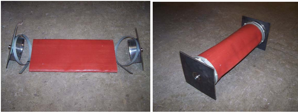
Figure 3-9: Apparatus used to test the failure mode for joint fabrication method
