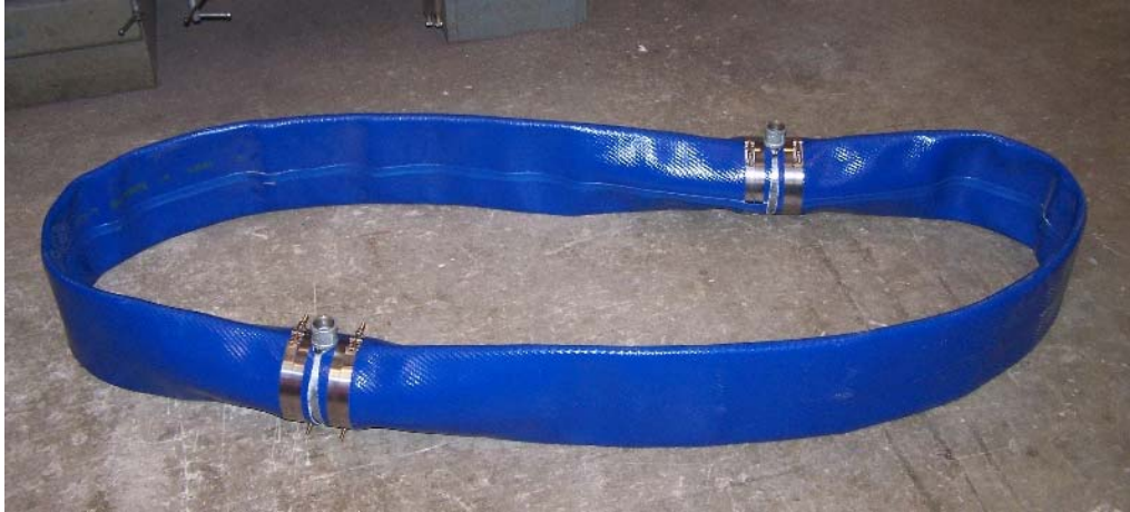
Figure 3-33: Bottom membrane seal fabricated for field shaft
