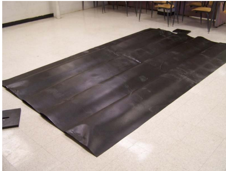
Figure 2-47: RPP used to fabricate side membrane used with long shaft
