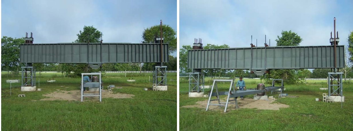
Figure 3-66: Wooden frame used to support digital dial gauges
