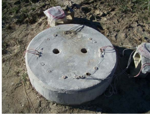
Figure 3-69: Drilled holes for additional instrumentation (strain and accelerometer)
