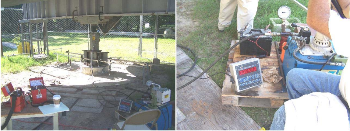
Figure 2-69: Applied load during static load test
