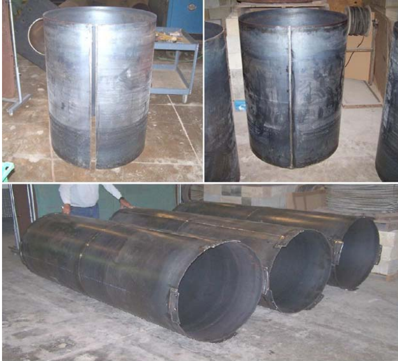
Figure 2-38: Temporary casing used with long shaft
