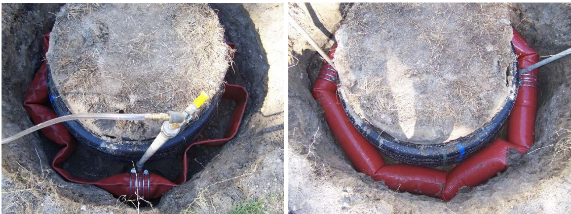
Figure 3-5: Test the improved membrane seal design with two hose clamps
