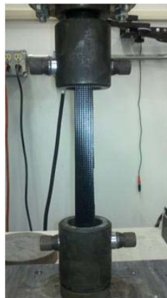
Figure 2-4: Tension test on reinforced low density polypropylene using UTM
