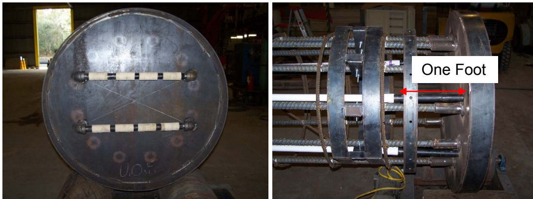
Figure 3-31: Tip grout delivery system
