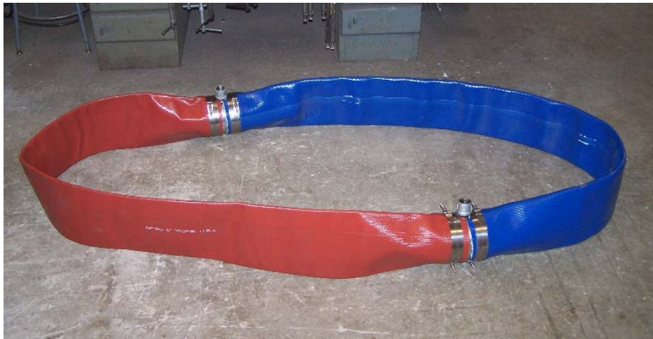
Figure 3-34: Top membrane seal fabricated for field shaft
