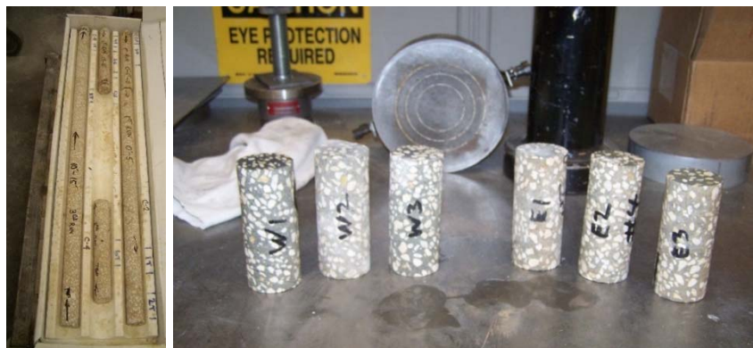
Figure 3-70: Recovered cores from field shaft
