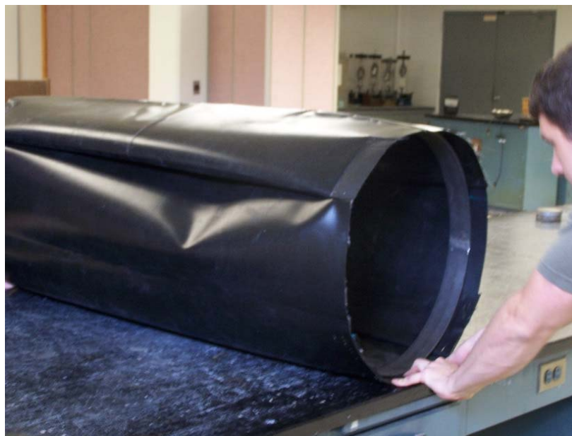
Figure 2-9: Vertical pleats used to reduce circumference of side membrane
