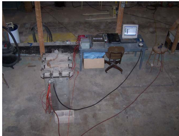
Figure 3-23: Pressure vessel test with RST push-in pressure cells
