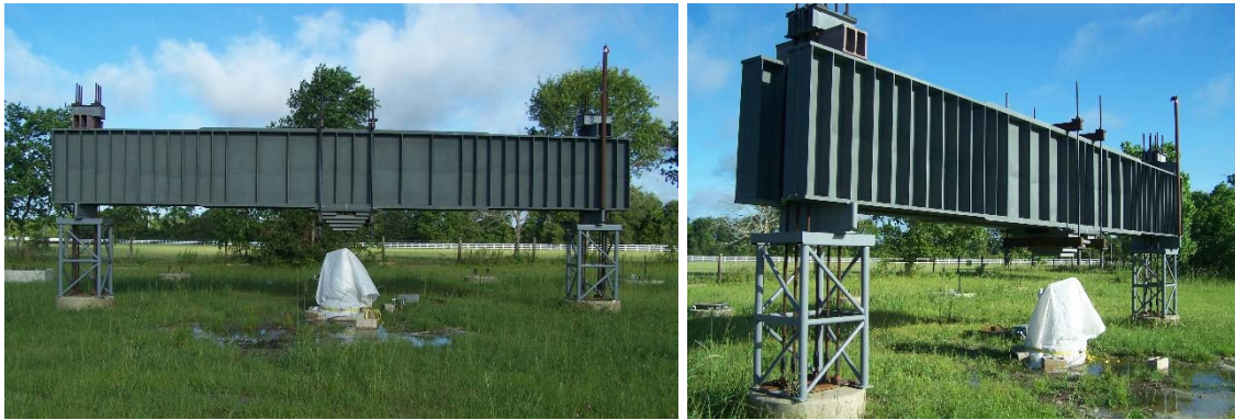
Figure 3-65: Field reaction system used for static load test
