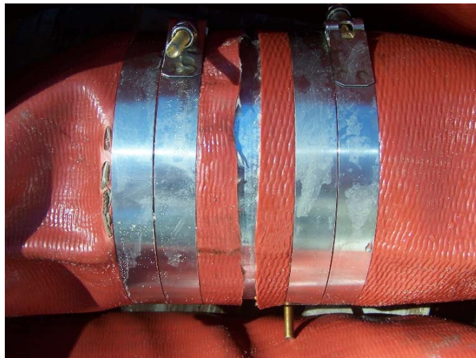
Figure 3-13: Rupture failure observed with final membrane seal joint fabrication method
