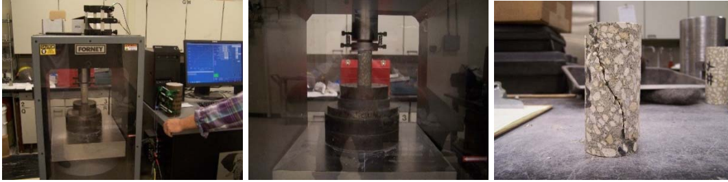
Figure 3-71: Unconfined compression test on recovered core sample
