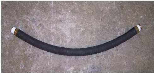
Figure 3-35: Flexible hydraulic hose used to allow membrane seal to expand outwards unrestricted
