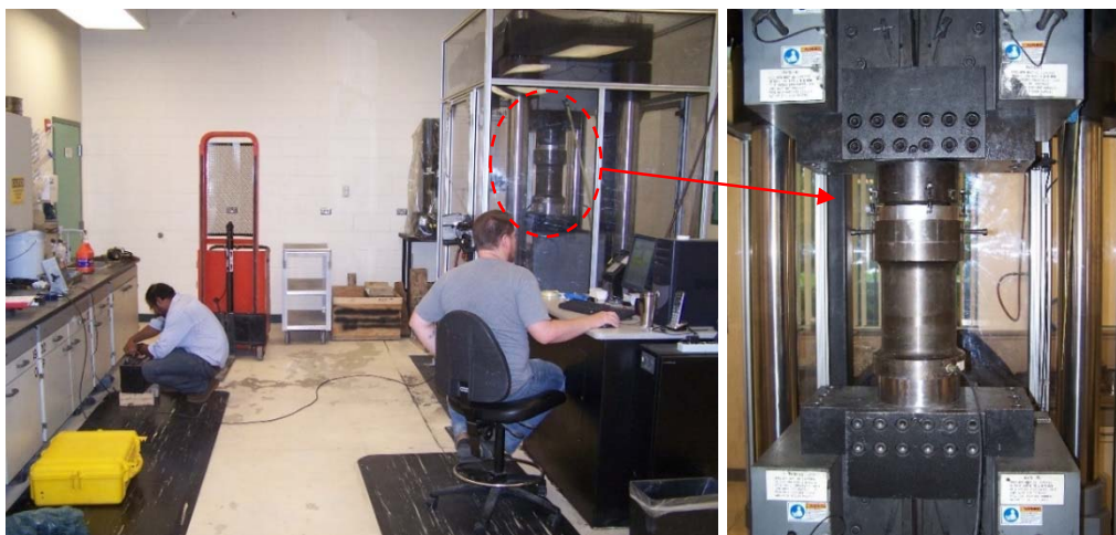
Figure 3-61: Checking load cell and readout boxes at SMO
