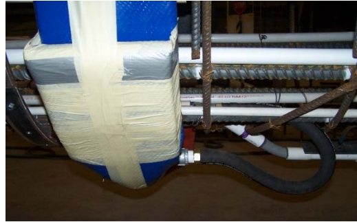
Figure 3-35: Flexible hydraulic hose used to allow membrane seal to expand outwards unrestricted
