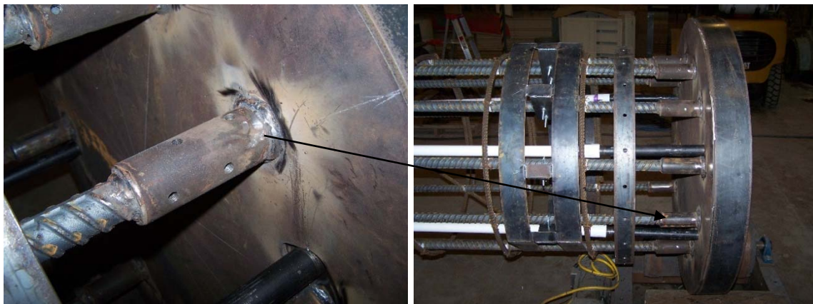
Figure 3-29: Base plate connection to rebar cage
