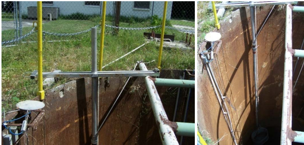
Figure 3-73: Suspend pipe from edge of test chamber with catch container below bottom of pipe
