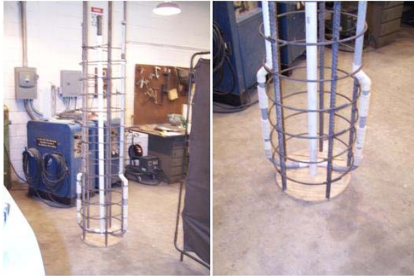
Figure 2-13: Grout delivery pipe for tip grouting
