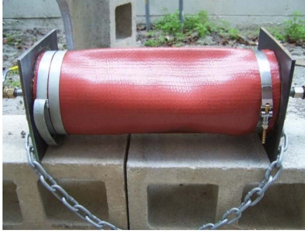
Figure 3-10: Test setup with steel banding (left) and t-bolt hose clamp (right)
