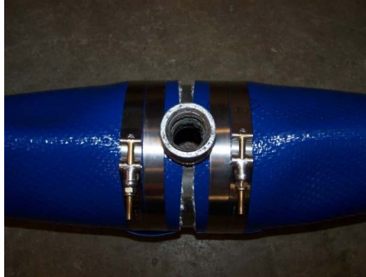
Figure 3-14: Blue layflat hose (310 psi rated working pressure)
