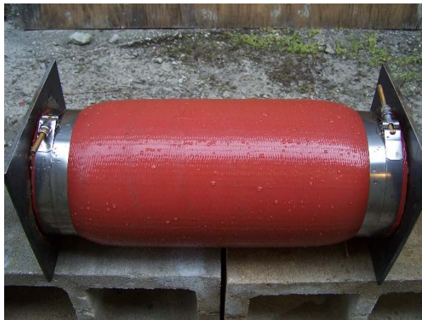
Figure 3-11: Final membrane seal joint fabrication method
