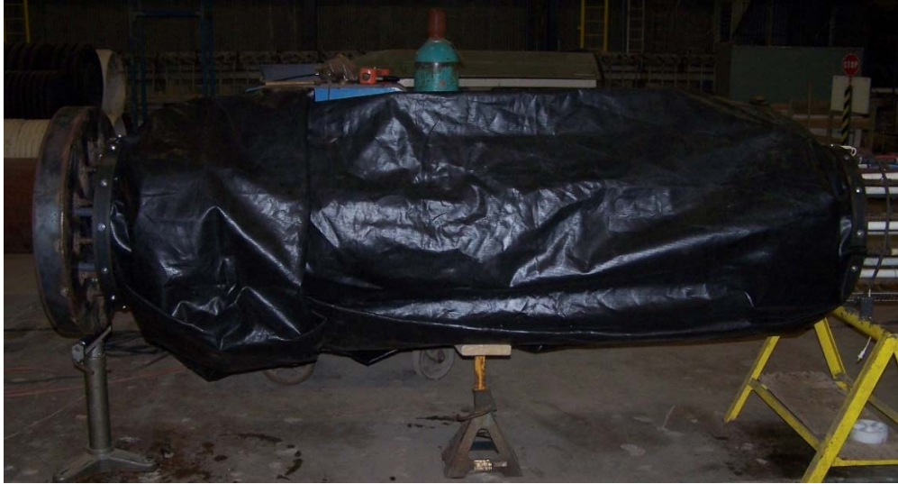
Figure 2-49: Pleated side membrane secured to cage by steel rings
