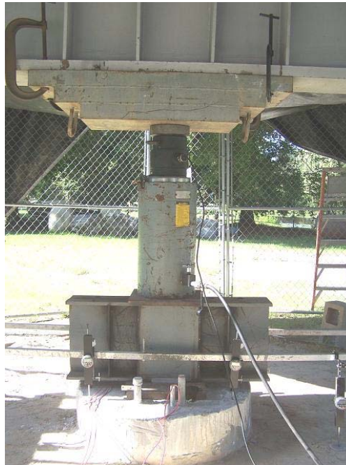
Figure 2-67: Load application setup for static test
