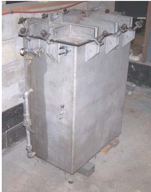
Figure 2-32: Pressure vessel used to test earth pressure cells
