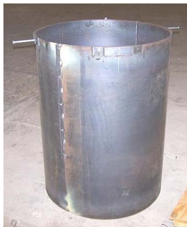
Figure 2-39: Removable shaft form used with long shaft
