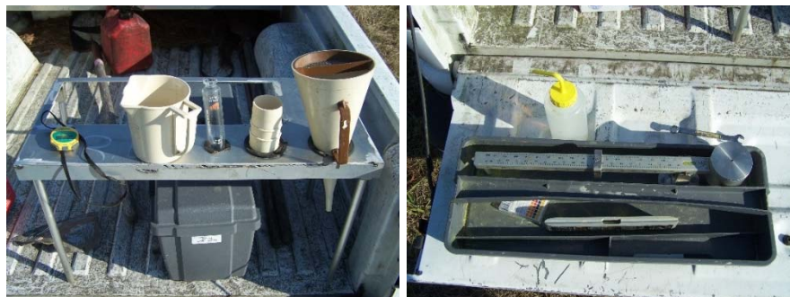
Figure 3-49: Equipment used to check slurry quality
