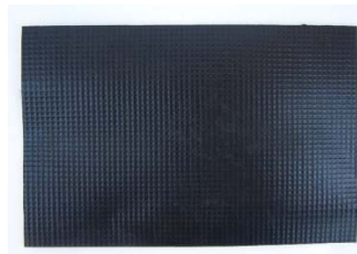
Figure 2-3: Piece of reinforced low density polypropylene (45 mil thick)
