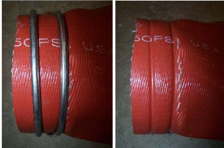
Figure 3-7: Permanent distortion of the hose due to the high torque wire clamps
