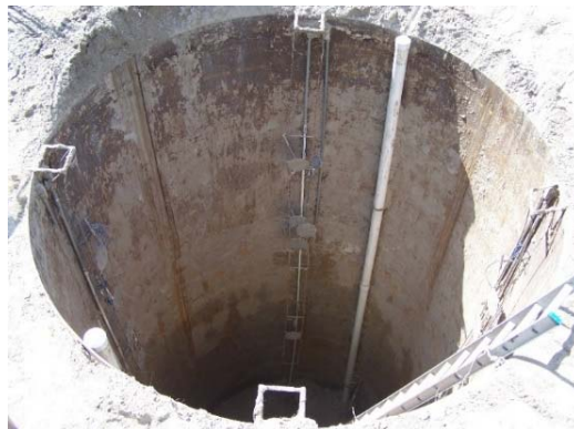
Figure 2-30: Recovered pressure cell secured to steel racks along sides of test chamber
