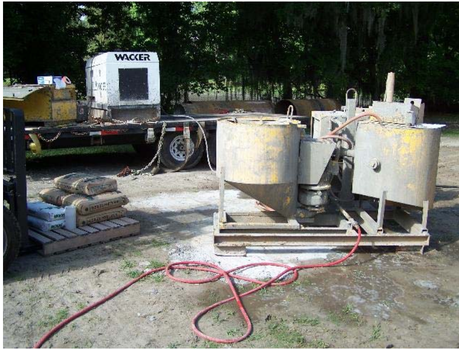
Figure 2-61: Conventional high pressure grout mixer and pump
