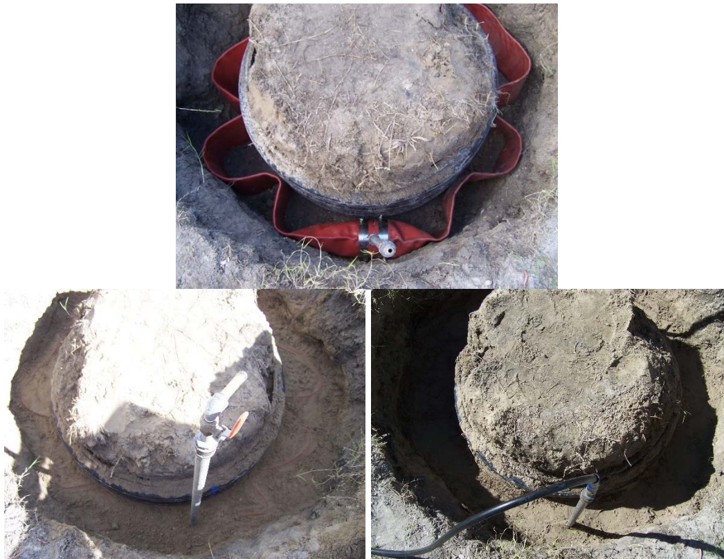
Figure 3-12: Test final membrane seal joint fabrication method with inner and outer boundary conditions
