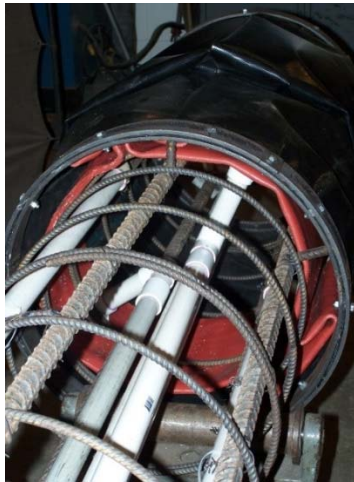
Figure 2-11: Steel rings used to secure the side membrane to rebar cage
