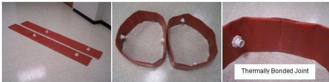
Figure 2-6: Membrane seal fabrication for short shaft
