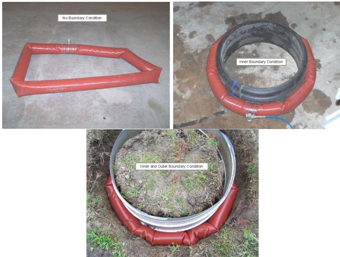
Figure 2-25: Test the effects of boundary conditions on membrane seal performance
