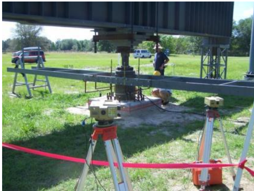
Figure 6-12. Test setup for top-down testing of jet-grouted pile 2
