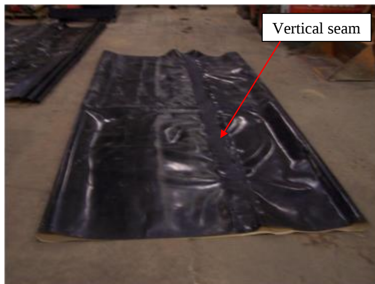
Figure 5-12. Membrane seamed for side grout zone
