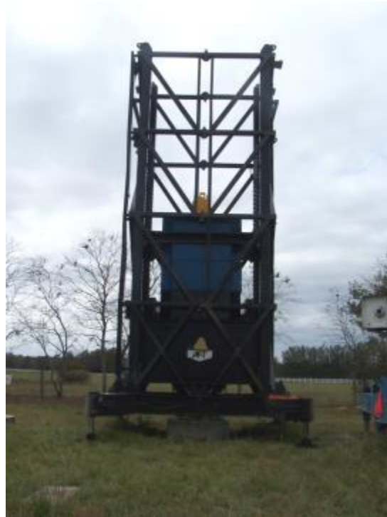
Figure 6-16. 500-ton Statnamic testing on jet-grouted pile 1
