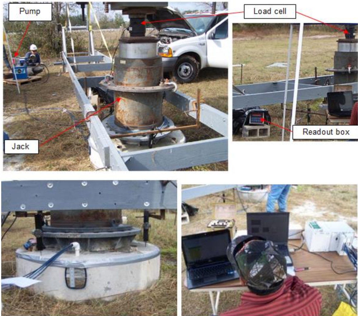
Figure 6-3. Hydraulic jack, load cell, digital dial gauges, mirrored scale with wire line reference, and data acquisition using National Instruments device
