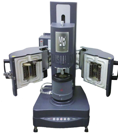
The dynamic shear rheometer, a tabletop device, can simplify testing the temperature performance of grout.
